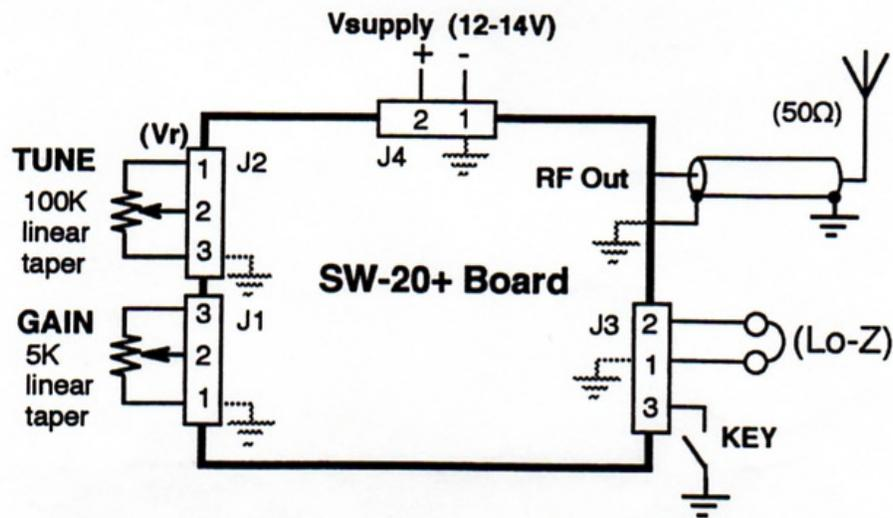
Wire the connectors and controls to the SW-20+ as shown pictorially below. Note that the keying return line lacks its own distinct board connection. This return line is shared with the headphones' return.
