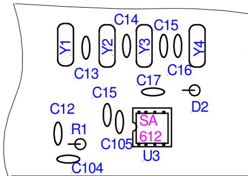
*(When these components have been installed, the product detector/BFO and crystal filter sections of the transceiver are complete.)*
