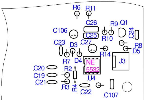
*(When these components have been installed, the audio amplifier section of the transceiver is complete.)*
