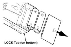
Move the LOCK tab in the opposite direction of the arrow marked on the bottom of the transceiver.
