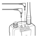
**Caution:** Use only microphone and speaker accessories that do not share a common ground for the speaker and the microphone. Doing otherwise might damage the transceiver.
