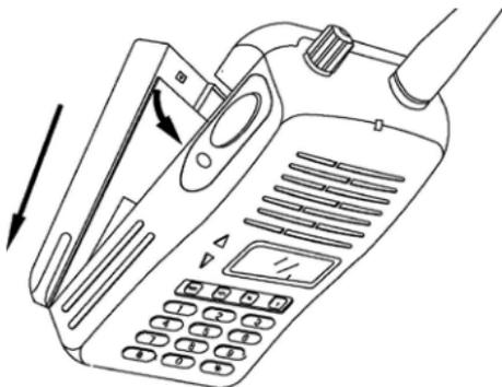
2. Push the battery pack along transceiver rear until the released button full lock the battery.
