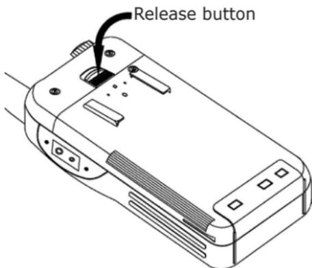
3. If want to remove the battery pack, just need to impulse the release button and then push the battery in opposite direction as install above.
