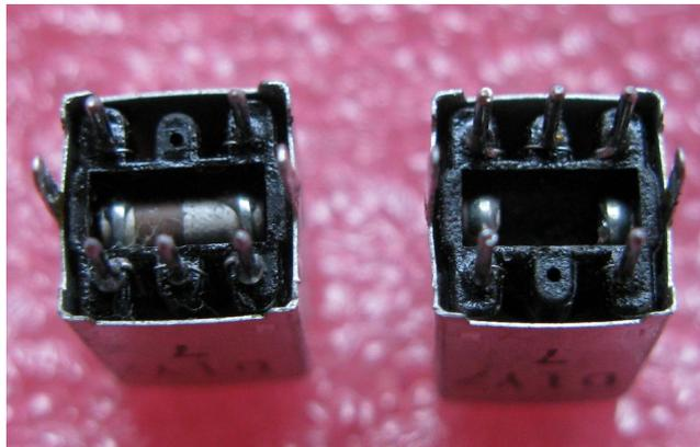
[ ] Solder the VXO crystal(s). You don't need to place insulator under the crystal or ground the crystal case. You may need to solder 1x or 2x crystals, depending on the frequency range you have selected for your kit. If you just need to solder 1x crystal, either slot will be okay
