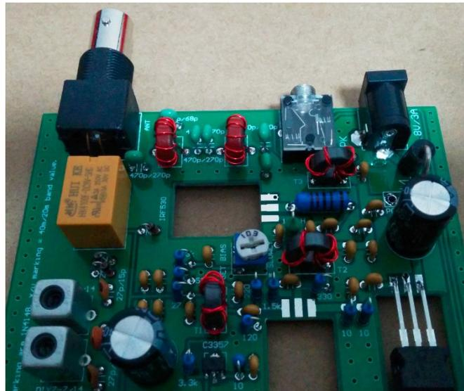
[ ] Desolder the 7808 voltage regulator, and clean the solder from the pads and pins
