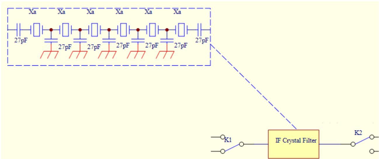
[ ] Pick 6x IF crystals and solder. You don't need to place insulators under the crystals or ground the crystal cases
