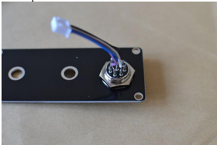
[ ] Make sure both potentiometers have a nut on first. Plug in the microphone cable into the SIP5 socket on board, install the front panel using two black chassis screws, then put a washer and another nut on each potentiometers, and finally install the knobs.
