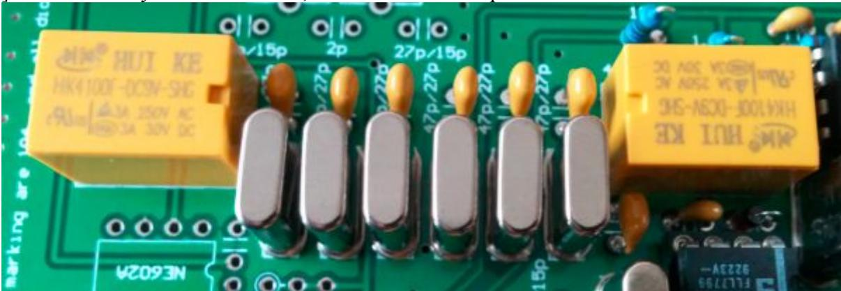
[ ] Plug in a 12~13.8 V power supply and connect an external speaker to the speaker connector. Touch pin 5 of the uninstalled NE602A using tweezers to note a little noise from the speaker. If it is not normal, please check your soldering. If it is okay, disconnect the power supply and the external speaker to proceed to the next step.
