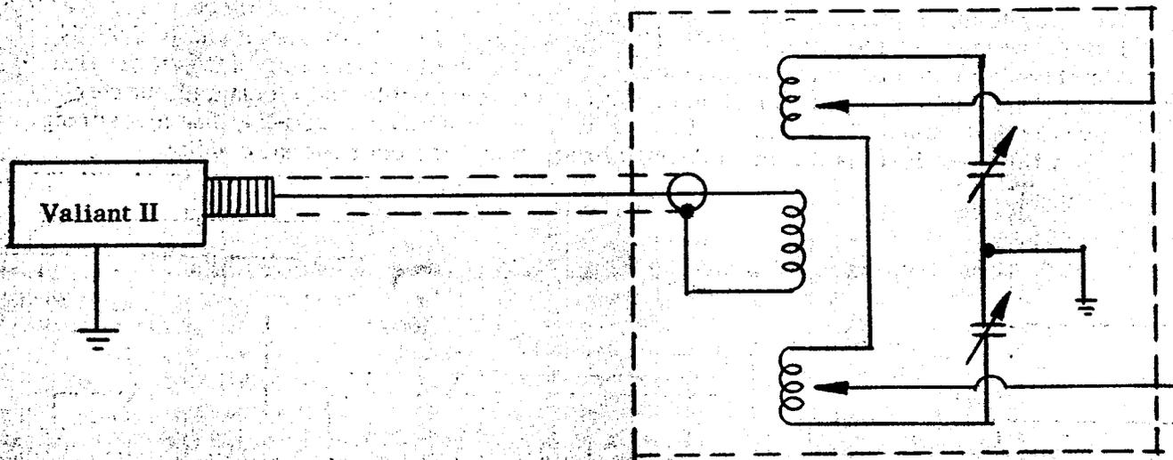
Feedpoint impedance of the coupler is adjusted by means of the inductor taps. Tap adjustment is unnecessary with the JOHNSON Matchbox. Final amplifier loading is adjusted with the transmitter output coupling controls.
