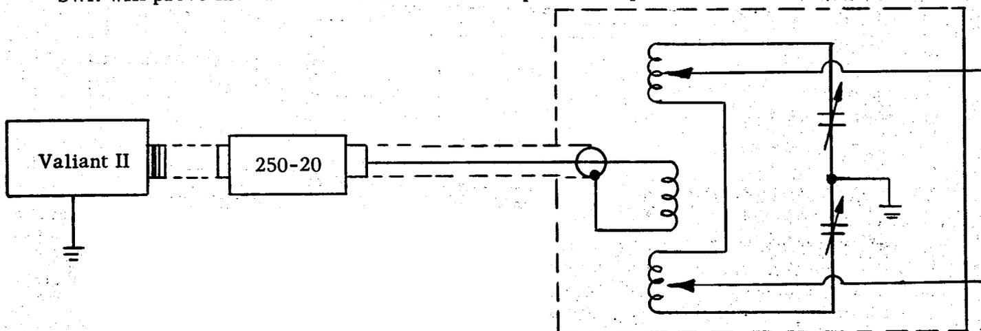
An end fed half-wave antenna may present loading problems, both from the standpoint that its impedance is higher than can be matched by the pi-network amplifier of the Valiant II, or that the low output coupling capacitance used reduces inherent harmonic attenuation below tolerable values. Therefore, the use of a half wave antenna may create TVI problems while other antennas prove perfectly satisfactory. In these cases it is recommended that the JOHNSON Matchbox be used.
