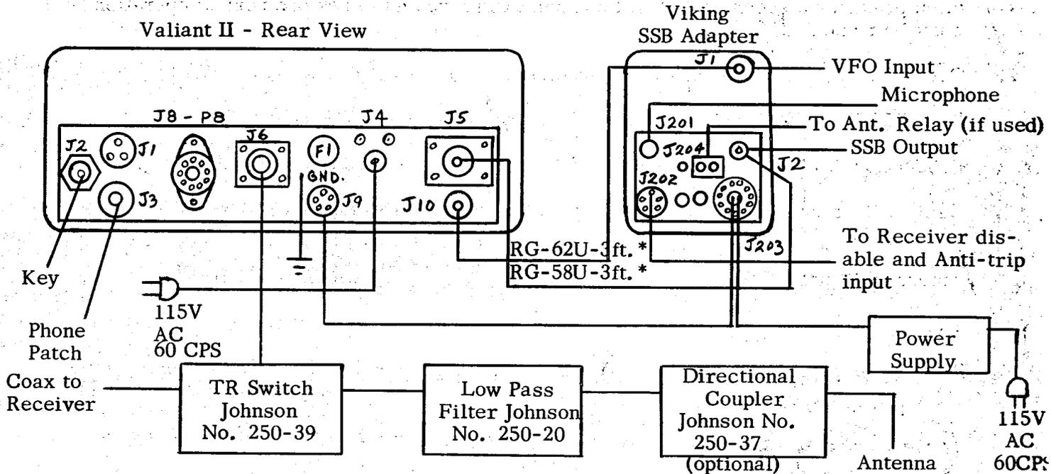
\* The RG-62/U and RG-58/U cables must be made exactly 3 feet long
