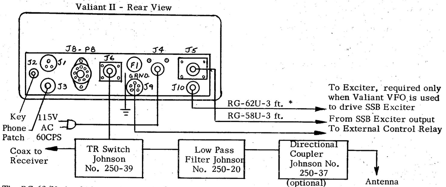
\* The RG 62/U should be made exactly 3 feet long.
