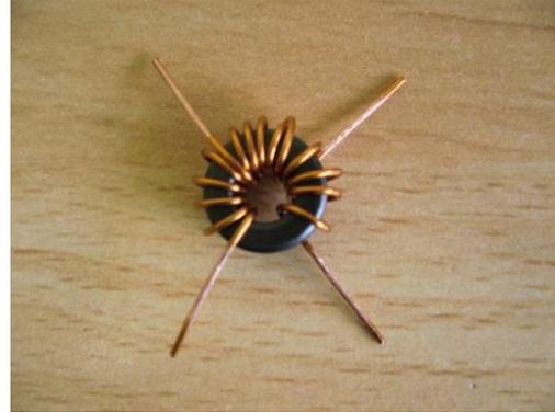
Important: Wind the toroid exactly as shown in the pictures. You must respect both the number of turns as the winding direction.
