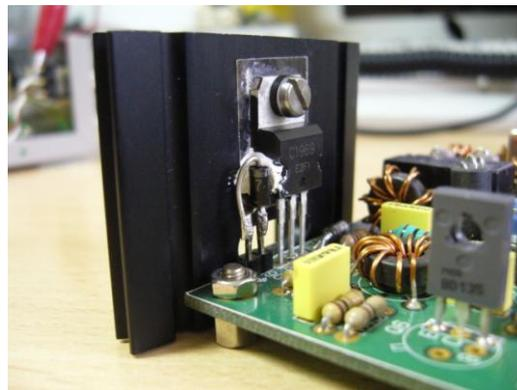
**DO NOT operate the transceiver without a heatsink for Q7.**
