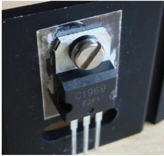
The Q7 encapsulation must be electrically isolated from the radiator. Use a lock washer and mica sheet that came with the transistor. Once clamped transistor, check with a multimeter that the transistor housing does not contact the screw or the radiator. Use the insulators supplied with a screw and a nut M3. It is advisable to apply some thermal paste.
