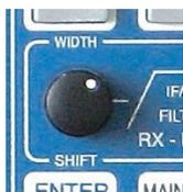
Adjustment of EQ bands is also possible with WIDTH/SHIFT control (as long as the EQUALIZER menu will be displayed):
