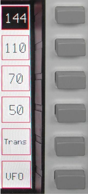
Select 2 m band; the softkey will be displayed inverse (as shown here); pressing this key again will toggle between the last two frequencies used within this band.
