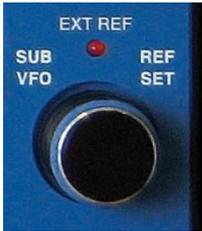
The correction value for the reference oscillator is adjustable by turning the SUB VFO / REF SET knob. Tuning range  $\pm 10$  Hz Ref ( $\pm 1$  ppm).
