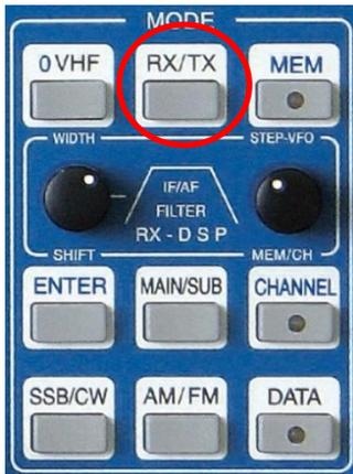
Pushing the button **RX/TX** located in the cluster MODE will call up two types of menus which gives access to various basic settings for RX and TX.
