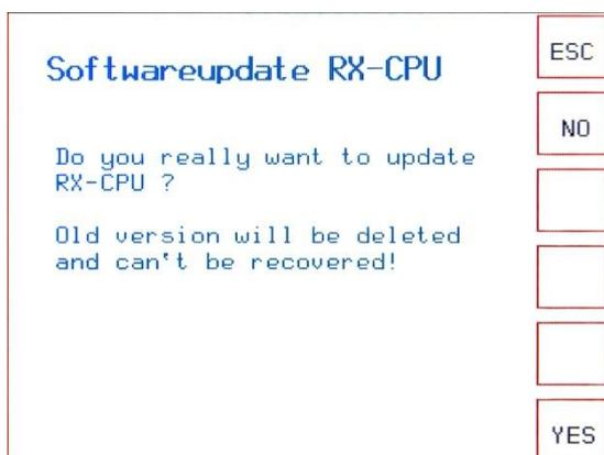
The **ESC** and **NO** softkeys lead back to the screen and the softkey menu *Softwareversion* (Fig. A2- 16/17).
