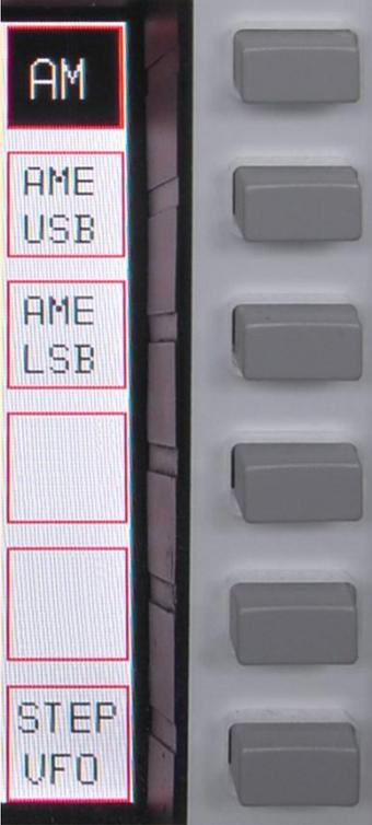
Amplitude Modulation (carrier and two sidebands); the softkey will be displayed inverse (as shown here); the display will show **AM** (left of frequency).
