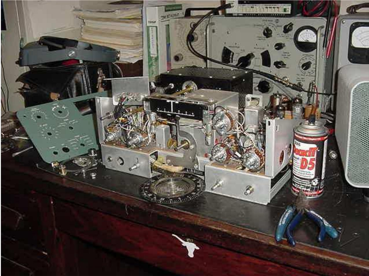
The "SB-101/SB-102 specific" information for this site is still being developed. They are pretty rugged units and I've found some weak tubes, a few tubes with grid emissions, the usual requirement for alignment per the manual, and slipping tuning dials needing adjustment. And yes, they are a poor (but smart) man's Collins.
