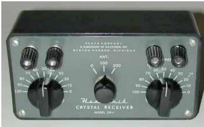
Over a period of about five years (1957 - 1962) Heathkit also sold a crystal radio set kit, the CR-1. This radio, like most, tuned the AM broadcast band from 540 KHz to 1600 KHz (kc
