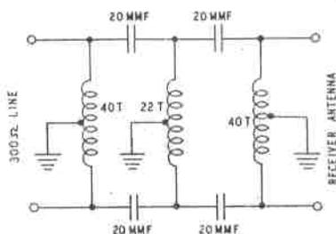
Coils are wound of No. 30 wire on a 1/8" diameter form.
