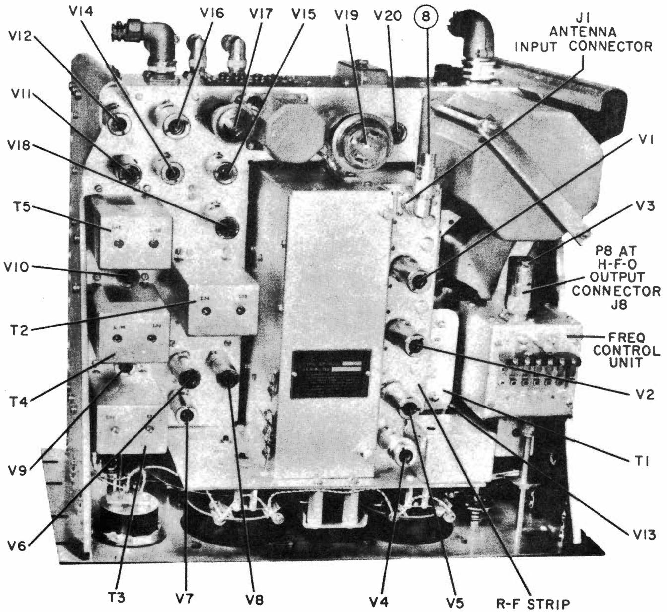
Figure 7. Radio Receiver, Top View of Chassis
