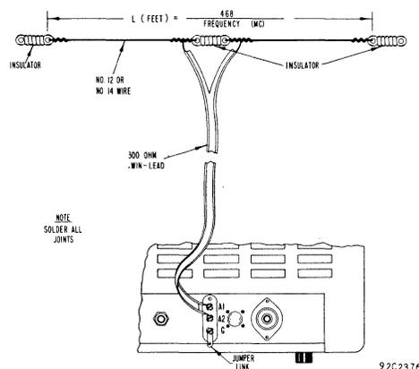
Fig. 3. Doublet Antenna Using Twin-Lead Transmission Line
