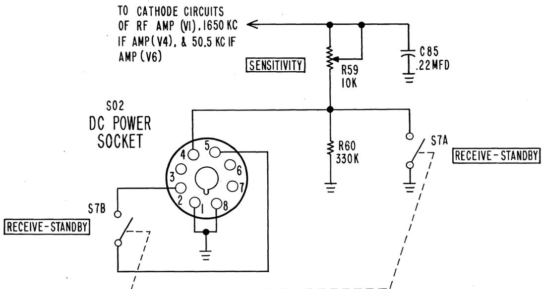
Fig. 6. Schematic Diagram of Sensitivity and Receive-Standby Circuits
