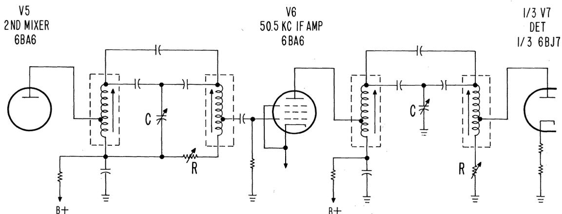
Fig. 13. Equivalent Schematic Diagram of 50.5 KC IF System
