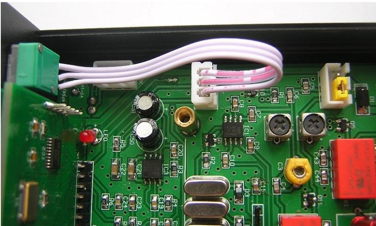
Solder a 3-pin header wire to one of the gain control potentiometers, following the above orientation to plug in the AF socket, and mount the potentiometer to the front panel (trim the positioning protruding part on the potentiometer before mounting).
