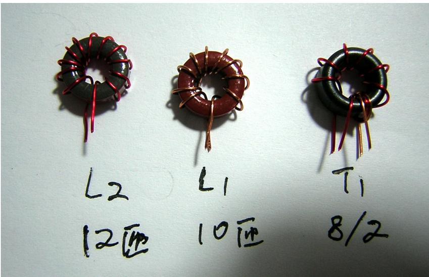
Wind the toroids as the above. L1 is 10 turns wound on the red toroid, and L2 is 12 turns wound on the red toroid, while T1 is a transformer wound on the black toroid, with 8 turns of primary winding, and 2 turns of secondary winding. Tin the wire ends before they are soldered to the PCB.
