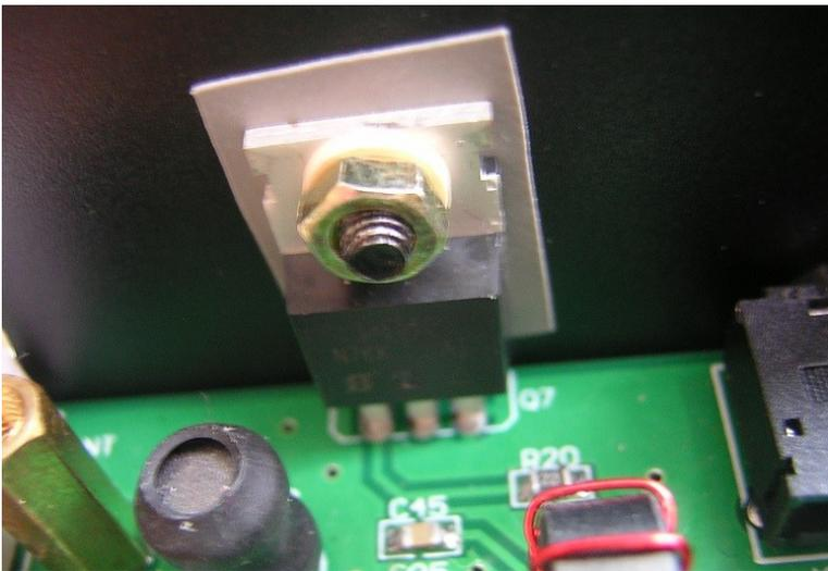
Put in a thermal pad between Q7 and the panel, plug in the screw and put on the thermal washer and tighten with nut. Now solder Q7 pins to PCB.
