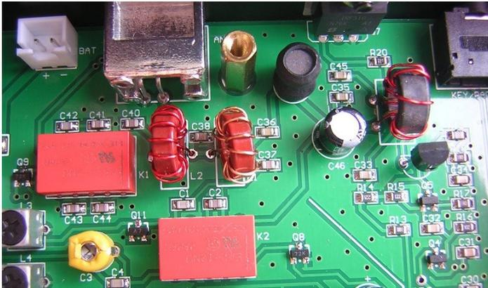
The 8 turns primary winding of T1 are installed near Q6, while the 2 turns secondary winding of T1 are installed near Q7.
