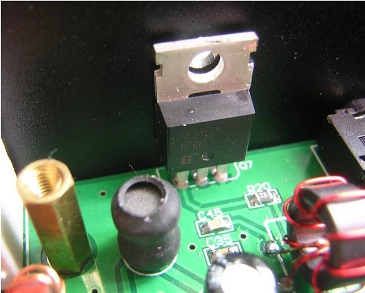
Plug in the final transistor Q7 to the PCB, but don't solder yet. Install the rear panel, and align the hole on the Q7 with the mounting hole on the panel.
