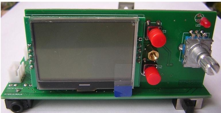
Plug in the display board to the main board. Leave no spacing between two boards and make them vertical. Check and solder.
