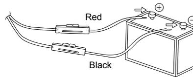
6. Connect the DC power cable to the transceiver's power supply connector.
