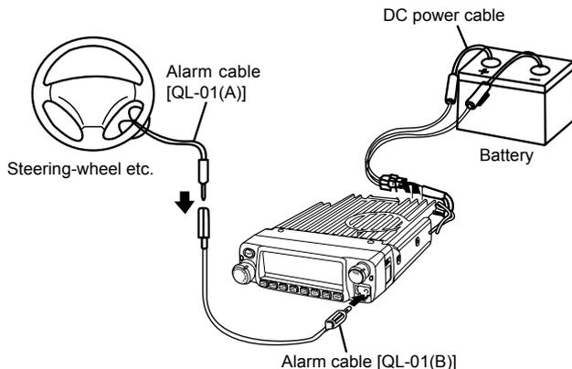
Connect DC power cable with car battery.
