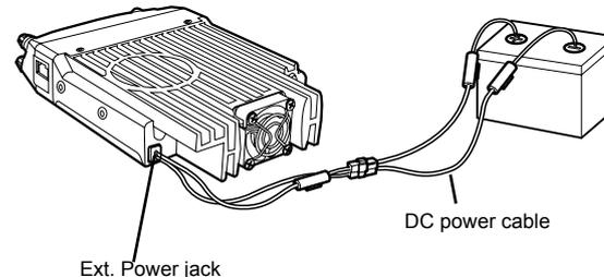
optional QCC-01 (For Cigar-Plug connection) cable. Connect one of the cables between the ACC terminal or a Cigar-Plug that operates with the vehicle ignition or ACC switch on the vehicle and EXT POWER jack on the rear side of the unit.
