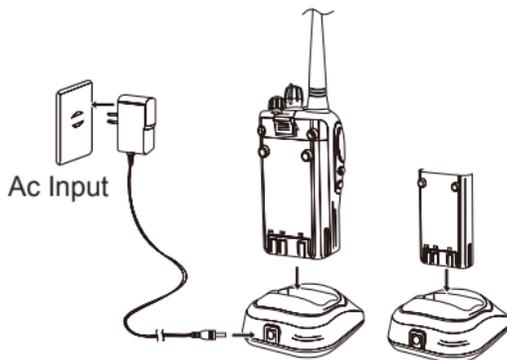
**NOTE:** when charging a power-on transceiver equipped with battery, the indicating lamp will not turn into green to show the fully charged status. Only when the transceiver is switched off, can the lamp indicate normally. The transceiver consumes energy when it is power-on, and the charger can not detect the voltage when the battery has been fully charged. So the charger will charge battery in constant voltage and fail to indicate correctly whether the battery has been charged fully.
