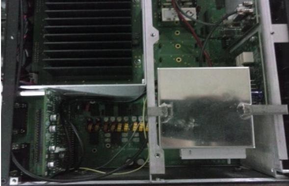
Mount the lateral panel with the 7 screws and beware with all cables from KXV3A.
