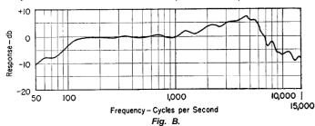
Response-Frequency Characteristic Model 55s Microphone. 27A62. 5-51.
