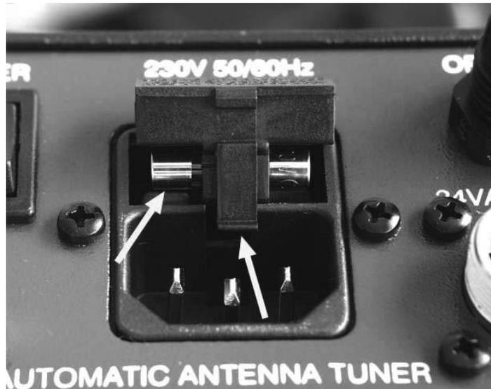
Fig. 5-1 Pulling out the AC line fuse.
