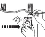
**9** Continue holding button in and scan beyond marked spot until the center green and 3 pairs of red LEDs go out.
