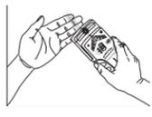
**15** The AC LED should light with an electrical cord an inch or two away.
