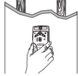
Position the TriScanner Pro SL flat against the wall. Select mode. Press and hold On/Off button.
