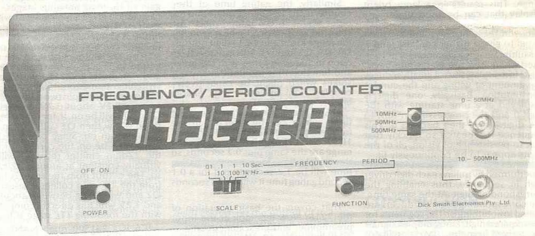
Essentially, you have two options when building this new DFM — you can either build the full 500MHz version or save money by building a 50MHz version. All you have to do is leave out the two pre-scaler ICs (IC4 and IC5) associated with the 500MHz range. More about this later on.
