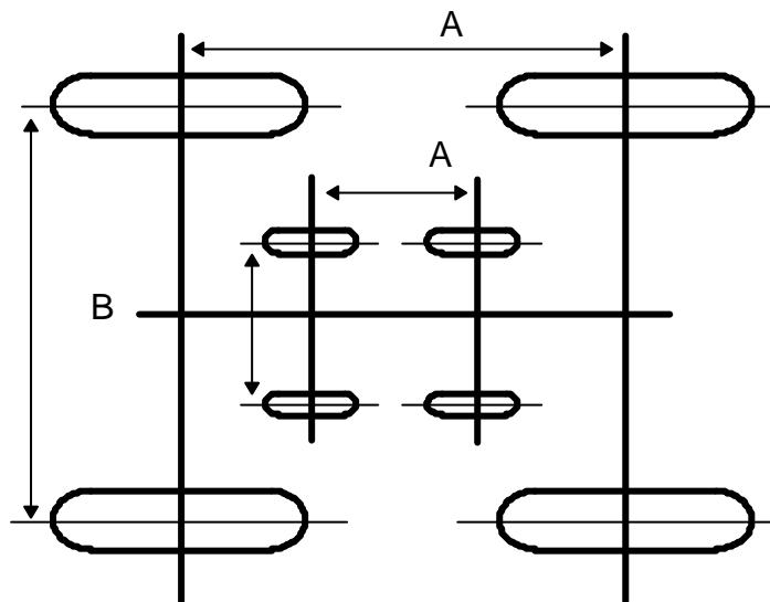
The antenna gain can be raised when stacking some antennas of same type vertically, horizontal or both. In theory you get an additional 3dB more gain by doubling the number of antennas at optimum stacking distance. Unluckily there are sidelobes when stacking, therefore a compromise between minimum sidelobes and maximum gain is to be found. See the table below for the different types of stacking.
