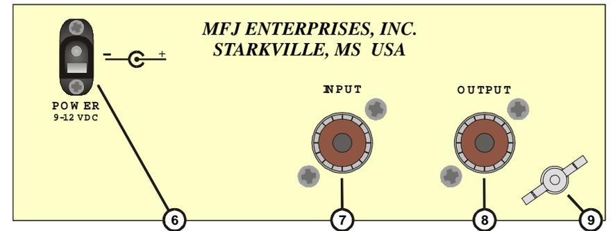
6. POWER: .....3.5mm barrel connector for power to MFJ-1020C 9-12 VDC with center positive. Inserting the plug into the rear jack automatically disconnects the internal battery. MFJ offers an optional 12 VDC adapter (AC-12).
