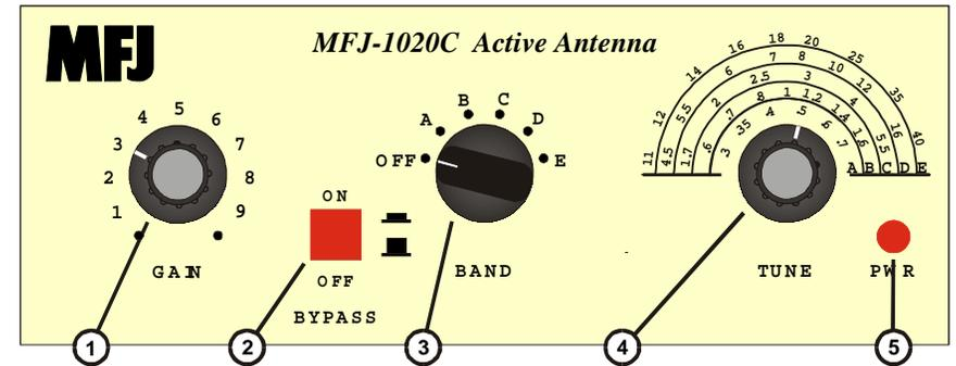
1. GAIN CONTROL:.....Adjust the gain of the MFJ-1020C from -10 dB to +10 dB.
