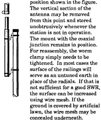
The disconnection point also allows for speedy changing of the upper section on terrace or balcony locations. In this way, a GPA antenna may be used for operation on 20/15/10m or 40/20/15/10m or 80/20/15/10m. If there is not enough space vertically, the antenna may be tilted outwards. If you wish to order your GPA with a disconnection point, please write "Tr" after the article number on your order. The disconnection point is separately priced.
