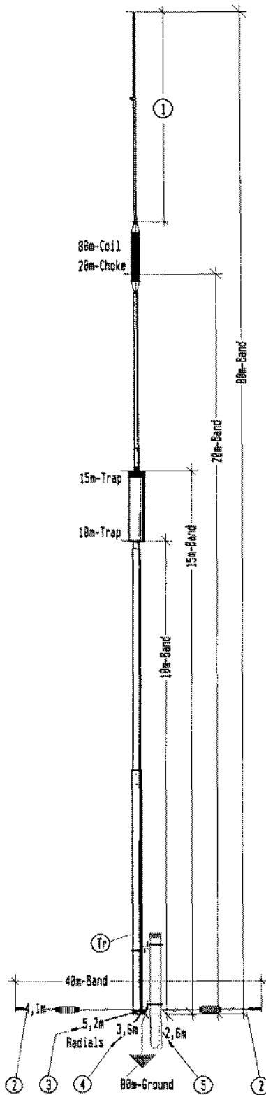
(1) The 80m resonance may be influenced at this point by lengthening or shortening. For the upper portion of the band, the tuning tube has to be pushed in and for the lower portion it must be extended. A change in length of 5cm results in a 50 kHz difference in resonance. A length of 135 cm, from the top to the edge of the coil plug, is taken as the approximate value for the middle of the band 3.65 MHz.
