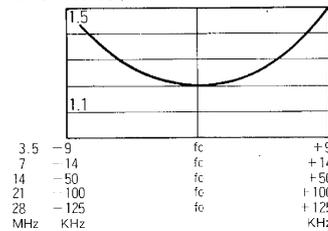
center frequency. Therefore, radial element has to be shortened for 105 mm to achieve 3535 center frequency.
