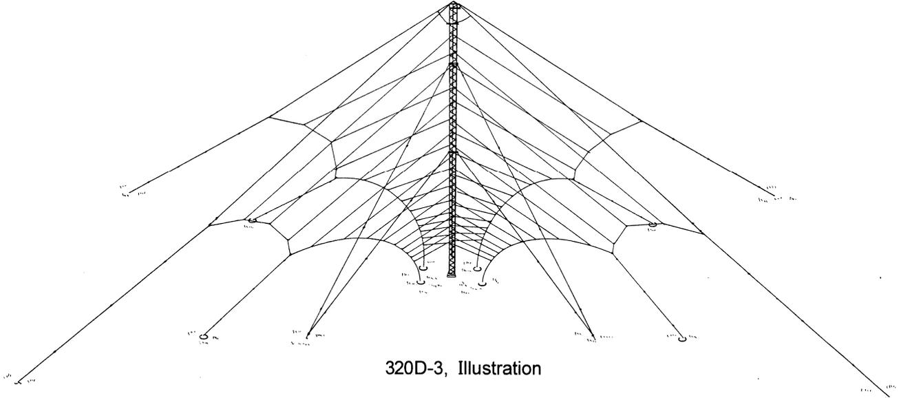
The CD model 320D log-periodic antenna is designed specifically to support reliable short-medium range communications. Vertically polarized antennas can not always provide reliable short range coverage because of limitations in the radiation pattern or excessive attenuation of the ground wave.
