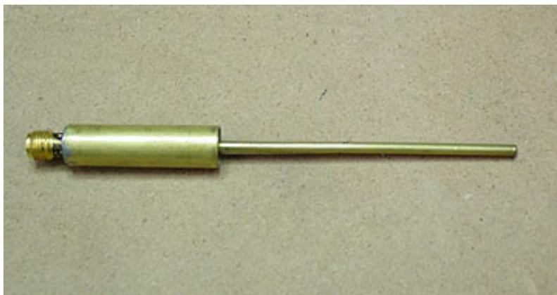
Figure 7: Completed decoupler assembly.
