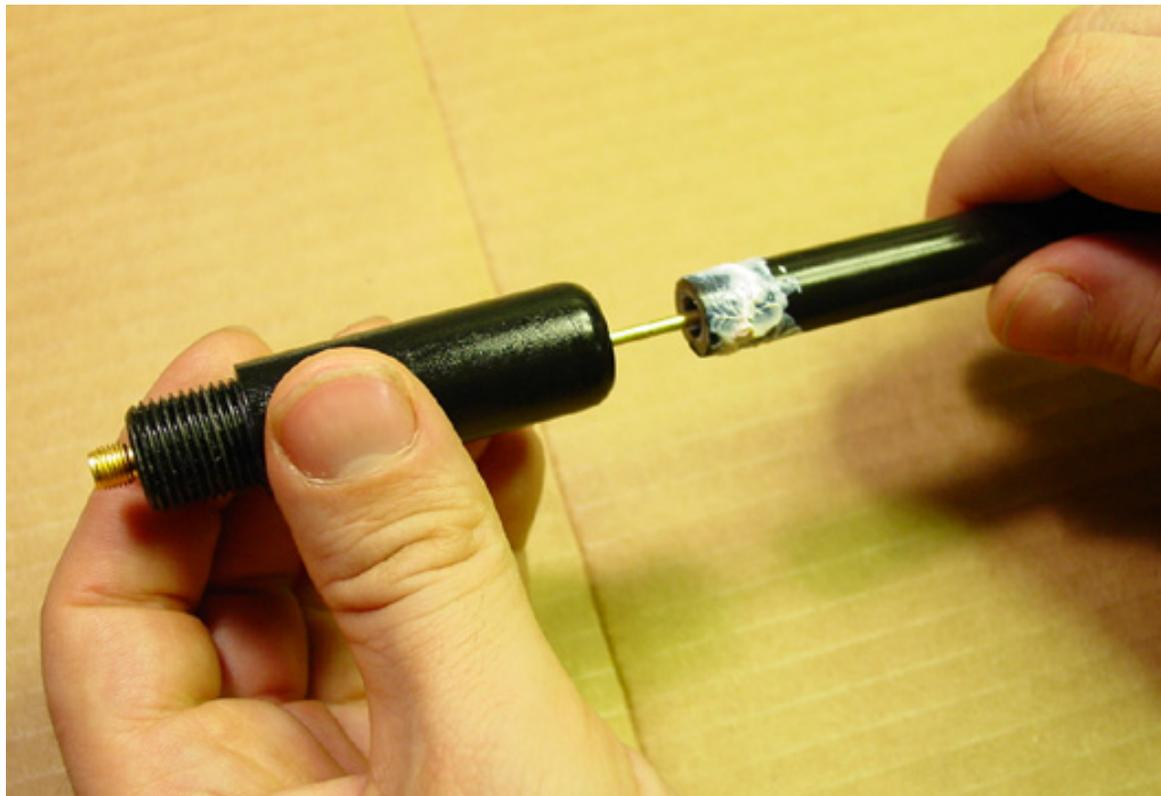
Figure 17. Epoxy applied to radome prior to insertion into threaded mounting component.
