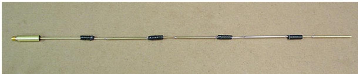
Figure 13. Anti-rattling tape applied to the coils.
