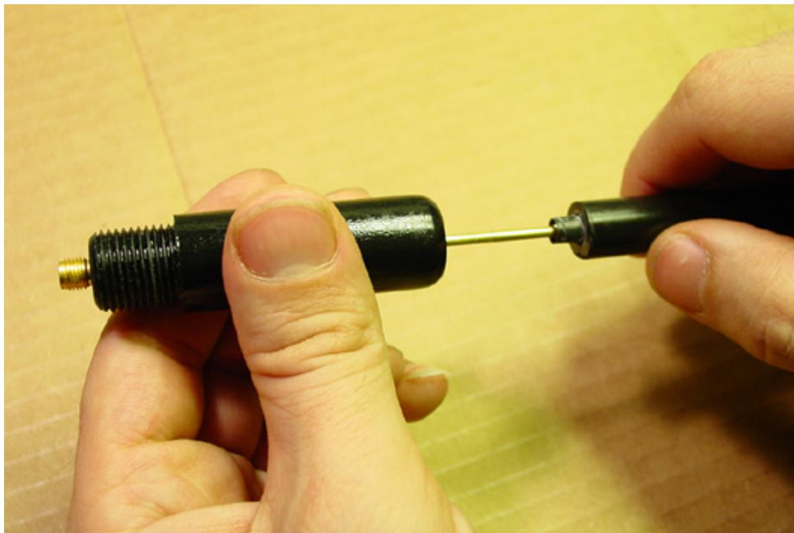
Figure 16. Retracting the radome once decoupler is set.
