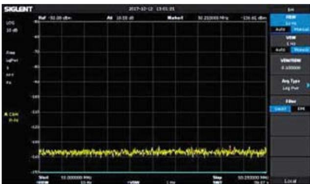
Foto 8 - Power-Supply NOISE @ 50.2 MHz – Null-Power
