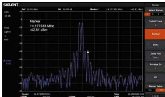
Fig. 6 - Two-Tone-Test @ 1,5 kW (14 MHz)
