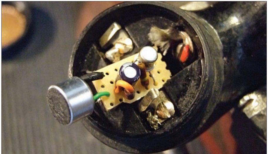
Fig. 3: The H-33F/PF handset showing the space for the microphone.
