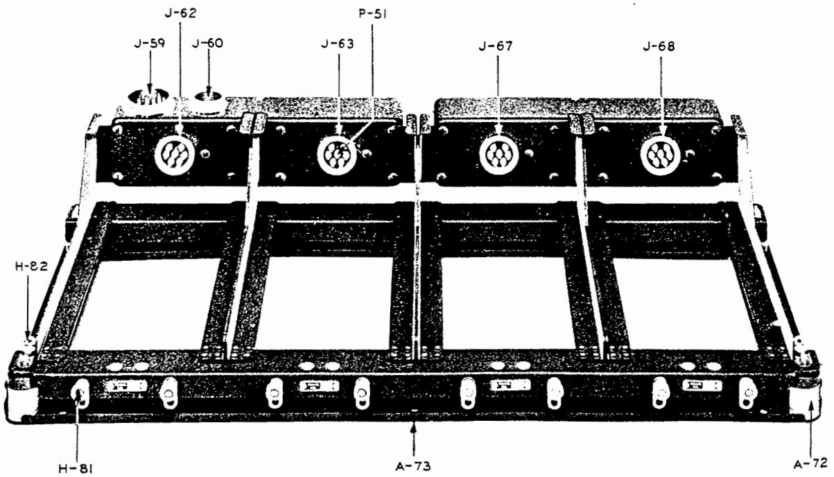
FIGURE 17B—RACK FT-331-A AND MOUNTING FT-332-A, FRONT VIEW
