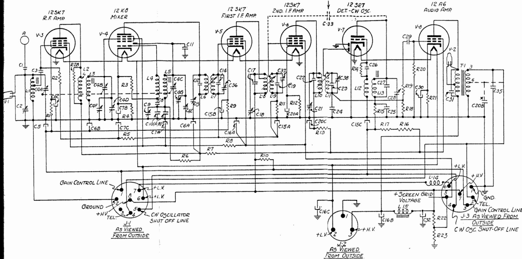
CIRCUITS IN RF COIL SET, IF COUPLING UNITS, CW OSCILLATOR, & OUTPUT TRANSFORMER.
