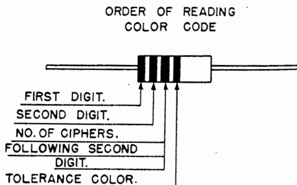
EXAMPLE: 360,000 ohms  $\pm 5\%$ : First method: orange body, blue tip, yellow dot, and a gold colored tip to represent the tolerance. Second method: orange, blue, yellow, and gold rings, starting at one end.
