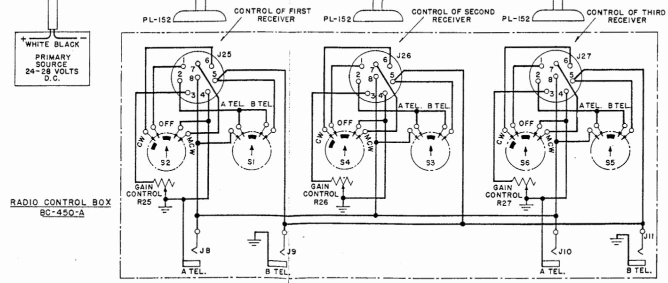
FIGURE 26-RADIO SET SCR-274-N RECEIVING EQUIPMENT, SCHEMATIC CIRCUIT DIAGRAM
