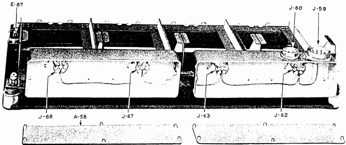
FIGURE 17A—RACK FT-331-A AND MOUNTING FT-332-A, REAR VIEW WITH COVER OF RACK REMOVED
