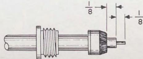
7. CUT INNER DIELECTRIC  $\frac{1}{8}$  INCH FROM BRAID, BEING CAREFUL NOT TO NICK INNER CONDUCTOR AND CUT OFF INNER CONDUCTOR  $\frac{1}{8}$  INCH FROM END OF DIELECTRIC.
