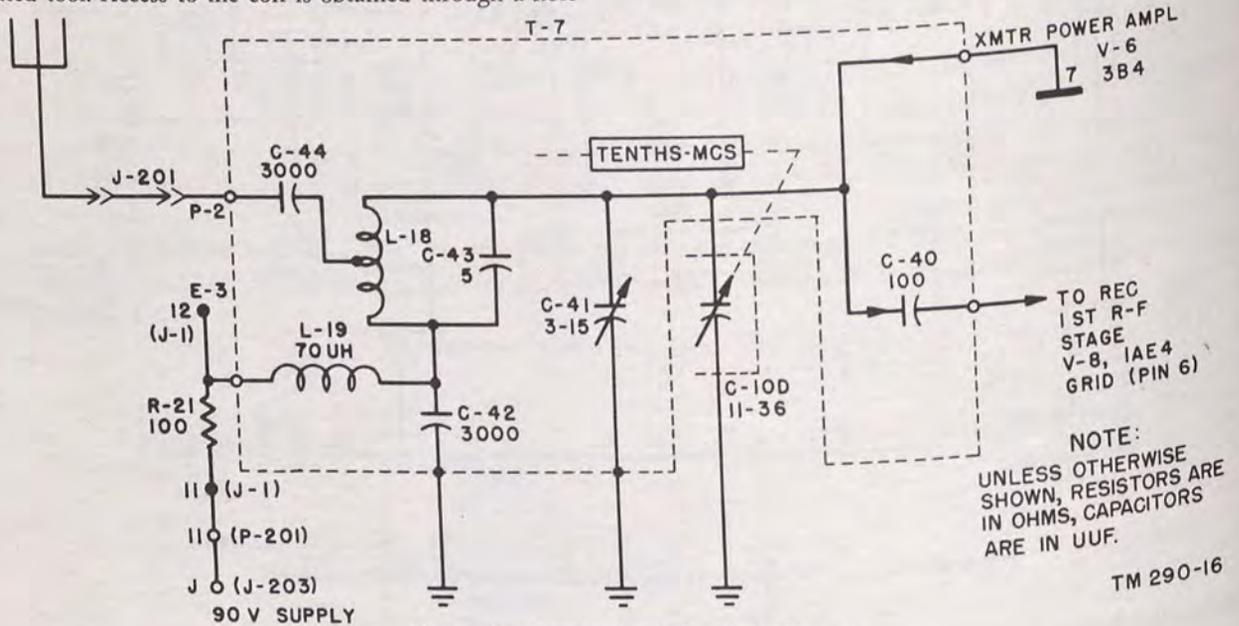
Figure 16. Antenna circuit, functional diagram.
