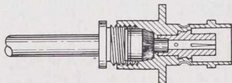
10. THE ASSEMBLY FOR PLUGS IS THE SAME EXCEPT FOR THE USE OF MALE CONTACTS AND A UG-260/U BODY.
