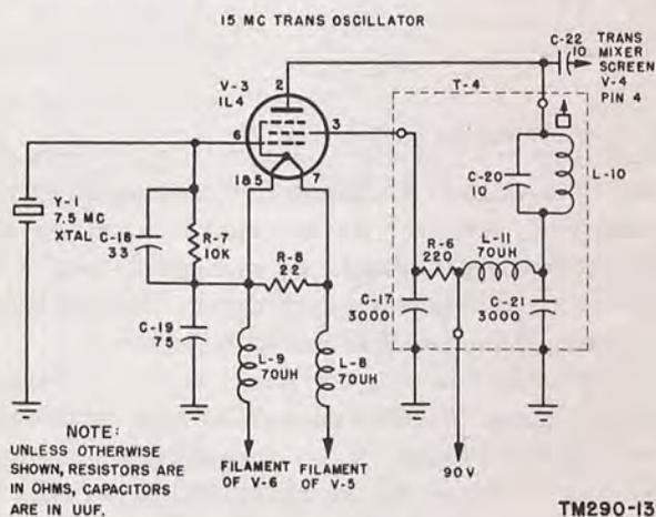
Figure 13. 15-mc transmitter oscillator, functional diagram.
