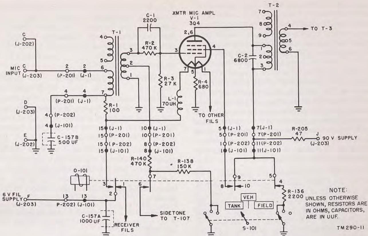
Figure 11. Microphone and microphone amplifier circuits, functional circuit diagram.
