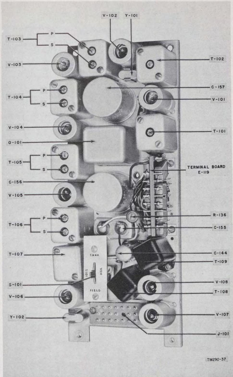
Figure 37. Receiver-Transmitter RT-70/GRC, component side of i-f chassis.
