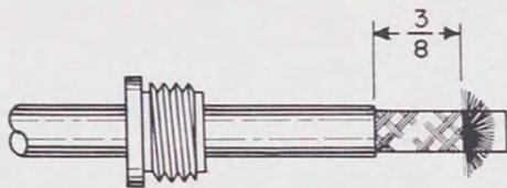
3. CUT OFF INNER INSULATION AND WIRE UNDER BRAID  $\frac{3}{8}$  FROM END OF JACKET.
