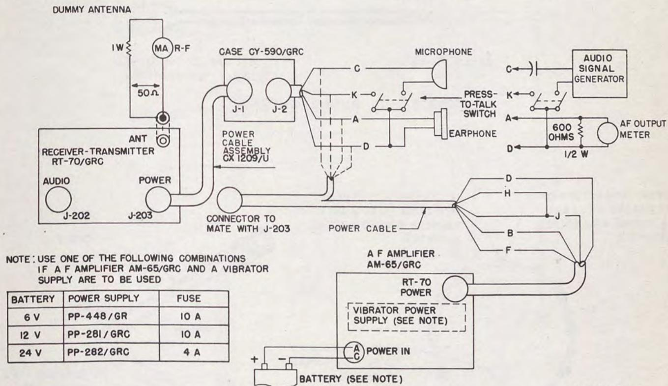
Figure 29. Test set-up for operational and trouble-shooting checks.
