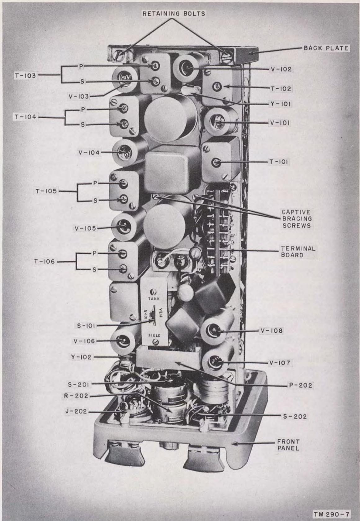
Figure 7. Receiver-Transmitter RT-70/GRC, case removed, view of i-f chassis (left side of panel-and-chassis assembly).
