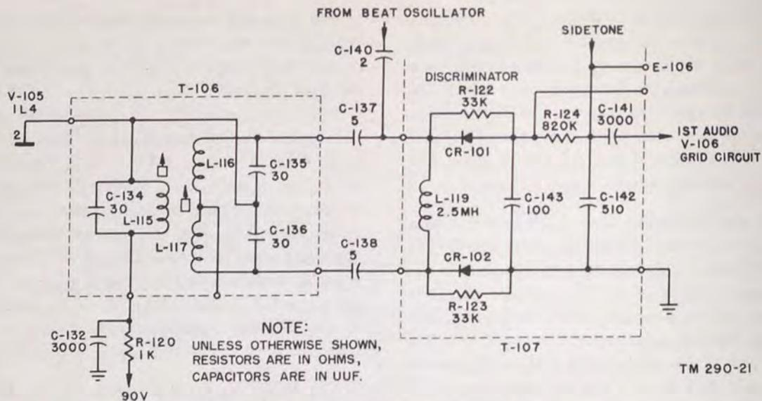
Figure 21. Discriminator circuit, functional diagram.
