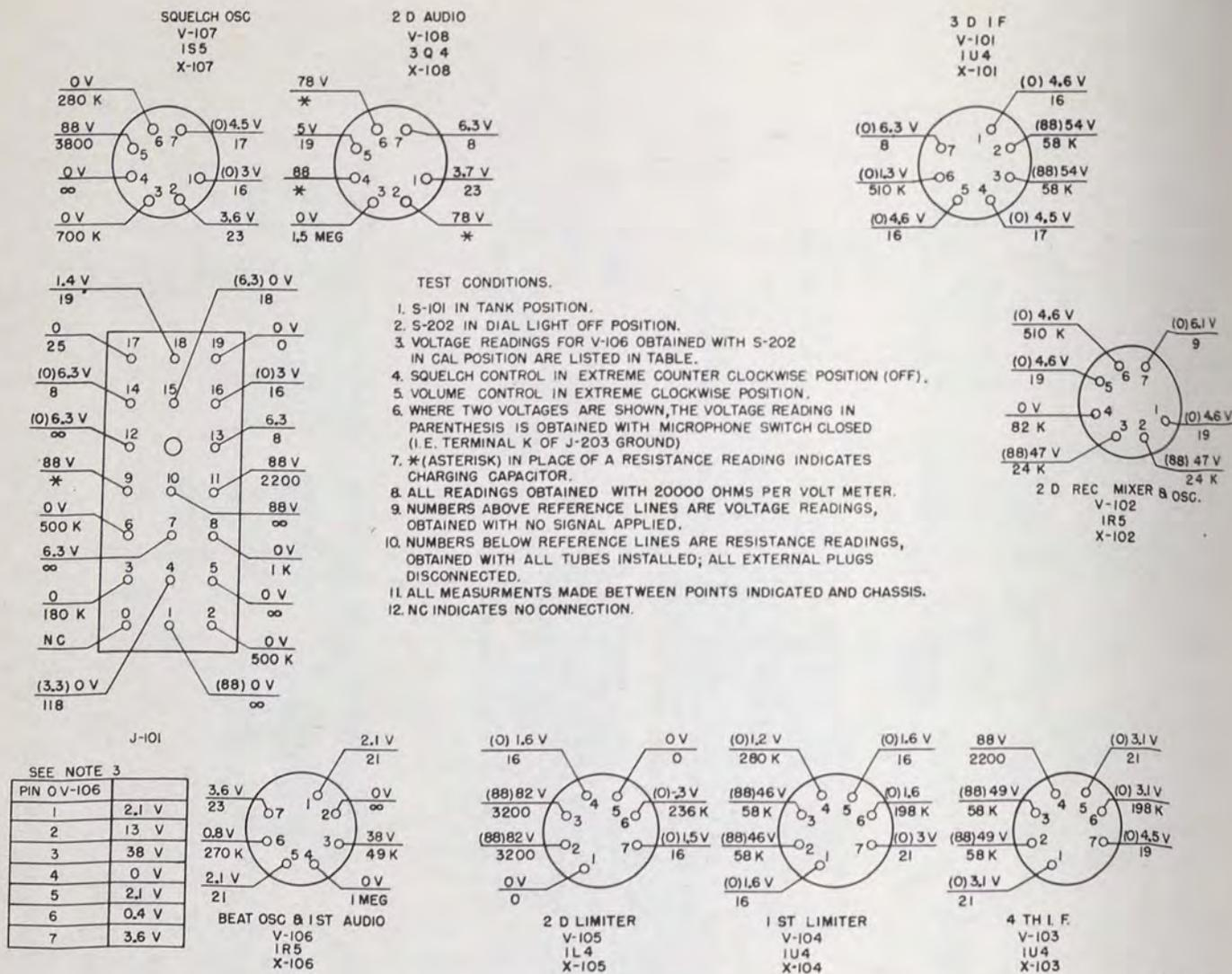
Figure 34. Resistance and voltage data, i-f chassis.
