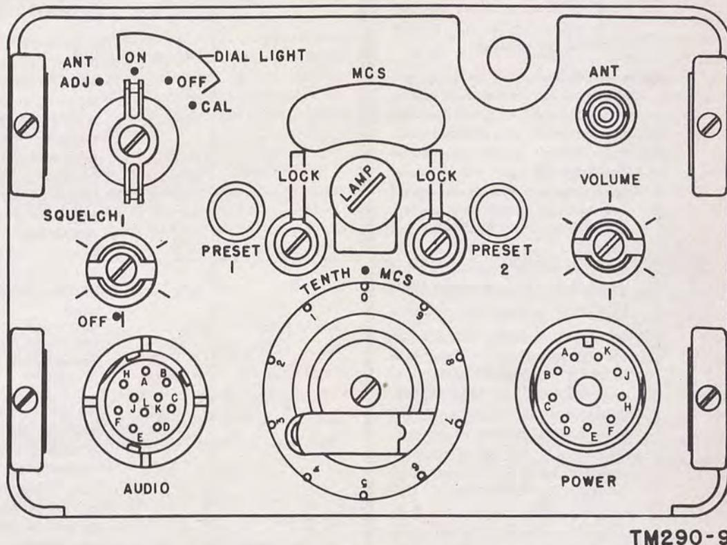
Figure 9. Receiver-Transmitter RT-70/GRC, panel controls and connectors.
