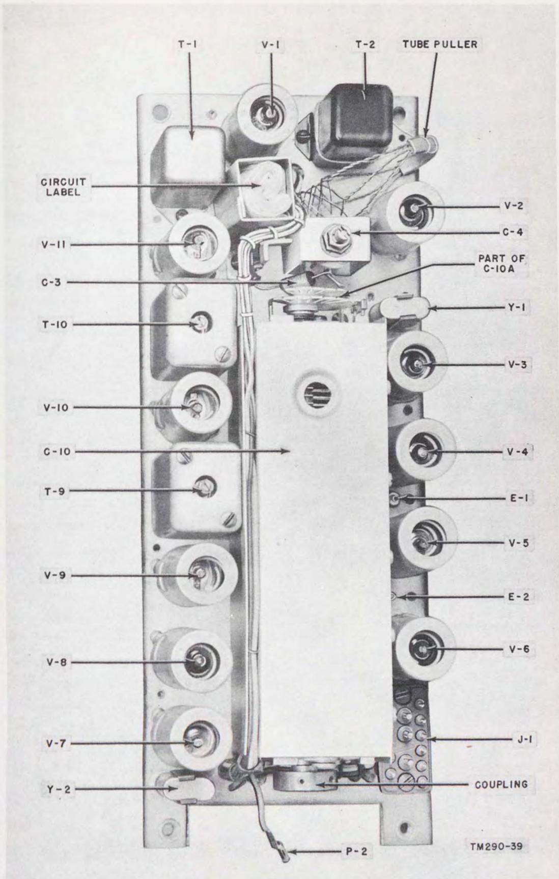
Figure 39. Receiver-Transmitter RT-70/GRC, component side of r-f chassis.
