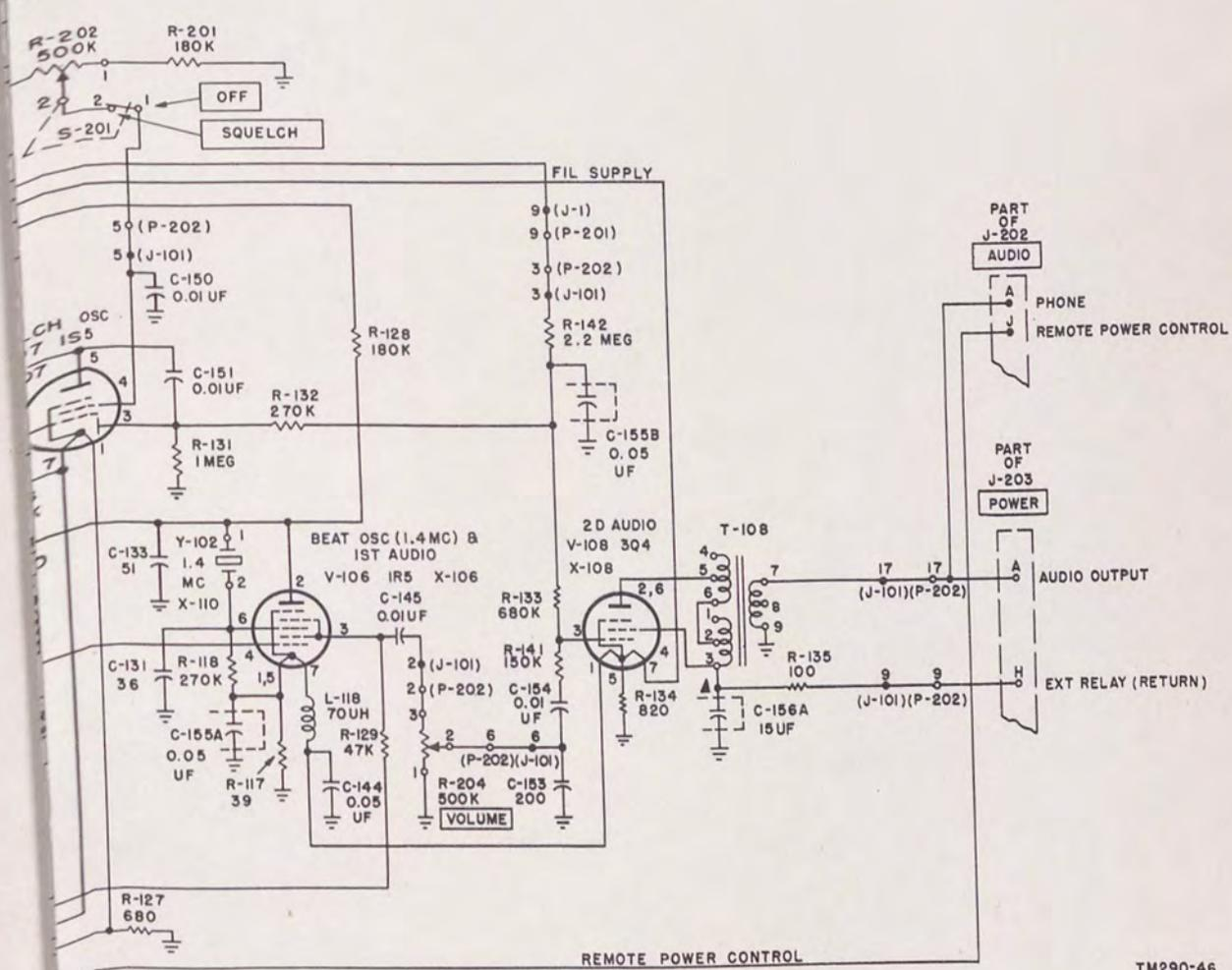
Figure 47. Receiver-Transmitter RT-70/GRC, schematic diagram.
