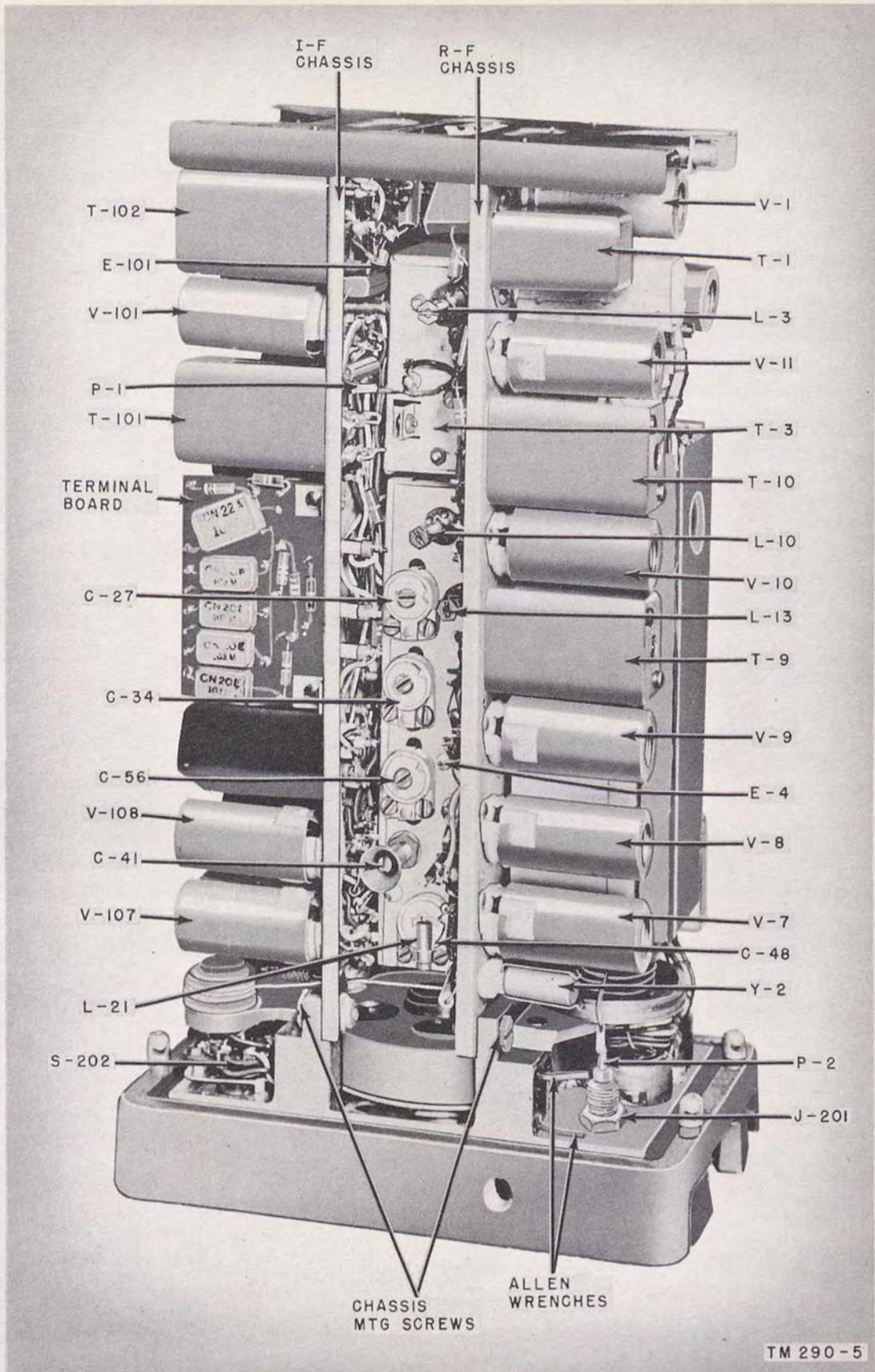
Figure 5. Receiver-Transmitter RT-70/GRC, case removed, top view of panel-and-chassis assembly.
