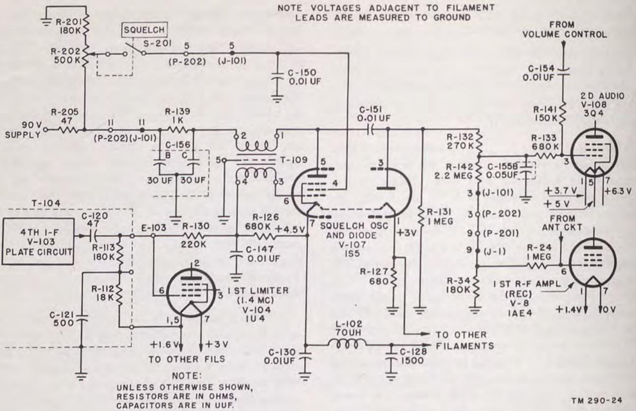
Figure 24. Squelch circuits, functional diagram.
