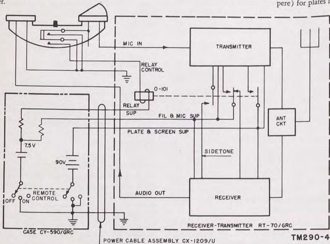
Figure 3. Application of Receiver-Transmitter RT-70/GRC to Radio Set AN/PRC-16, simplified block diagram.
