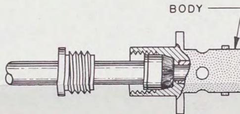
9. PUSH INTO BODY AS FAR AS IT WILL GO, THEN SLIDE NUT INTO BODY AND SCREW INTO PLACE, WITH WRENCH, UNTIL MODERATELY TIGHT. HOLD CABLE AND SHELL RIGIDLY AND ROTATE NUT.
