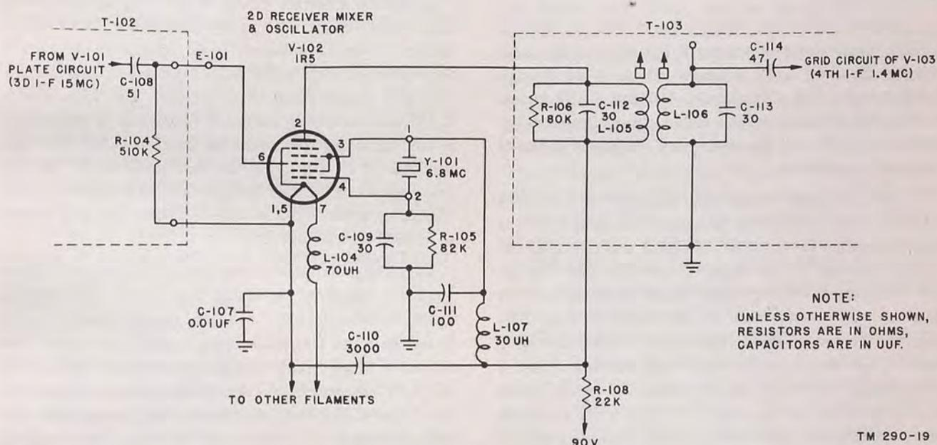
Figure 19. Second receiver mixer and oscillator, functional diagram.
