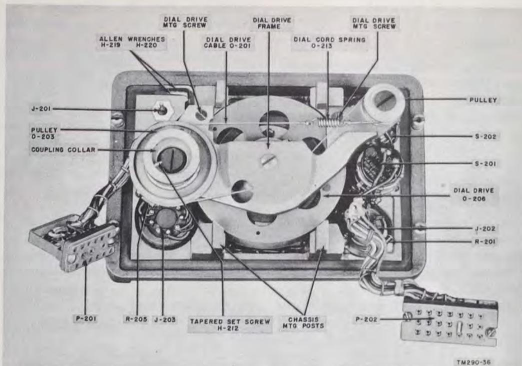
Figure 36. Receiver-Transmitter RT-70/GRC, rear view of panel.
