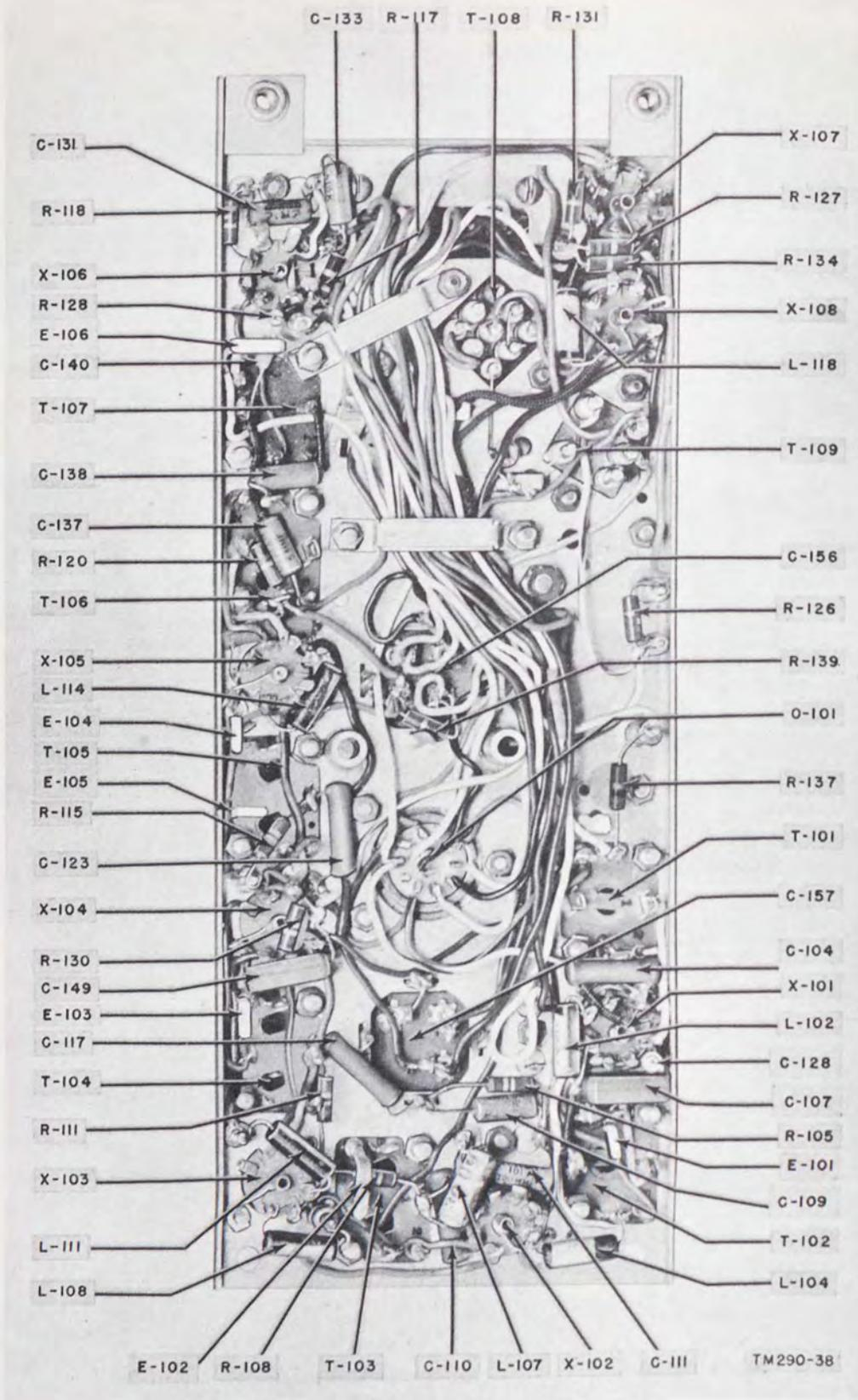
Figure 38. Receiver-Transmitter RT-70/GRC, wiring side of i-f chassis.
