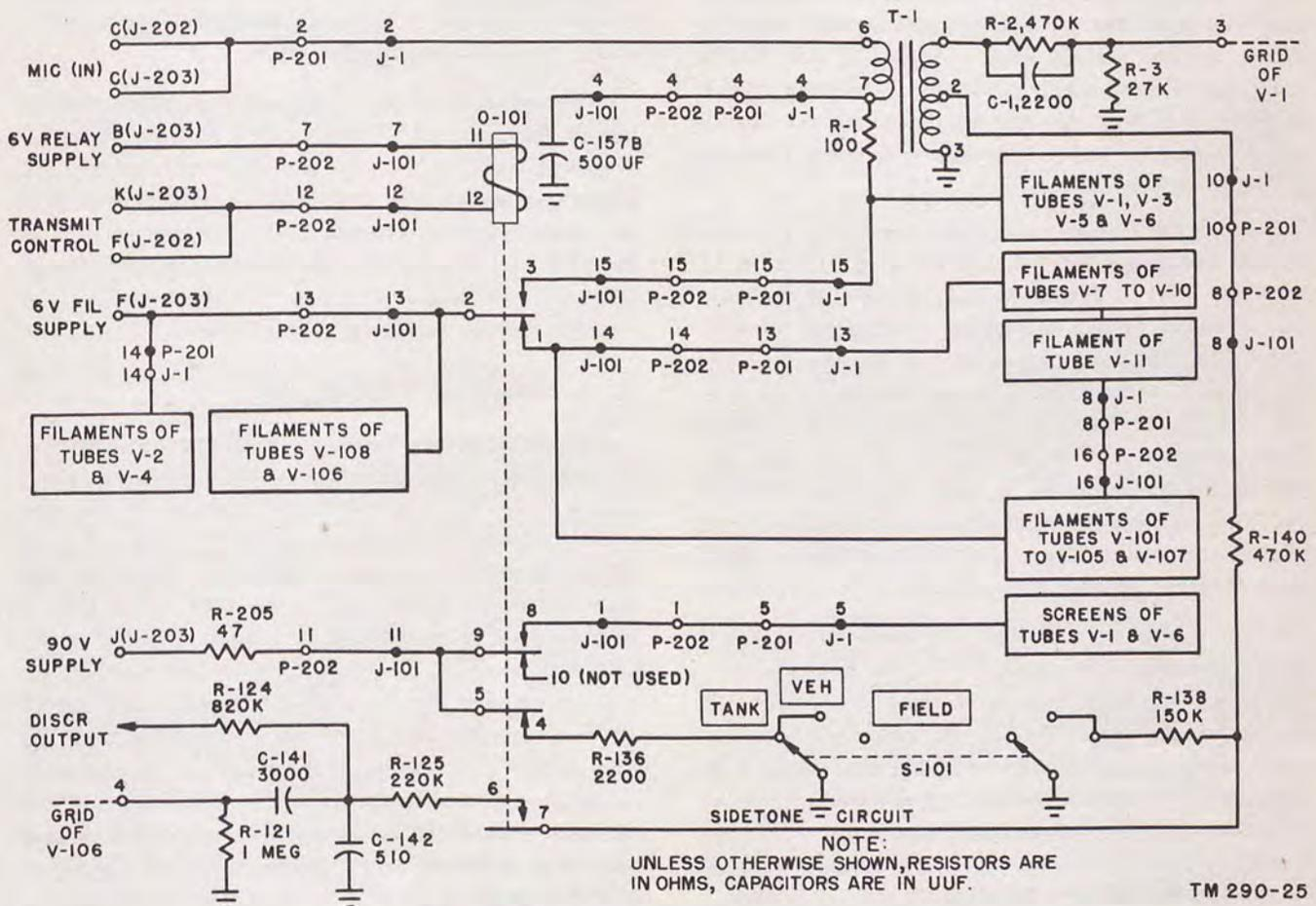
Figure 25. Control circuits, functional diagram.
