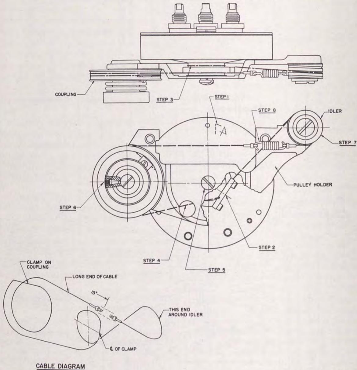
Figure 43. Replacement of dial drive cable.
