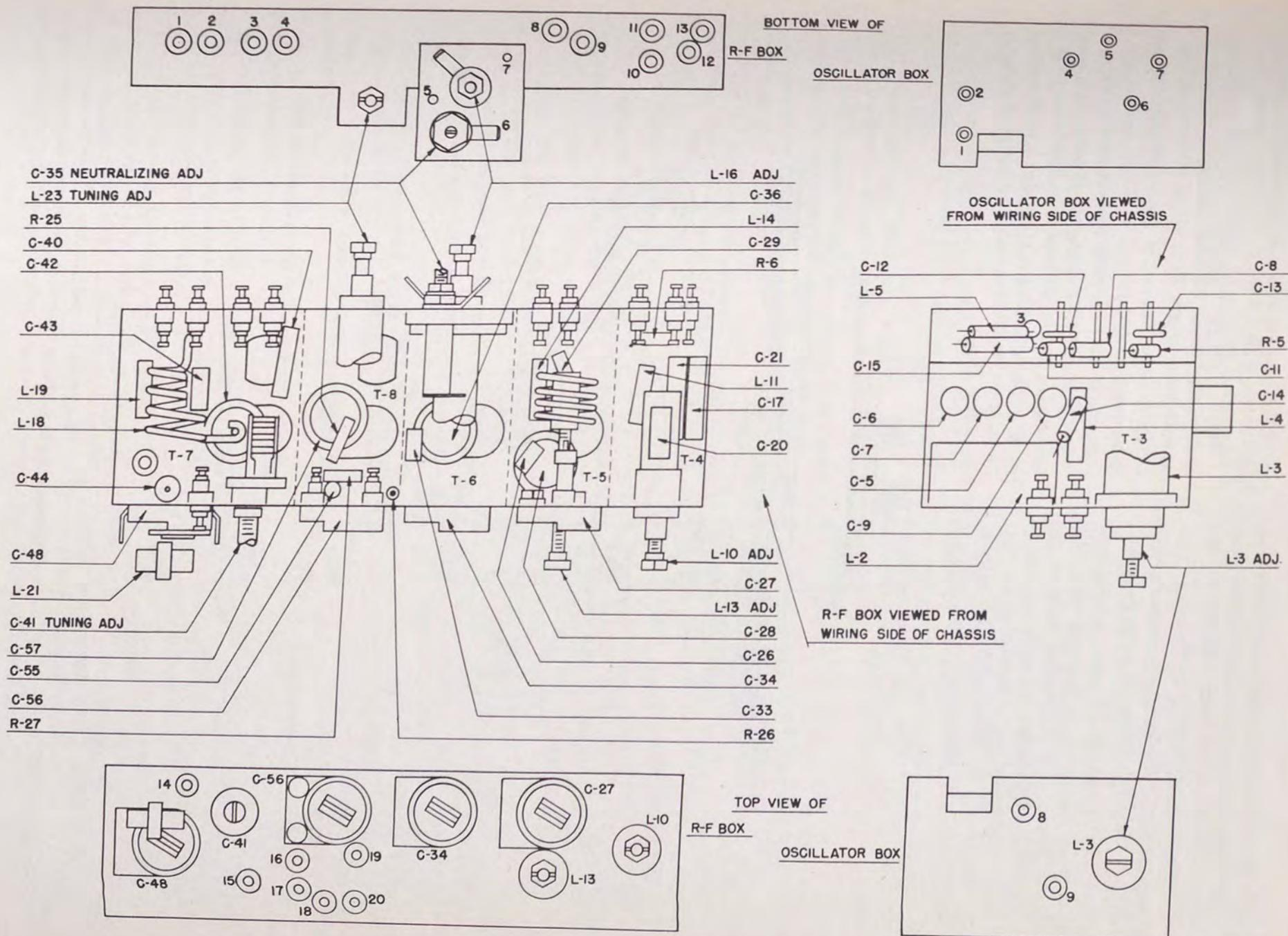
Figure 42. RF coil compartment, component location diagram.
