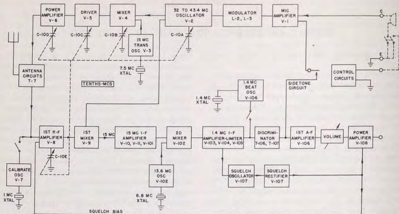
Figure 10. Receiver-Transmitter RT-70/GRC, functional block diagram.
