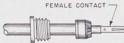
8. TIN INSIDE HOLE OF FEMALE CONTACT, TIN CENTER CONDUCTOR OF CABLE, SLIP FEMALE CONTACT IN PLACE AND SOLDER, REMOVE EXCESS SOLDER. BE SURE CABLE DIELECTRIC IS NOT HEATED EXCESSIVELY AND SWOLLEN SO AS TO PREVENT DIELECTRIC ENTERING BODY.
