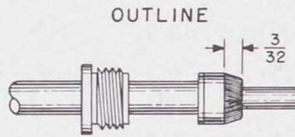
6. WITH SLEEVE IN PLACE, COMB OUT BRAID, FOLD BACK SMOOTH AS SHOWN, AND TRIM TO  $\frac{3}{32}$  INCH FROM END.
