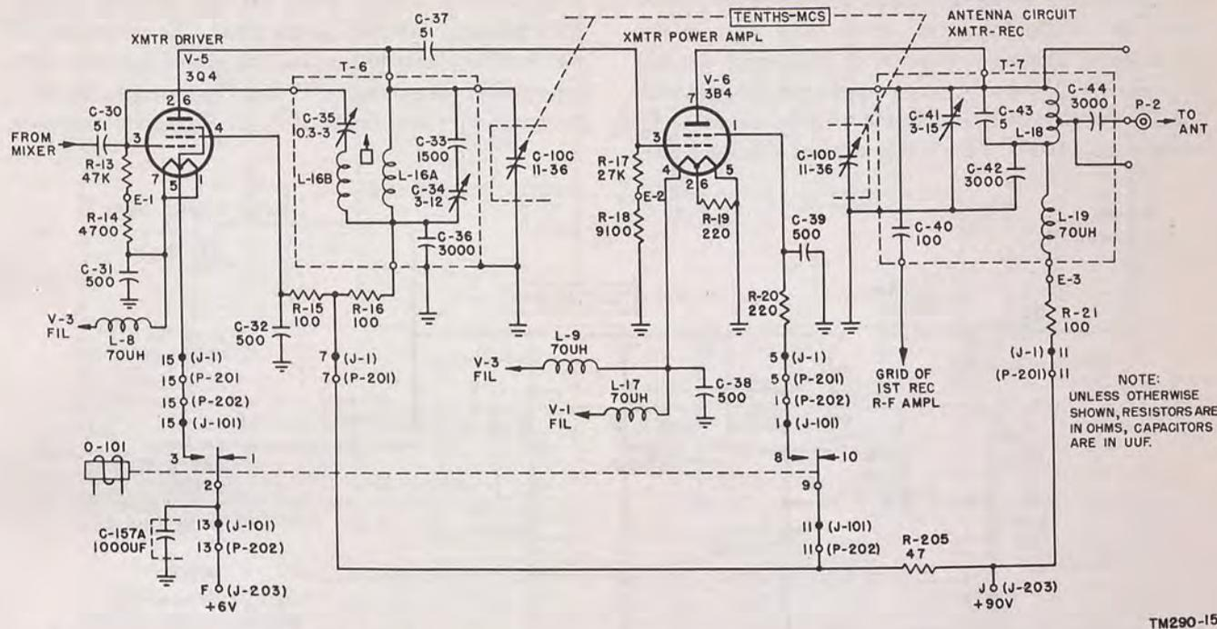
Figure 15. Transmitter driver and power amplifier circuits, functional diagram.
