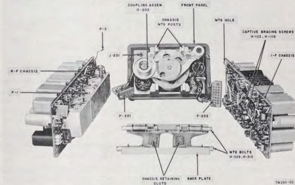
Figure 35. Receiver-Transmitter RT-70/GRC, disassembled view.
