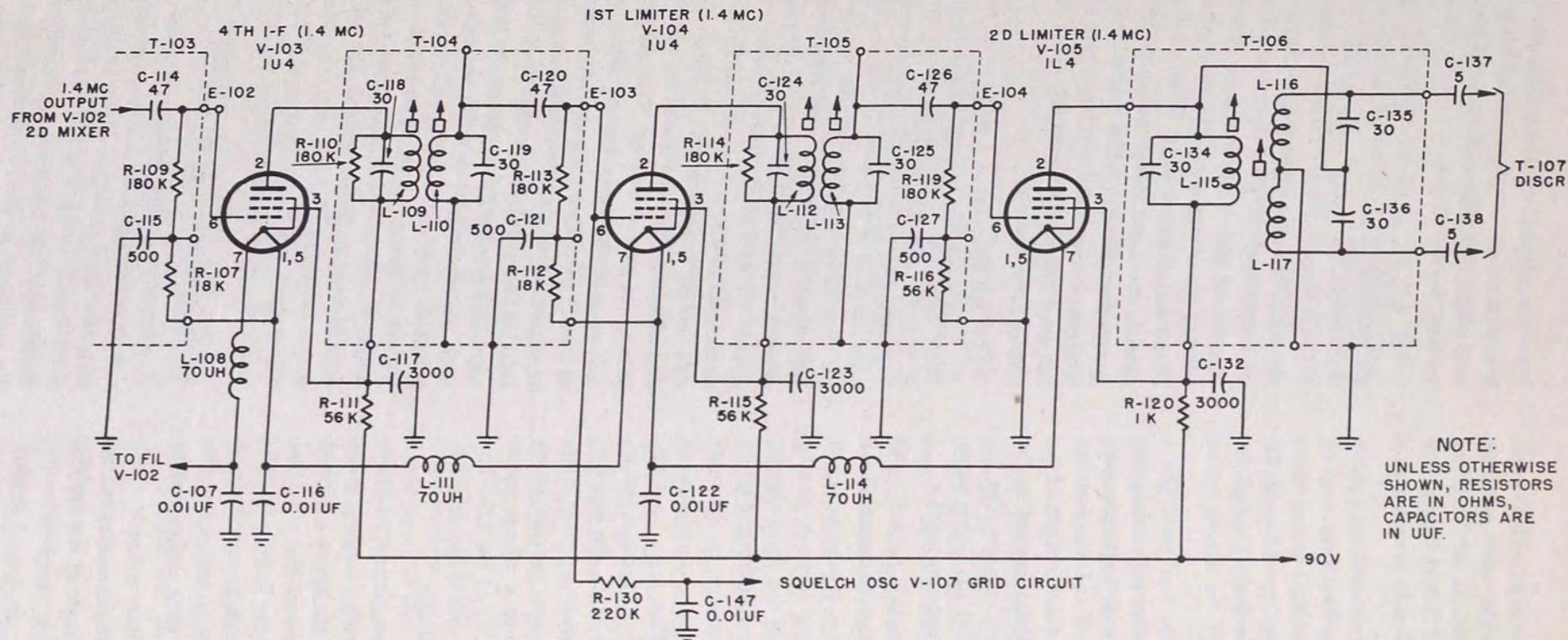
Figure 20. 1.4-mc i-f amplifier and limiters circuits, functional diagram.
