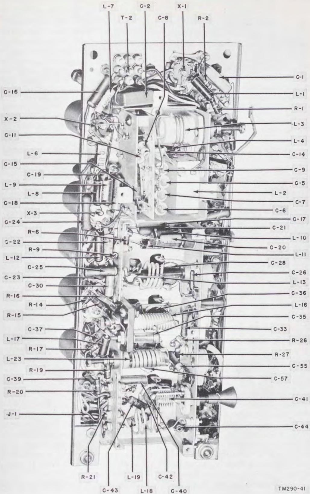
Figure 41. Receiver-Transmitter RT-70/GRC, wiring side of r-f chassis, with coil compartment covers removed.
