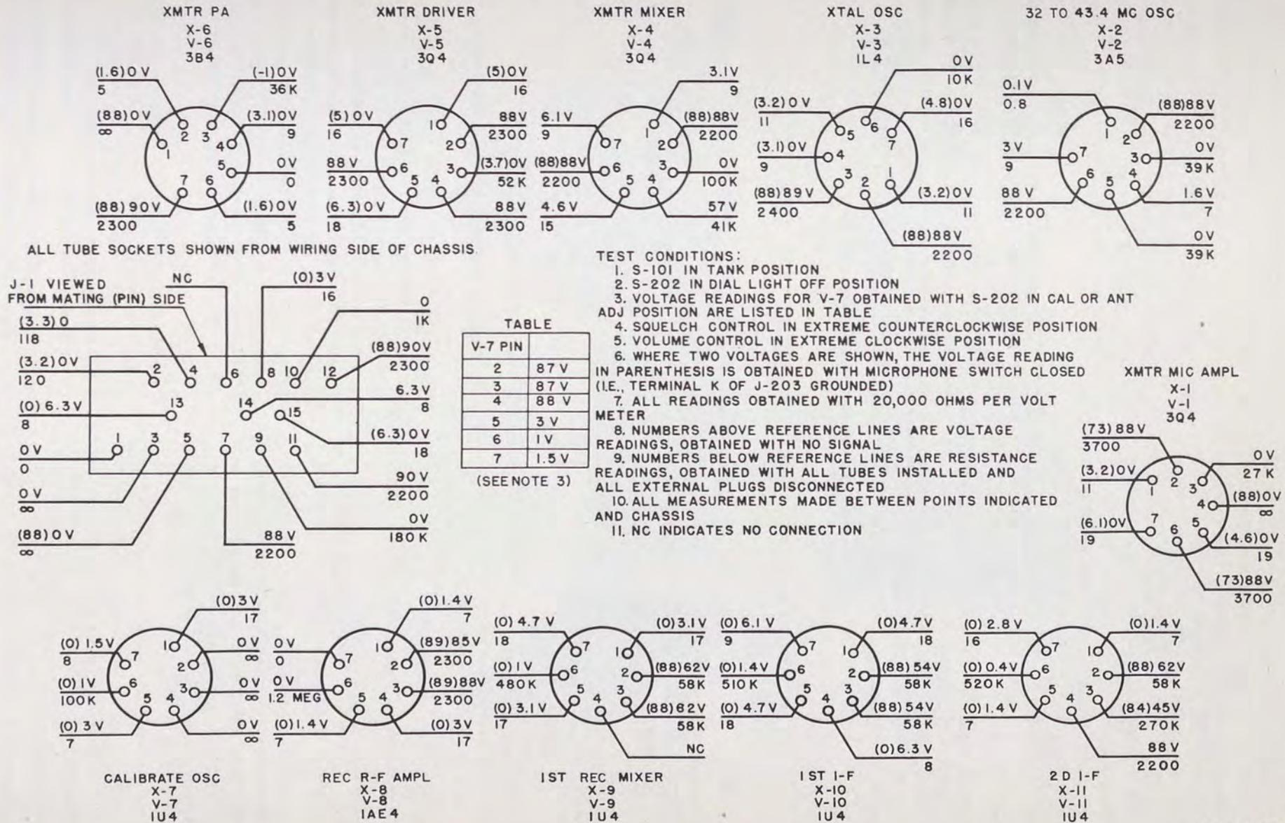
Figure 33. Resistance and voltage data, r-f chassis.
