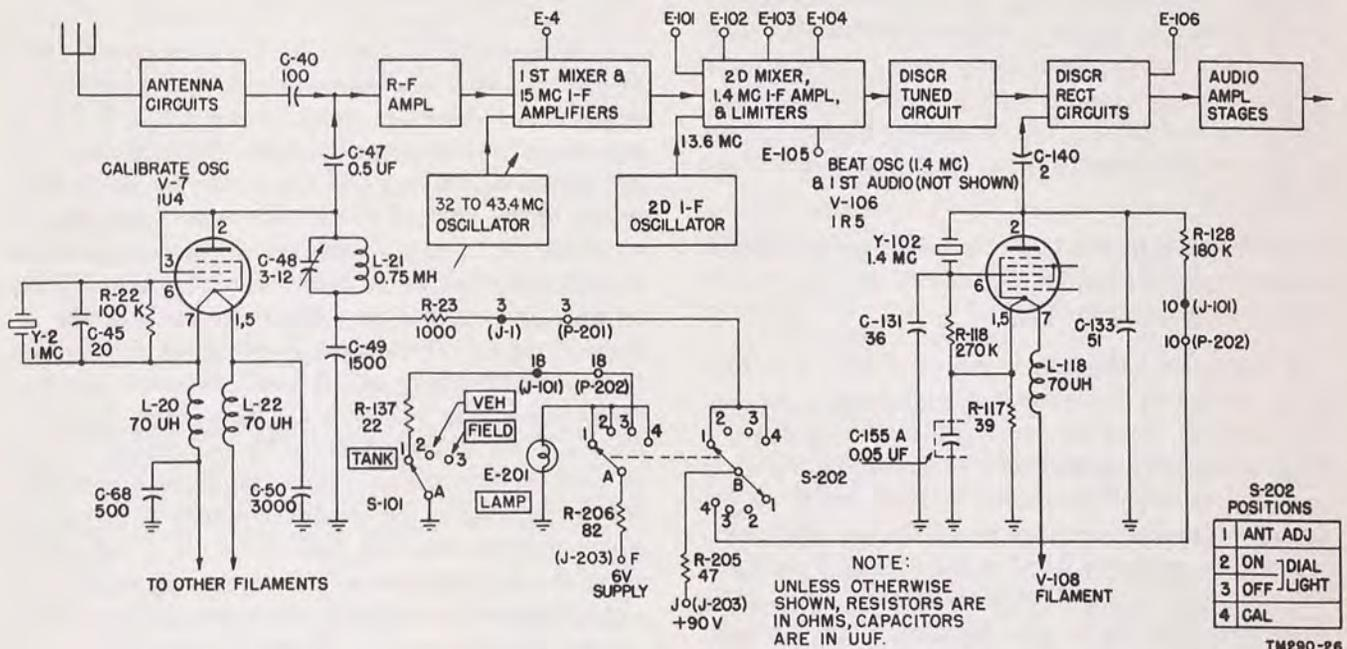
Figure 26. Calibrate and beat oscillator circuits, functional diagram.
