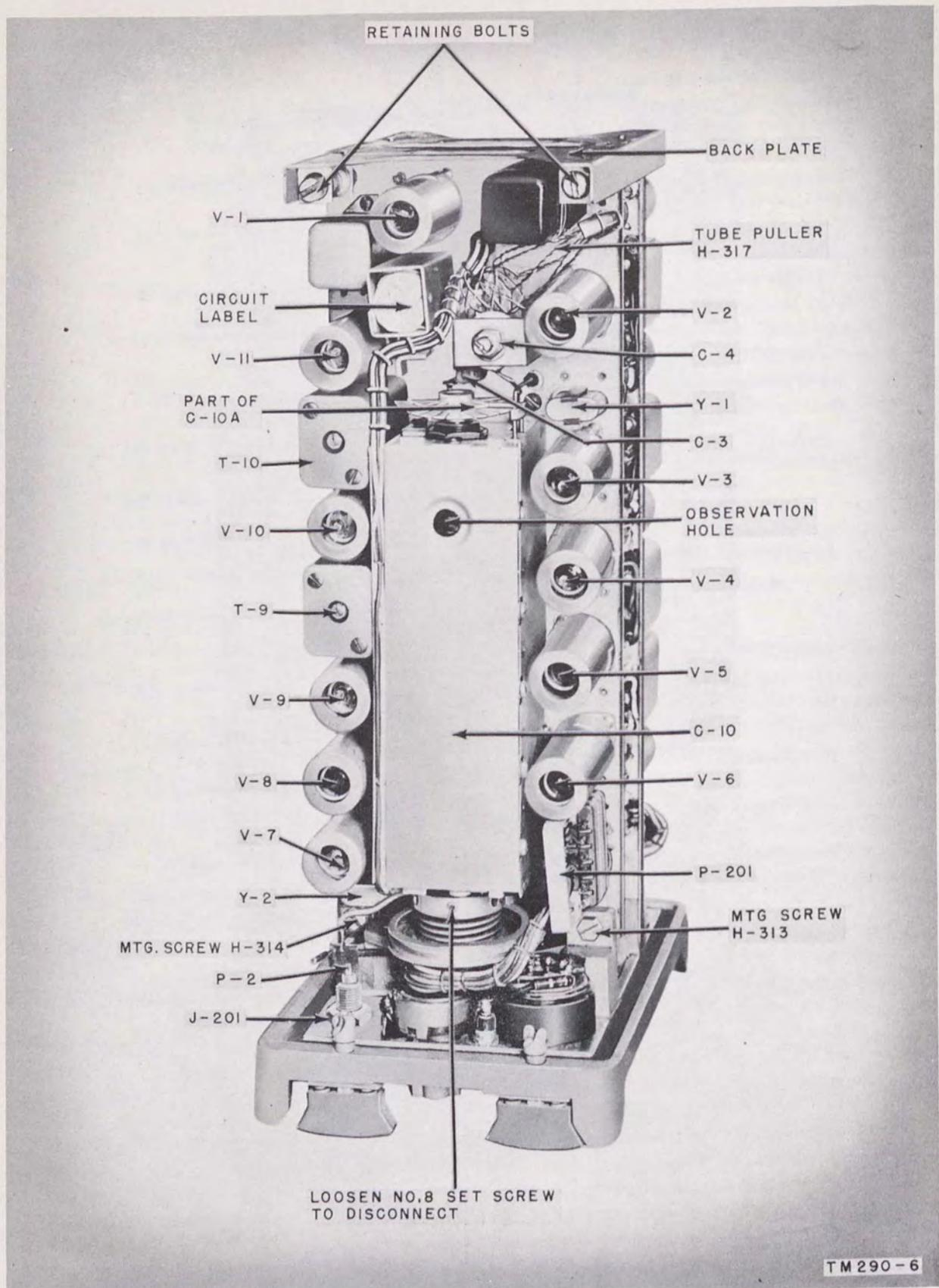
Figure 6. Receiver-Transmitter RT-70/GRC, case removed, view of r-f chassis (right side of panel-and-chassis assembly).
