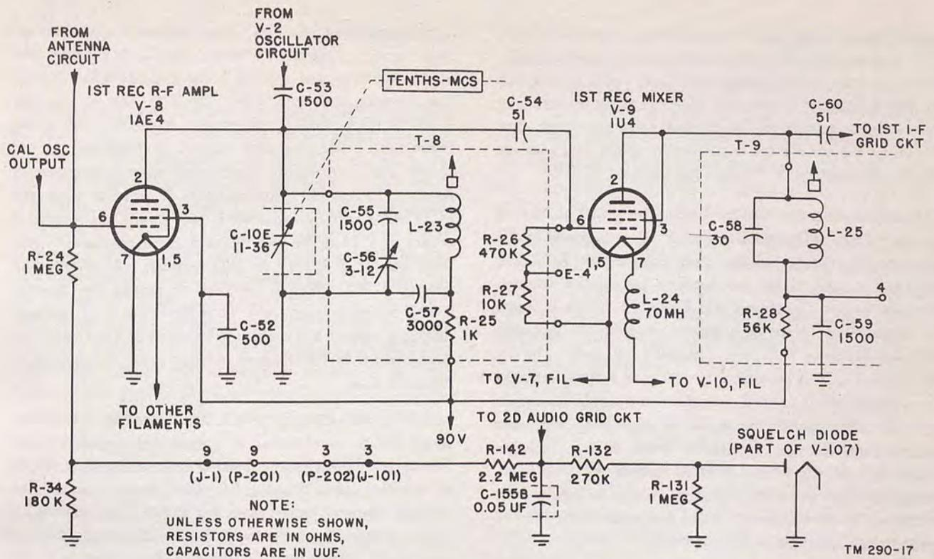
Figure 17. Receiver first r-f amplifier and mixer circuits, functional diagram.
