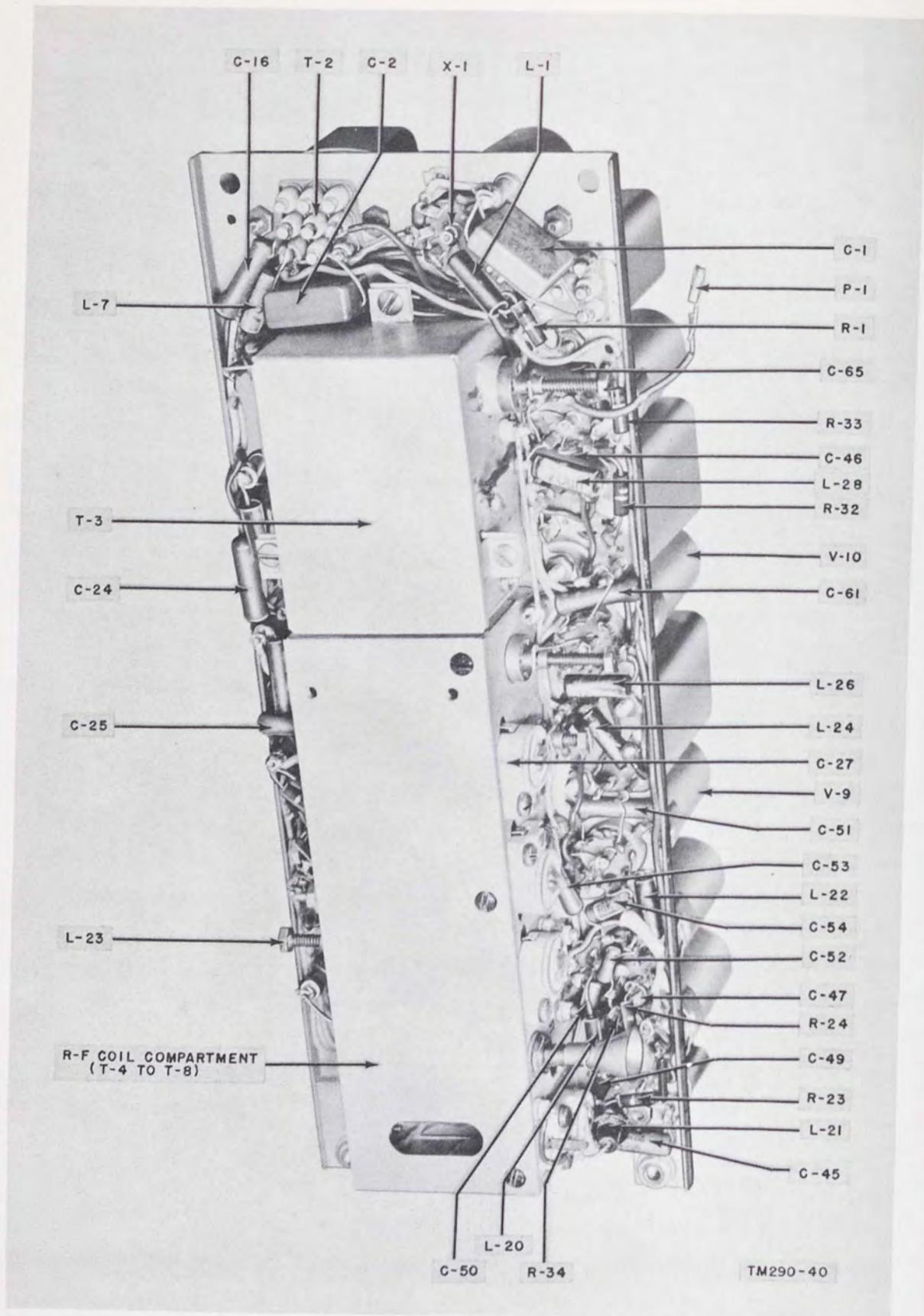
Figure 40. Receiver-Transmitter RT-70/GRC, wiring side of r-f chassis.
