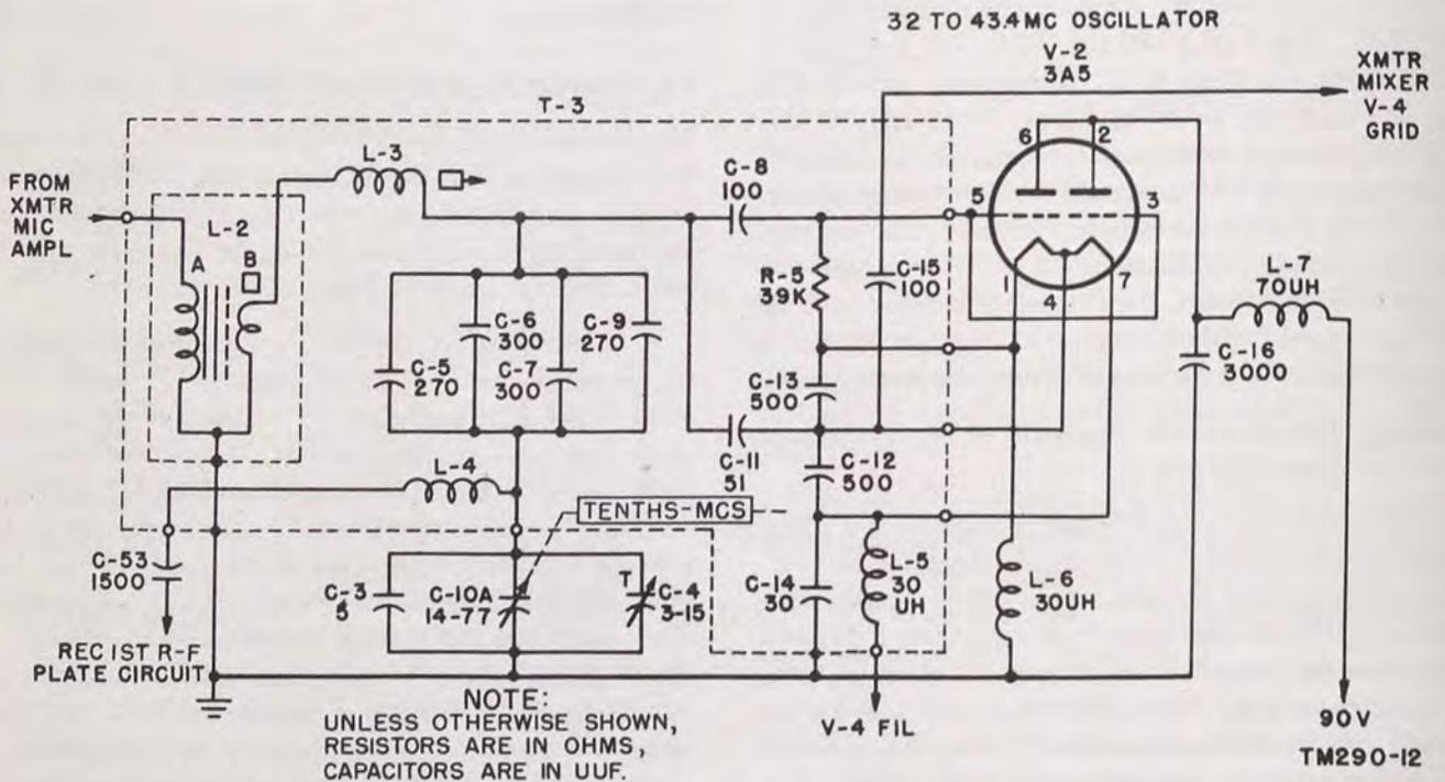
Figure 12. Reactance modulator and 32- to 43.4-mc oscillator circuits, functional diagram.
