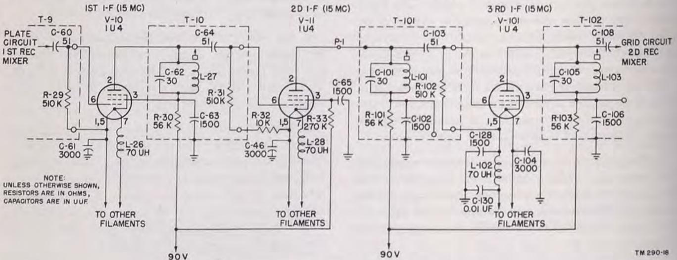
Figure 18. 15-mc i-f amplifiers, functional diagram.
