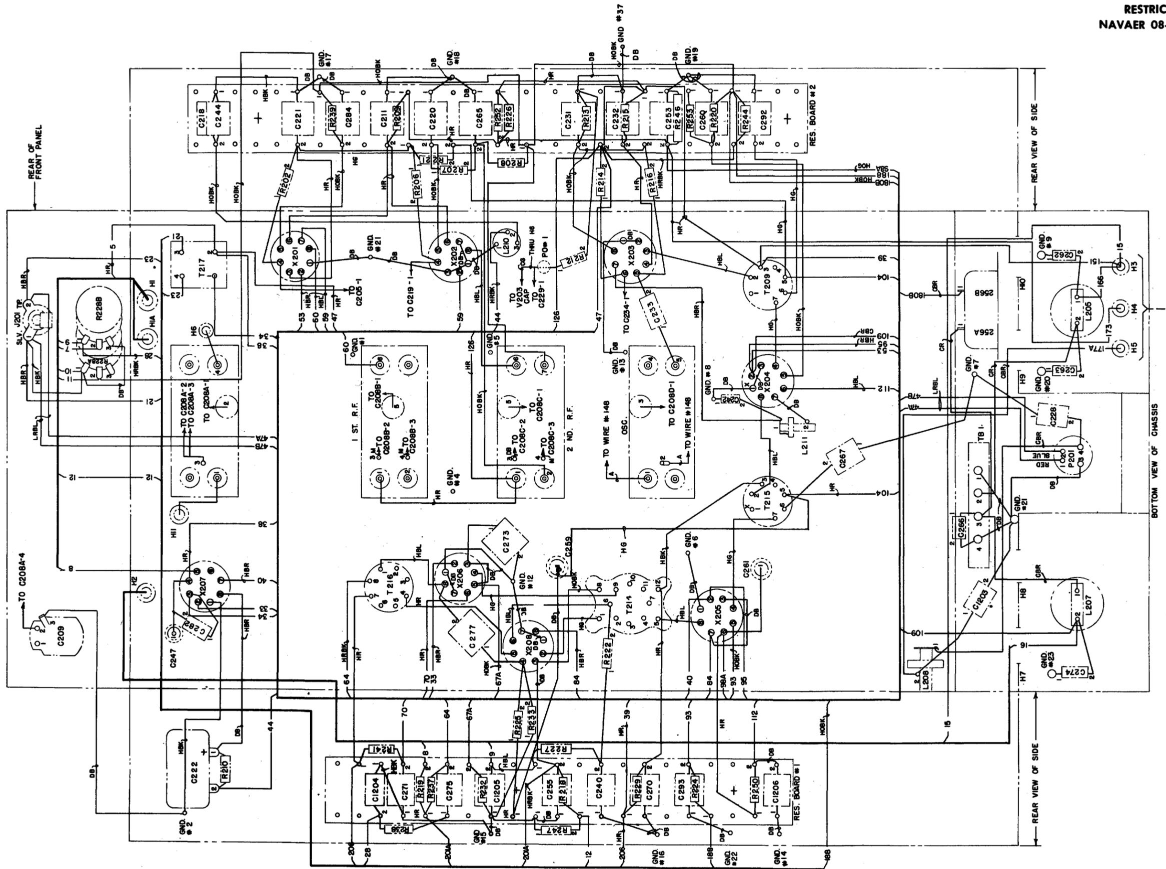
Connection Diagram, Type CG-46116 Receiver Unit No. 2
