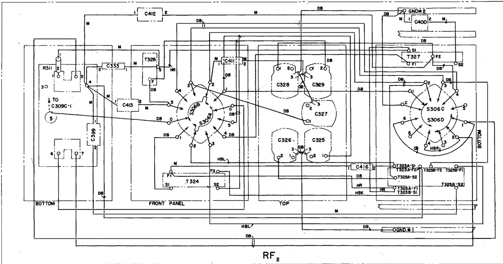
Connection Diagram, R-f Units, Type CG-46117 Radio Receiver No. 3
