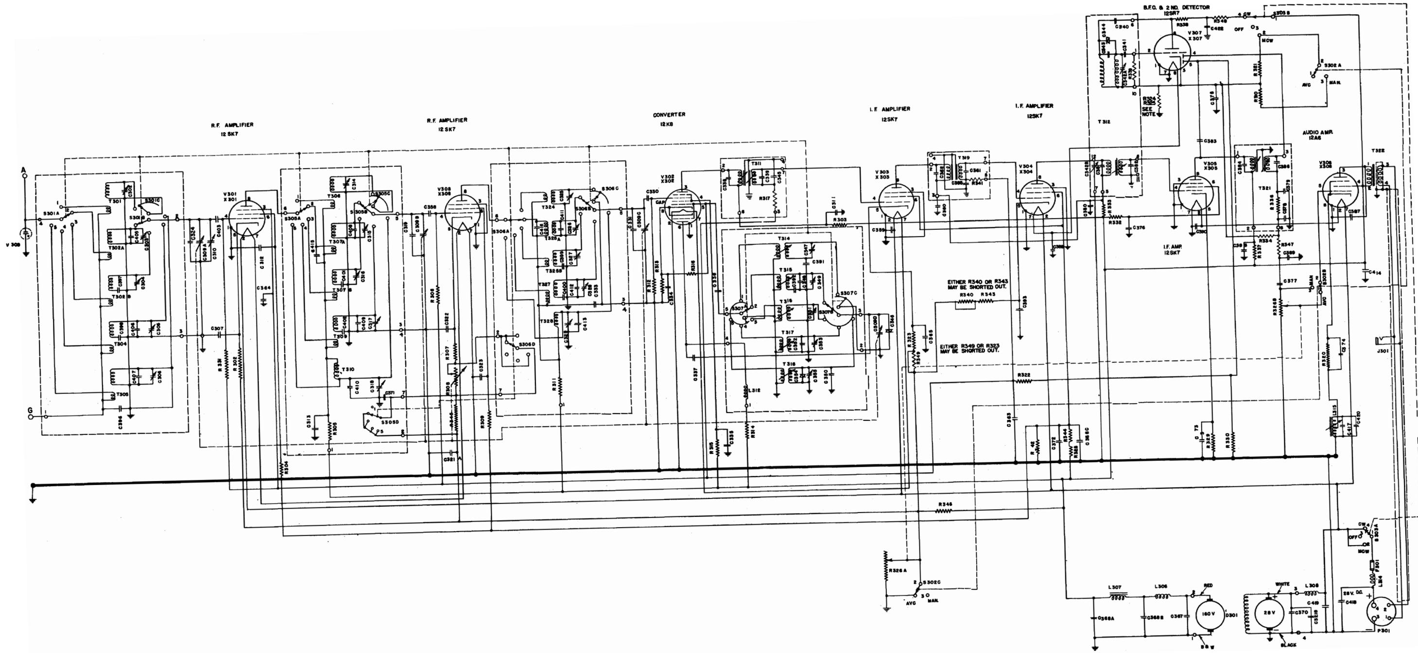
Schematic Diagram, Type CG-46117 Receiver Unit No. 3
