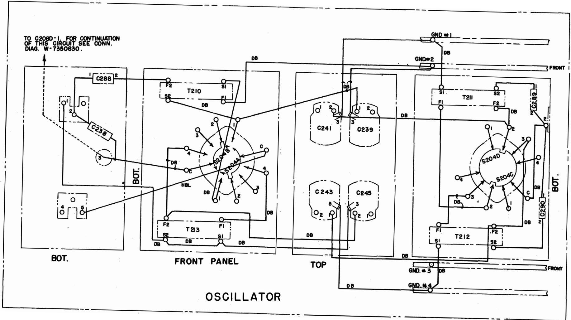
Connection Diagram, R-f Units, Type CG-46116 Radio Receiver No. 2
