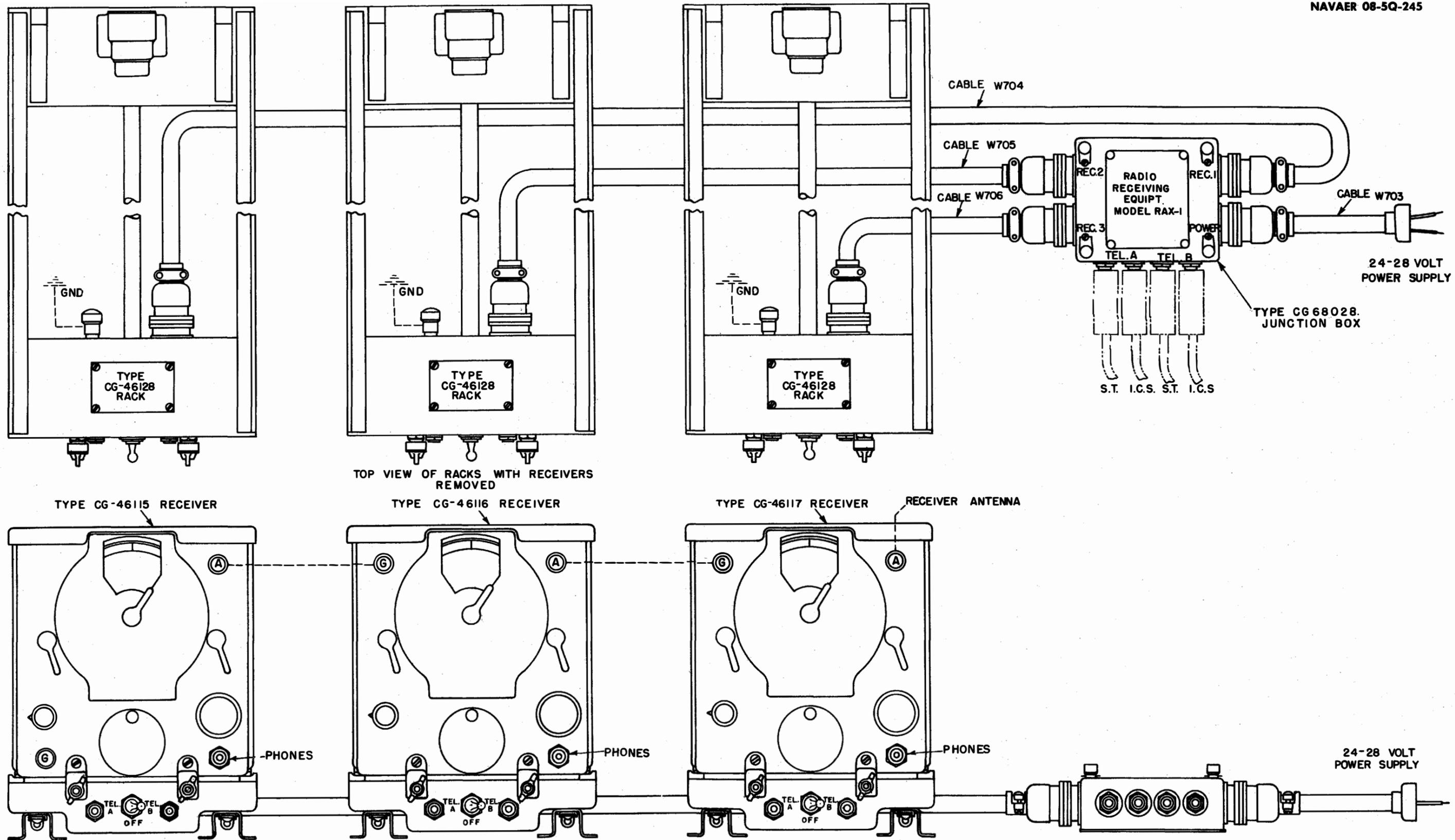
Cabling Diagram, Model RAX-1 Radio Receiving Equipment
