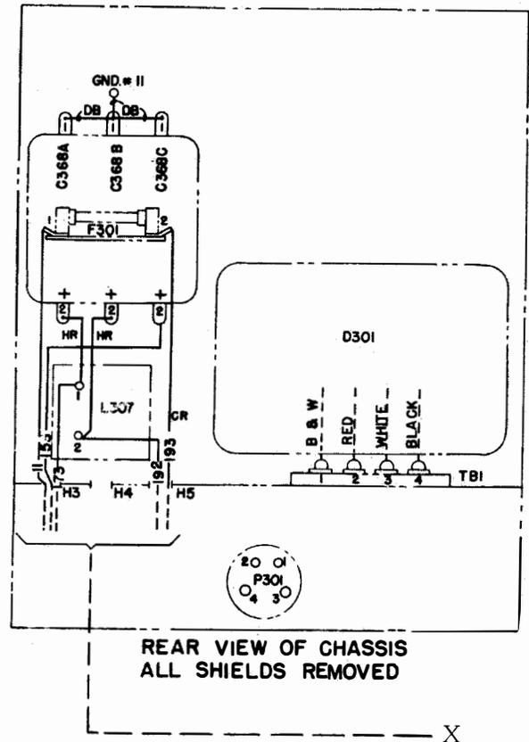
Connection Diagram, Type CG-46117 Receiver Unit No. 3
