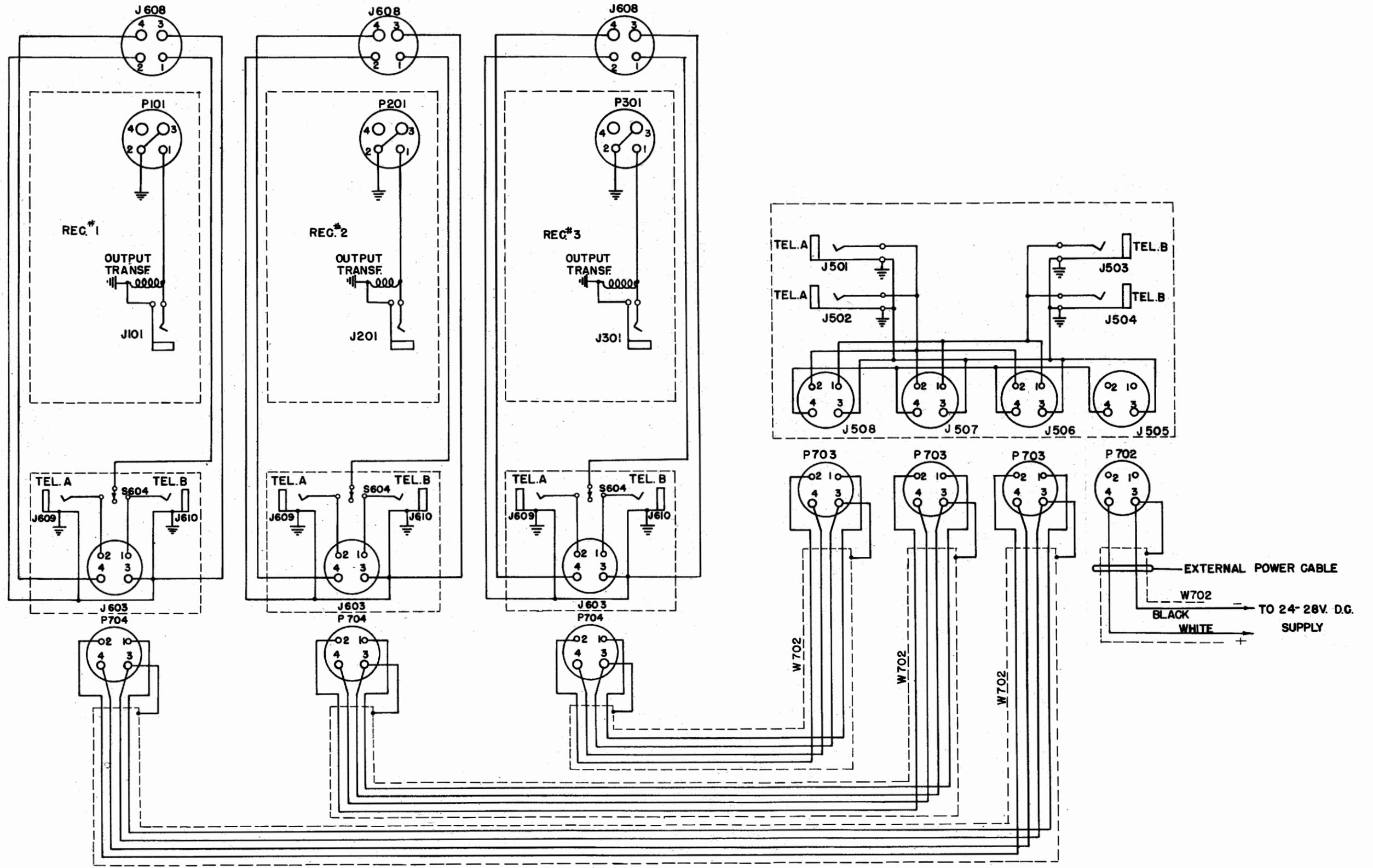
Schematic Diagram of Single Receiver Mounting and External Connections
