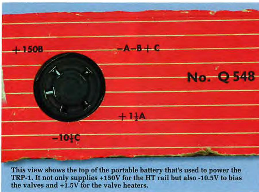
This view shows the top of the portable battery that's used to power the TRP-1. It not only supplies +150V for the HT rail but also -10.5V to bias the valves and +1.5V for the valve heaters.
