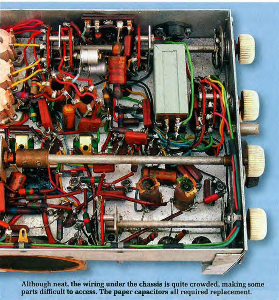
Although neat, the wiring under the chassis is quite crowded, making some parts difficult to access. The paper capacitors all required replacement.
