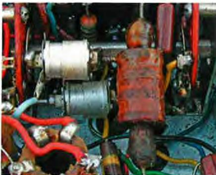
Some parts in the TRP-1 are difficult to access, particularly around the transmitter output stage.
