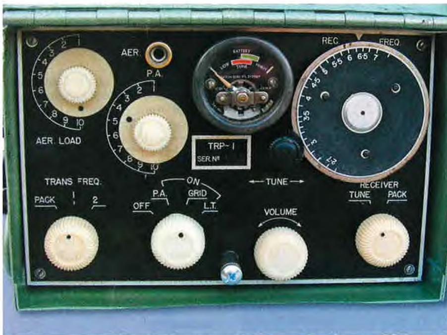
**This close-up view shows the front panel controls on the fully-restored unit. It tunes the frequency range from 2.7-7MHz and has a transmitter power output of between 1.5W and 2.3W.**
