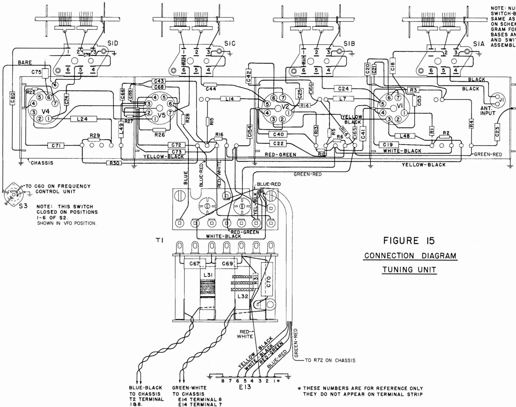
NOTE: NUMBERS ON SWITCH-BASES ARE SAME AS THOSE ON SCHEMATIC DIAGRAM FOR SWITCH BASES AND COIL AND SWITCH ASSEMBLIES.
