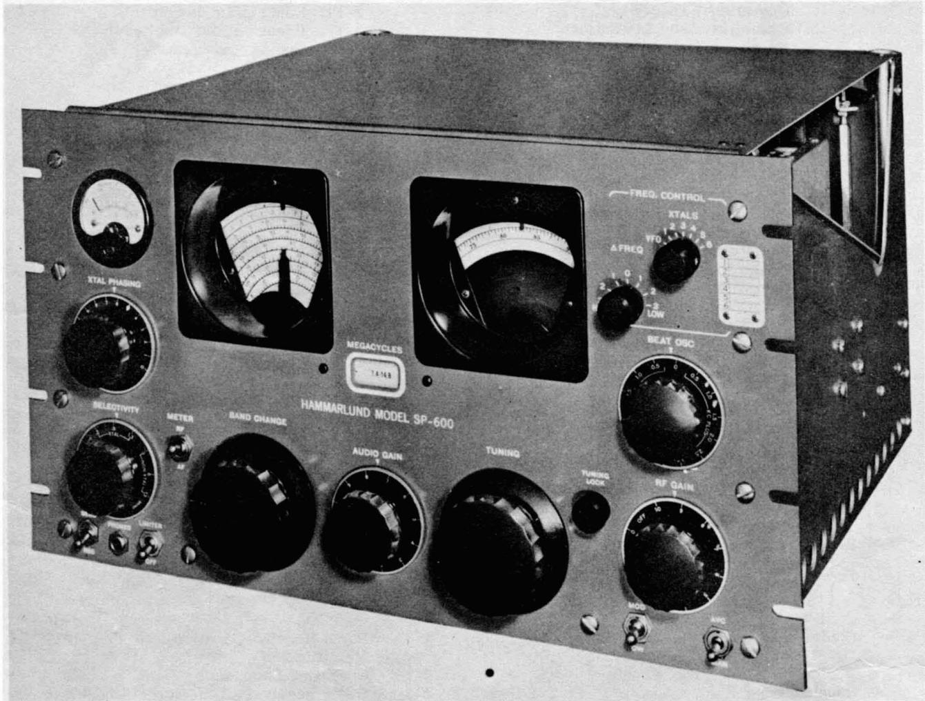
Figure 1-1. Radio Receiver, Model SP-600-JX Rack Mountings
