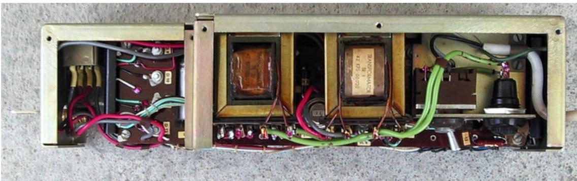
*View from the top and bottom, note Z1 on the left, new capacitors have been fitted*
