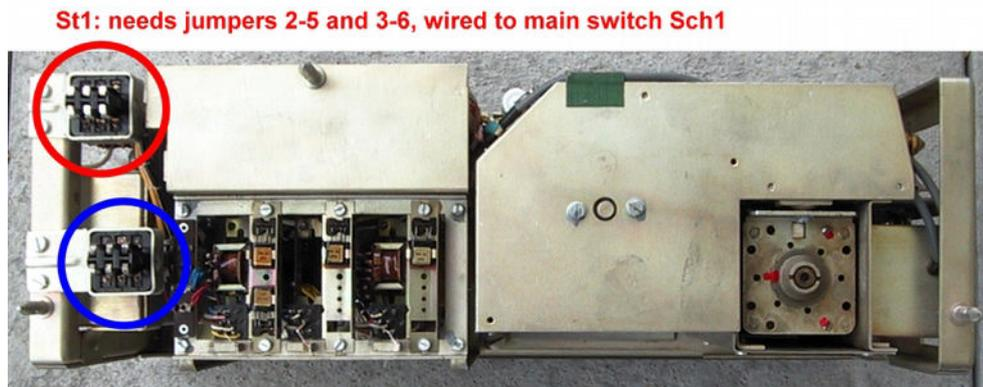
**St1: needs jumpers 2-5 and 3-6, wired to main switch Sch1**
