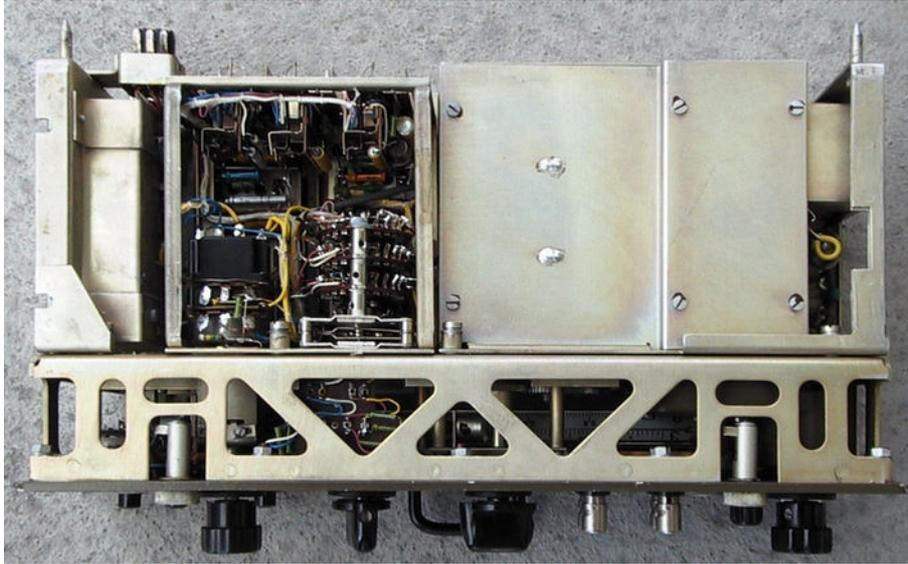
*Bottom view, audio circuits and mode and power switches on the left*
