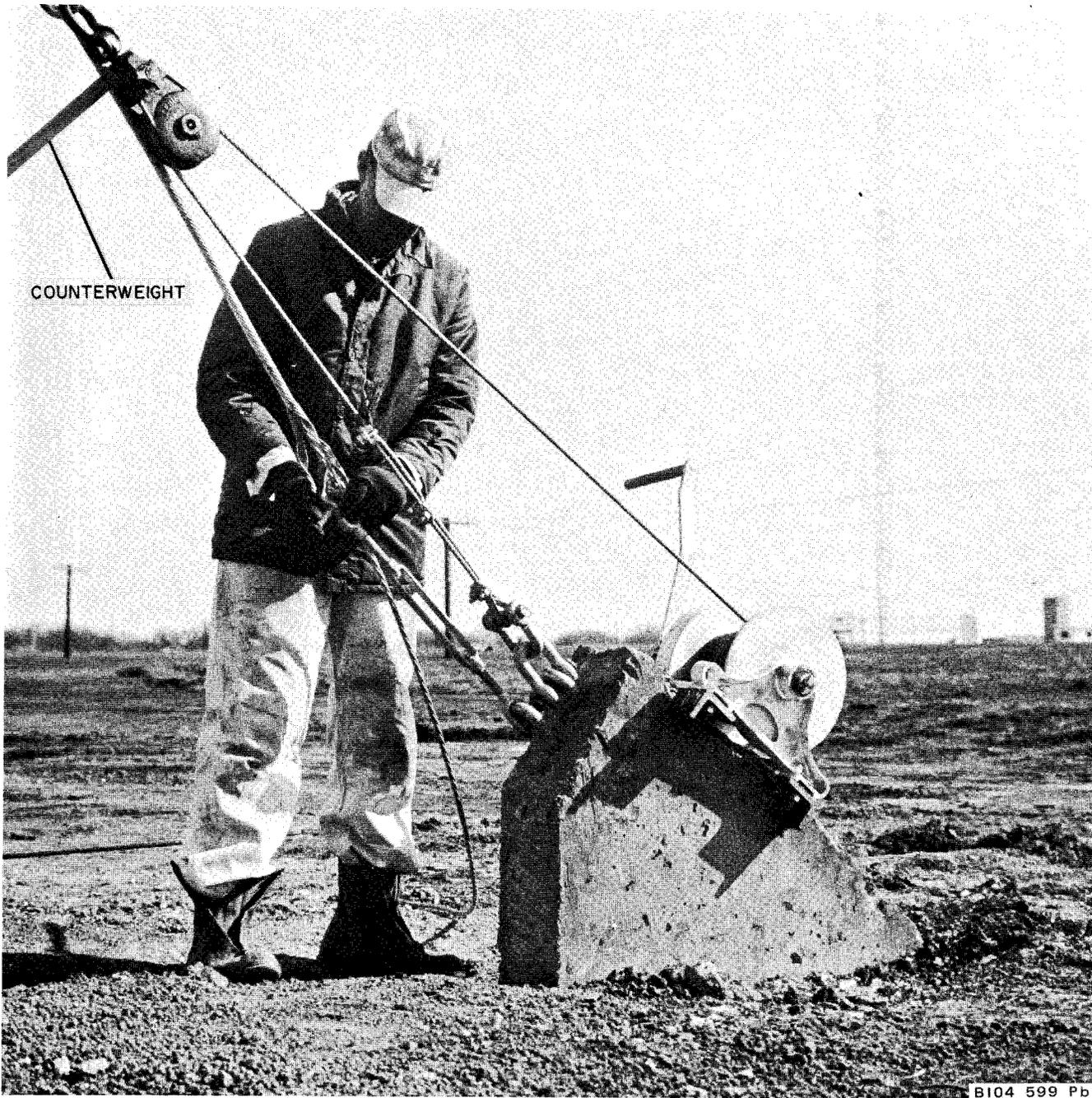
Figure 2-14. Winch and Block Assembly in Use.
