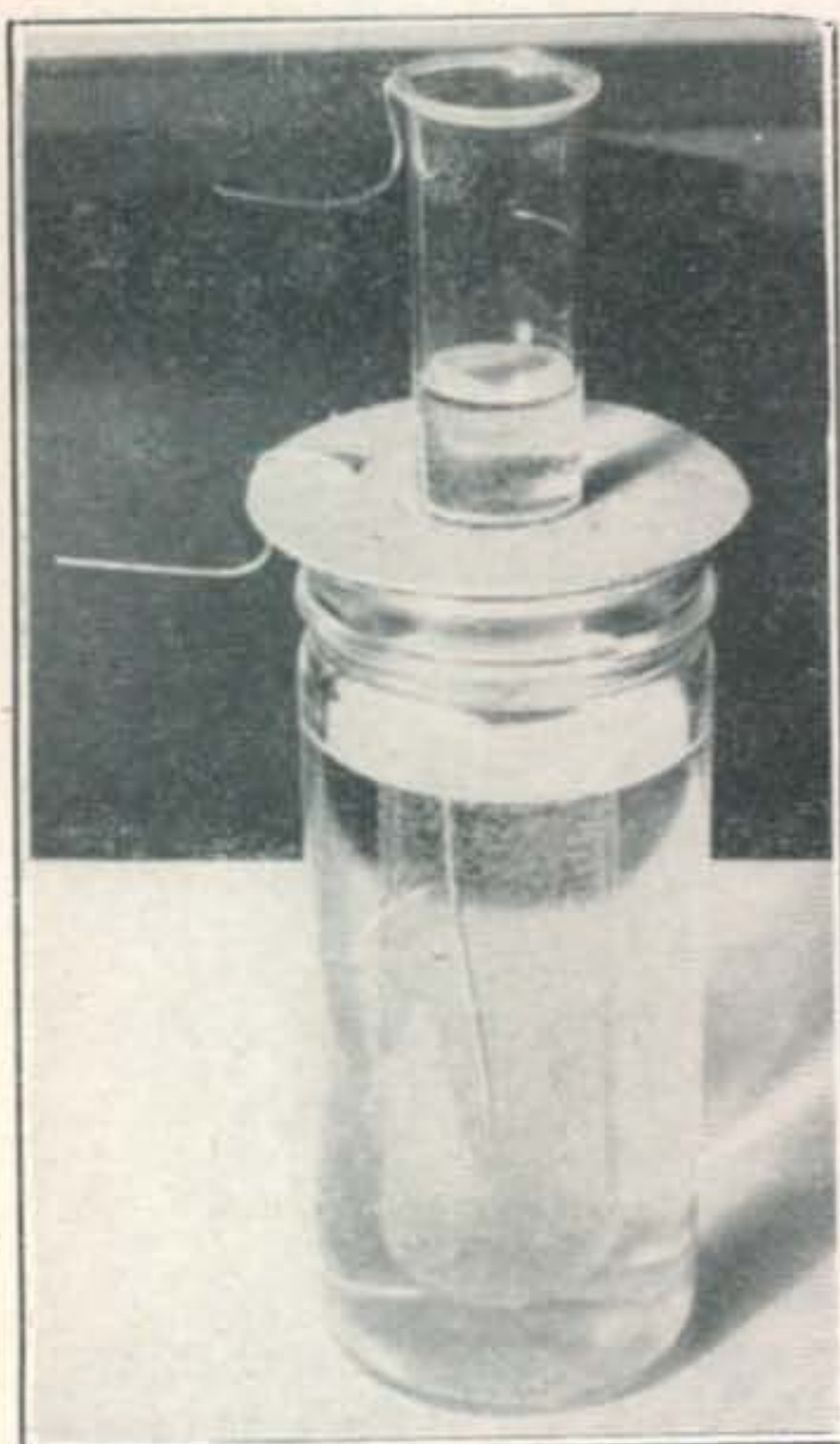
The water capacitor consists of two glass containers, one suspended inside the other, both filled with water. Bare wire leads immersed in the solution of each container act as the conductors.
