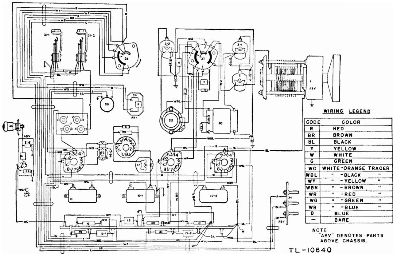
Figure 89. Frequency Meter BC-221-AE, chassis wiring diagram.
