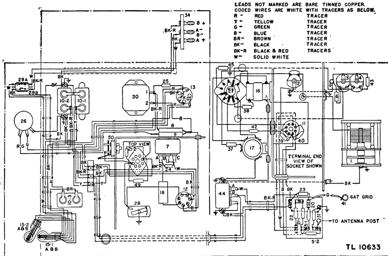
Figure 55. Frequency Meter BC-221-(3), chassis wiring diagram.
