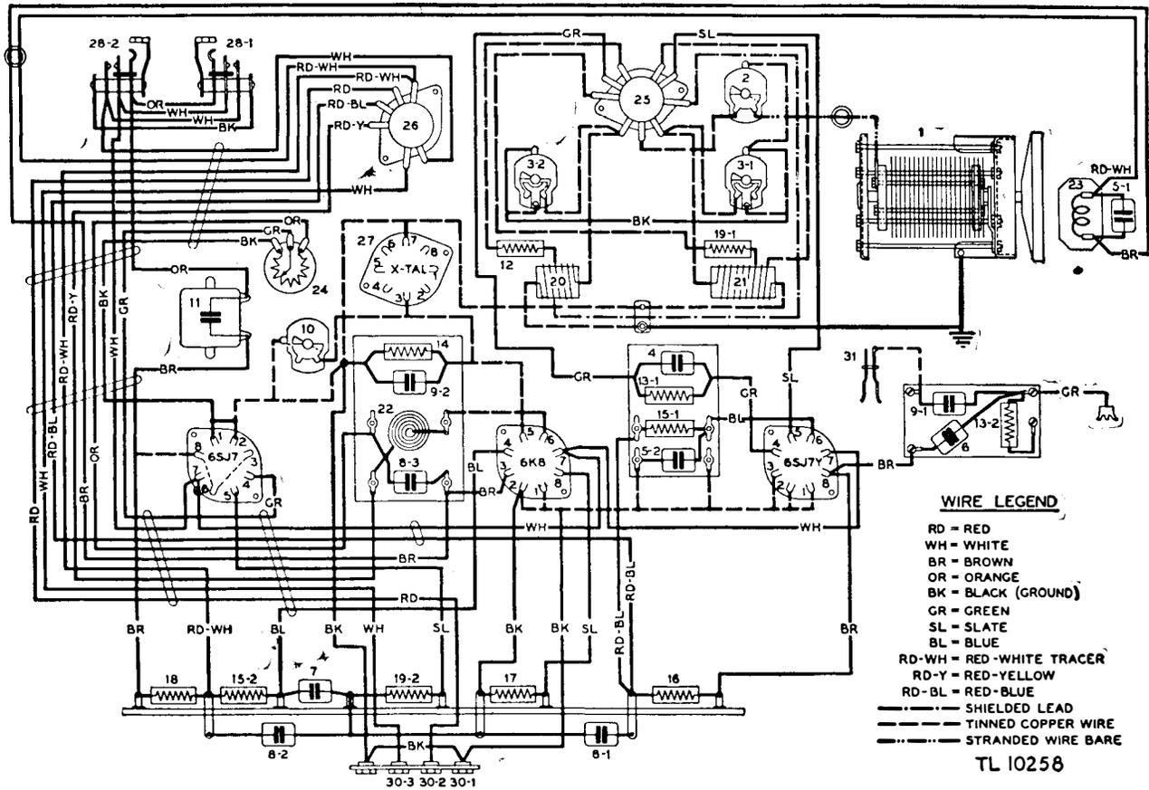
Figure 45. Frequency Meter BC-221-Q, chassis wiring diagram.
