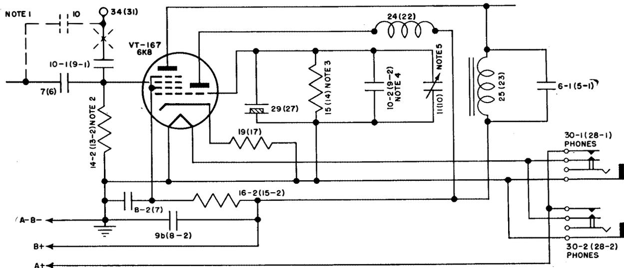
NOTE 1:-- CONNECTION SHOWN DASHED AND OPEN CIRCUIT SHOWN  $\times$  APPLIES TO EARLY MODEL OF BC-221-B
