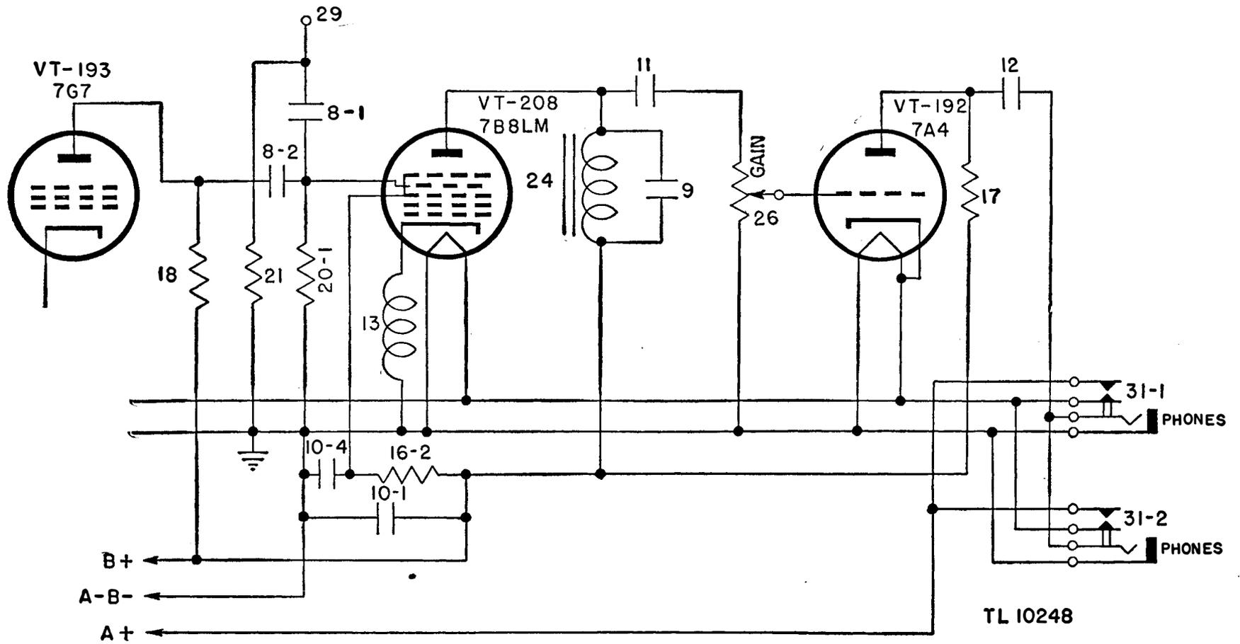
Figure 4B. Frequency Meter BC-221-E, functional diagram, detector and audio-amplifier circuits.
