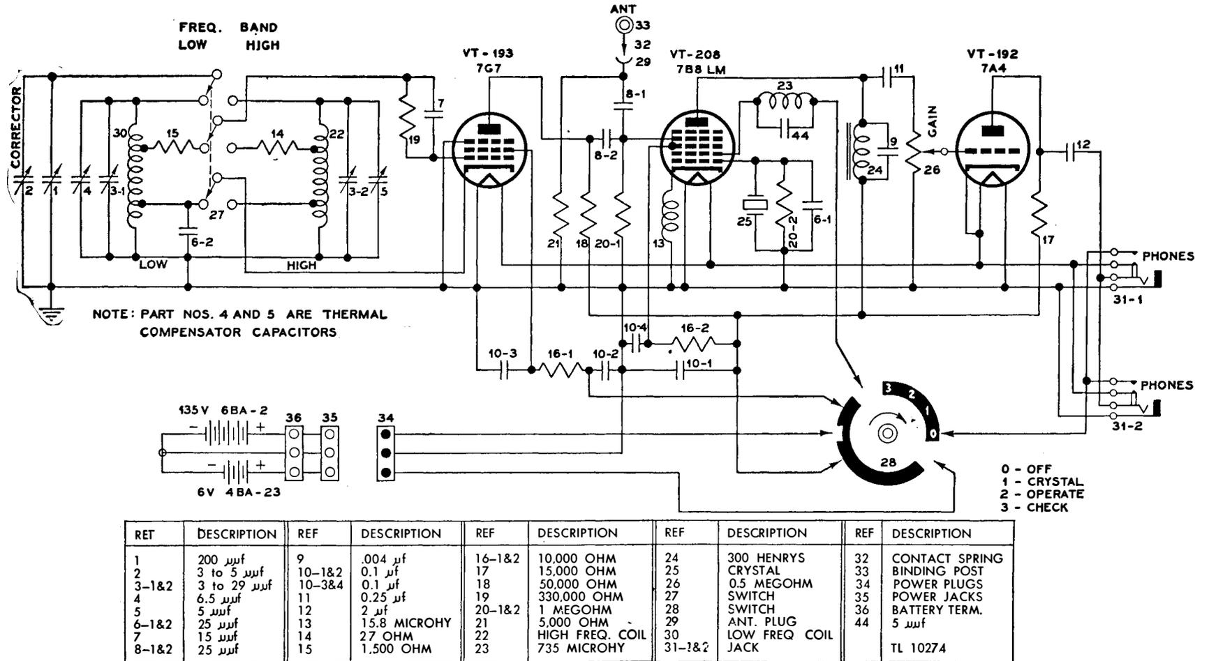
Figure 49. Frequency Meter BC-221-E, schematic diagram.
