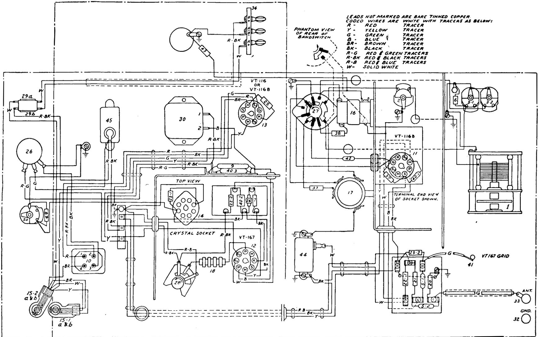
Figure 82. Frequency Meter BC-221-AF, chassis wiring diagram.
