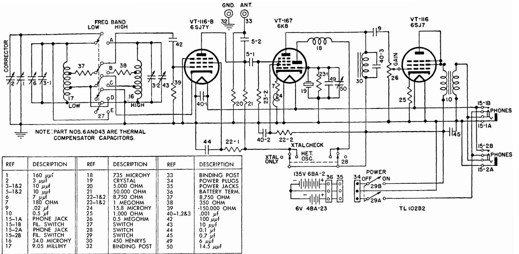
Figure 79. Frequency Meter BC-221-AF, schematic diagram.
