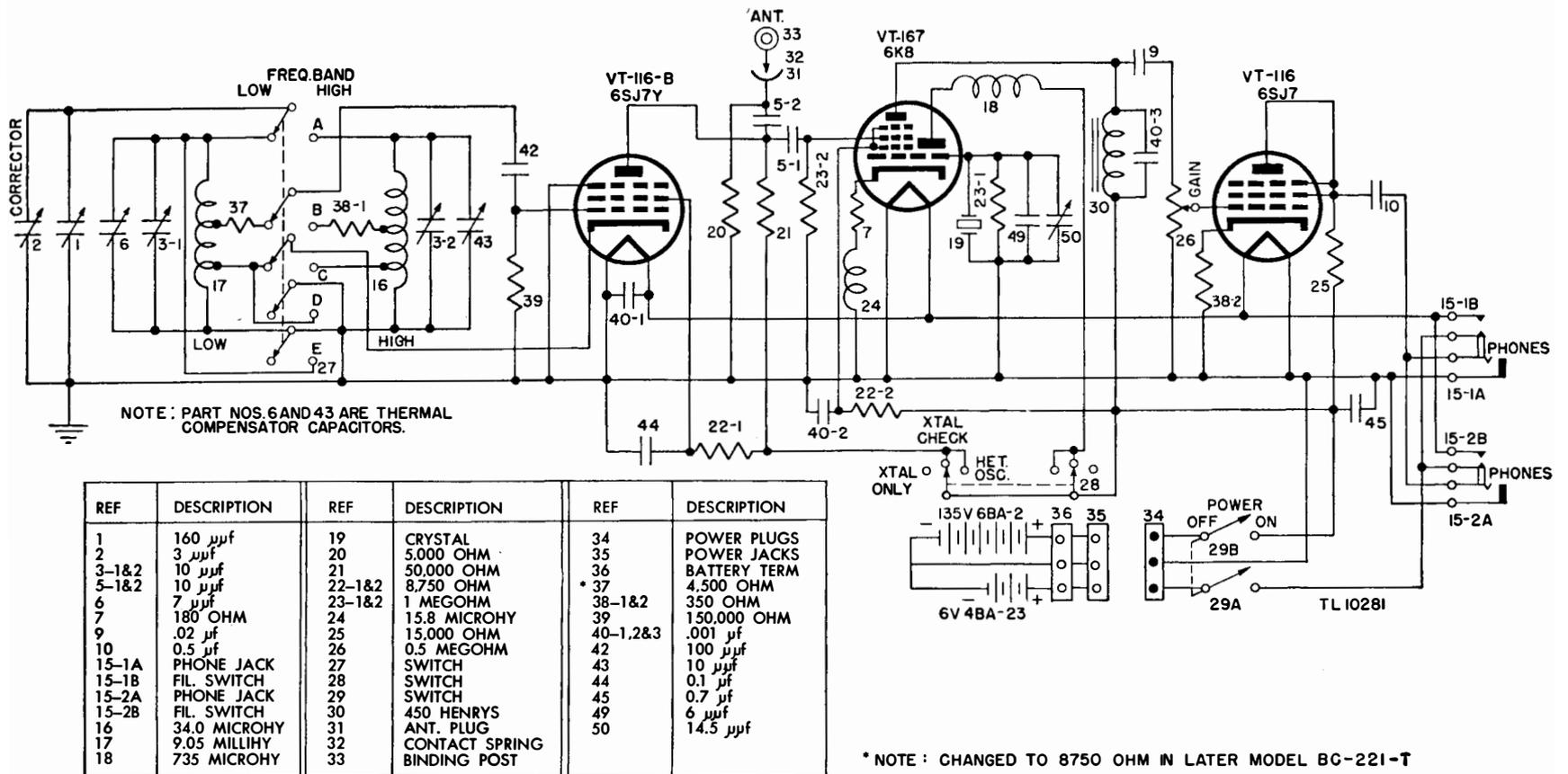
Figure 78. Frequency Meters BC-221-P and BC-221-T, schematic diagram.
