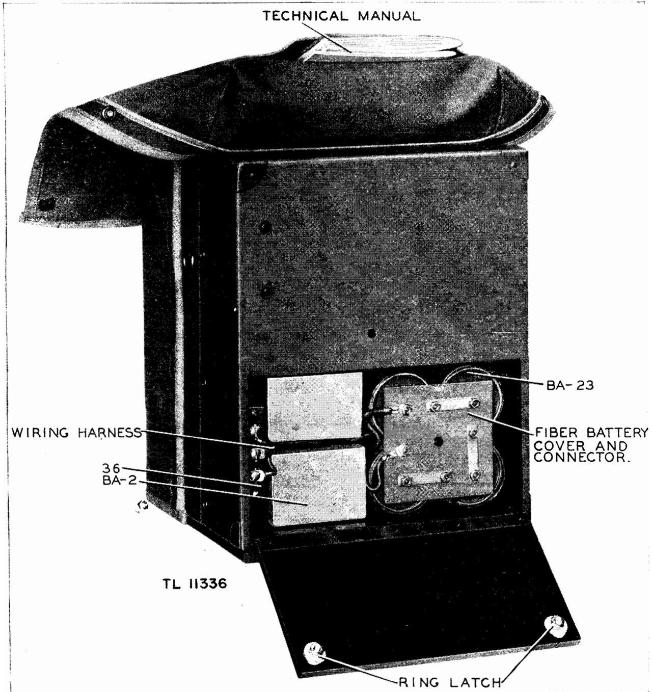
Figure 67. Frequency Meter BC-221-(G), wooden cabinet, battery installation.
