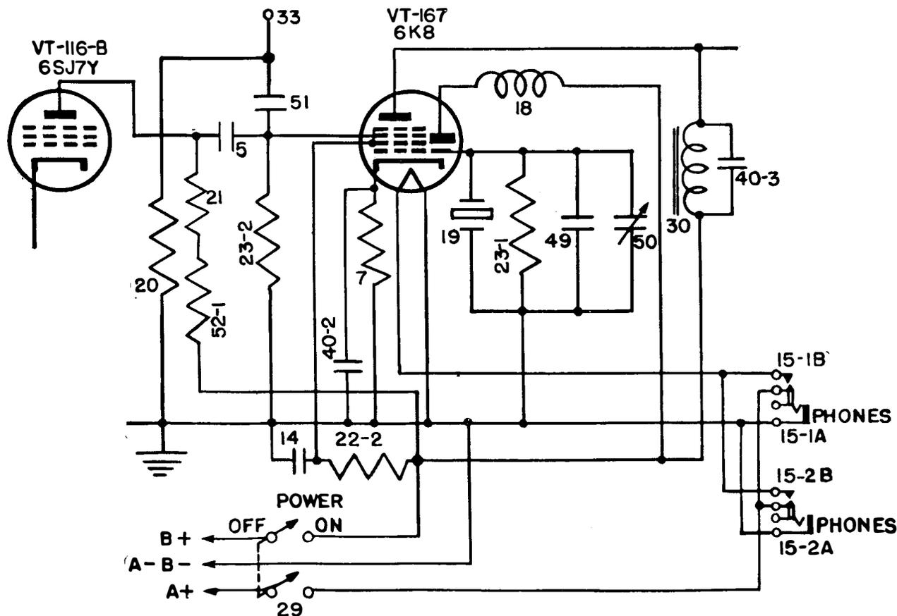
Figure 96. Frequency Meter BC-221-(8), functional diagram, crystal-oscillator circuit.
