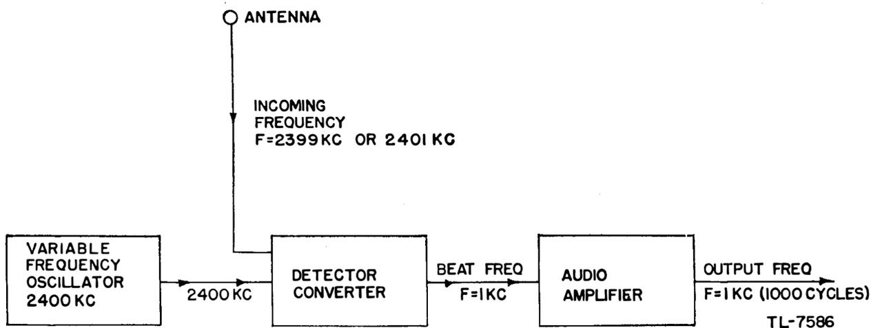
Figure 18. Block diagram, measurement of an external signal.
