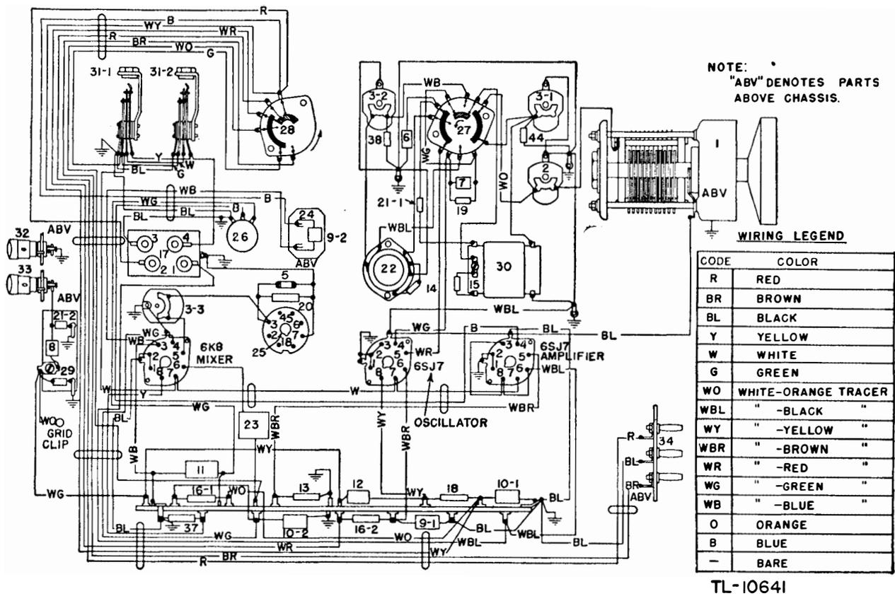
Figure 90. Frequency Meter BC-221-AG, chassis wiring diagram.
