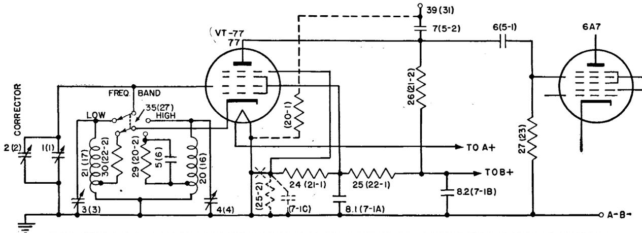
NOTE: - ITEMS SHOWN IN DASHED LINES ARE INCLUDED IN BC-221-C AND BC-221-D ONLY. THE CONNECTION AT JUNCTION OF PARTS (25-2) AND 24(21-1) TO GROUND, SHOWN  $\times$  INDICATES AN OPEN CIRCUIT ON THE BC-221-C AND BC-221-D.
