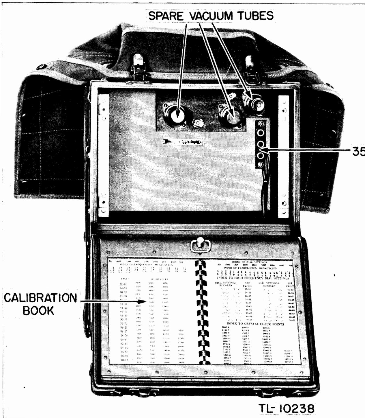
Figure 21. Frequency Meter BC-221-AF, view of cabinet interior and calibration book.
