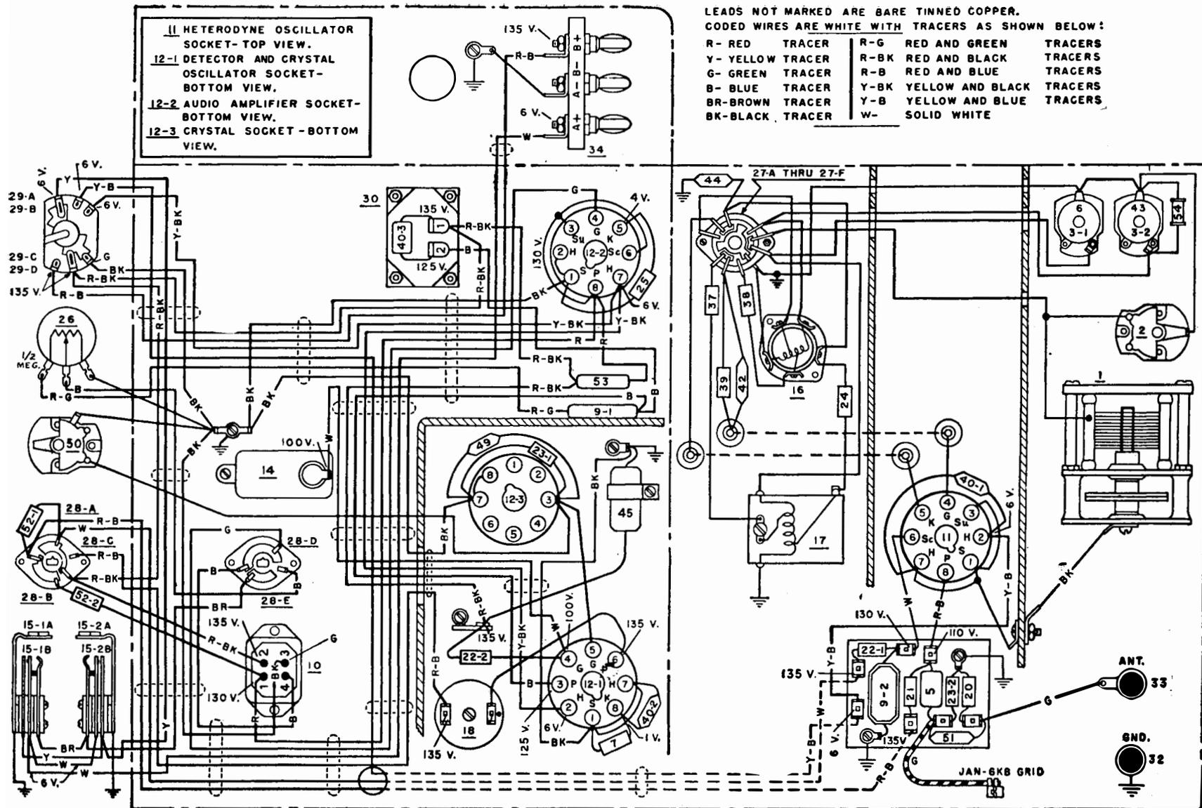
Figure 101. Frequency Meter BC-221-Aj, chassis wiring diagram.
