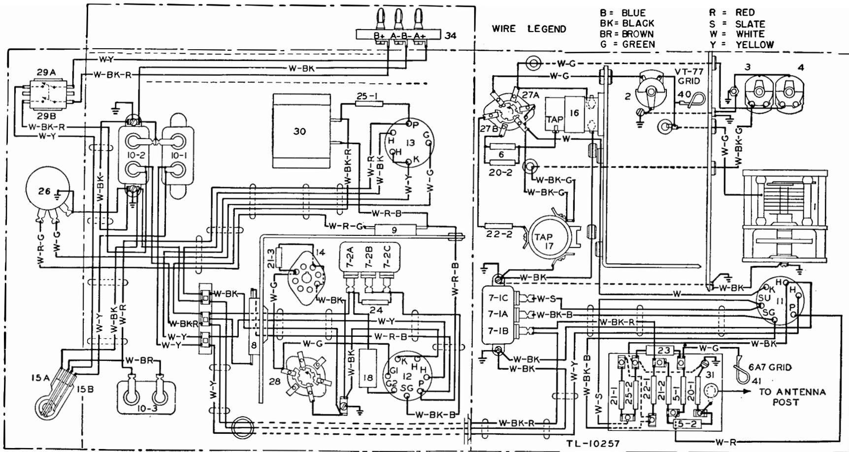
Figure 34. Frequency Meters BC-221-C and BC-221-D, chassis wiring diagram.
