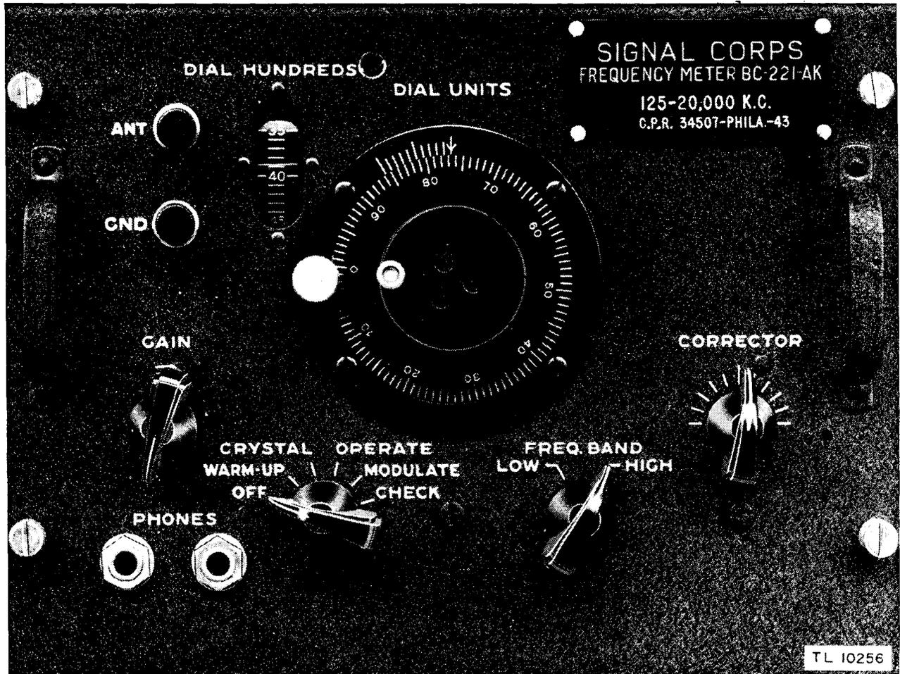
Figure 8. Frequency Meter BC-221-AK, control panel lay-out.
