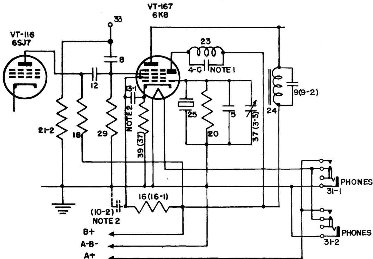
NOTE 1:- THE BY-PASS CAPACITOR, PART NO. 4-C, IS OMITTED IN THE BC-221-AG.
