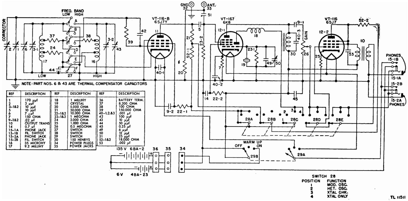
Figure 100. Frequency Meter BC-221-AL, schematic diagram.
