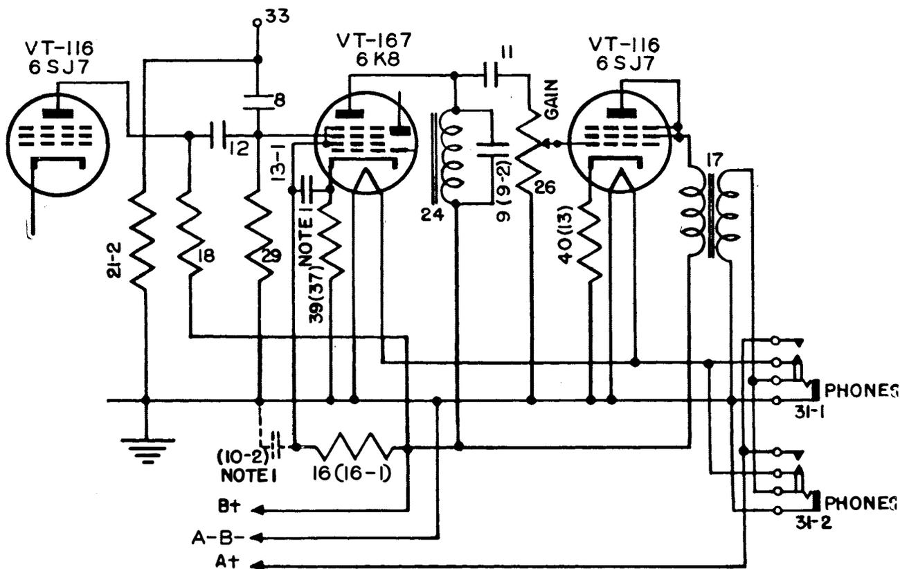
NOTE 1: PART NO. 13-1 IS OMITTED & REPLACED BY PART NO.(10-2) SHOWN IN DASHED LINES, IN THE BC-221-AG.
