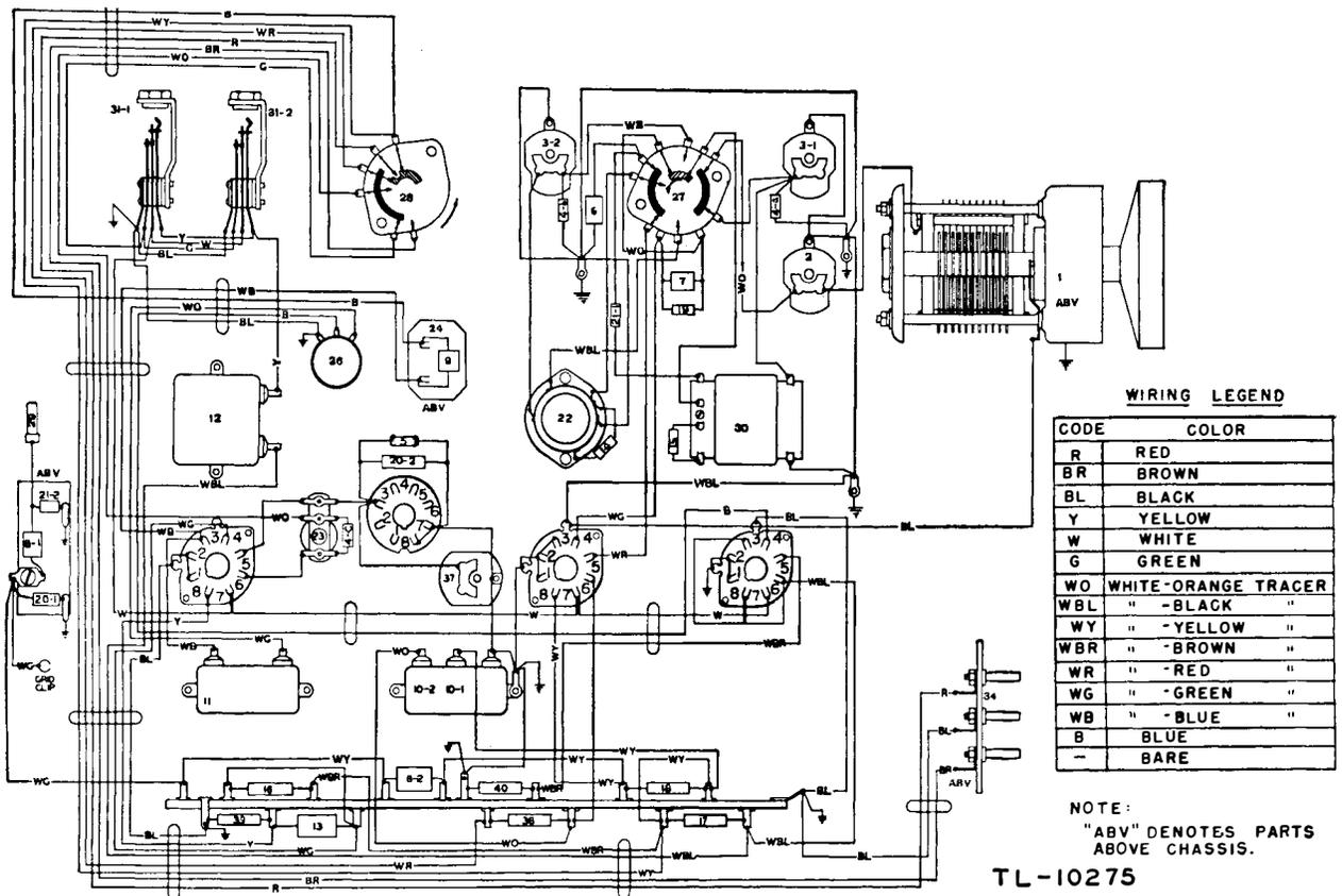
Figure 72. Frequency Meter BC-221-N, chassis wiring diagram.
