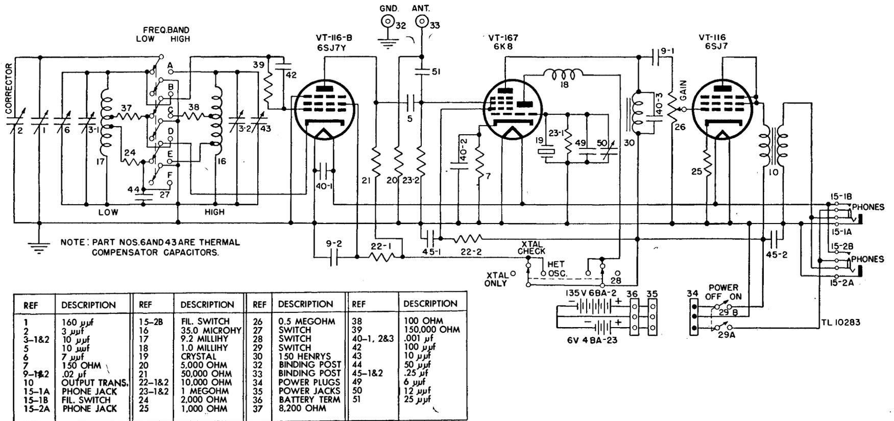
Figure 80. Frequency Meter BC-221-AH, schematic diagram.
