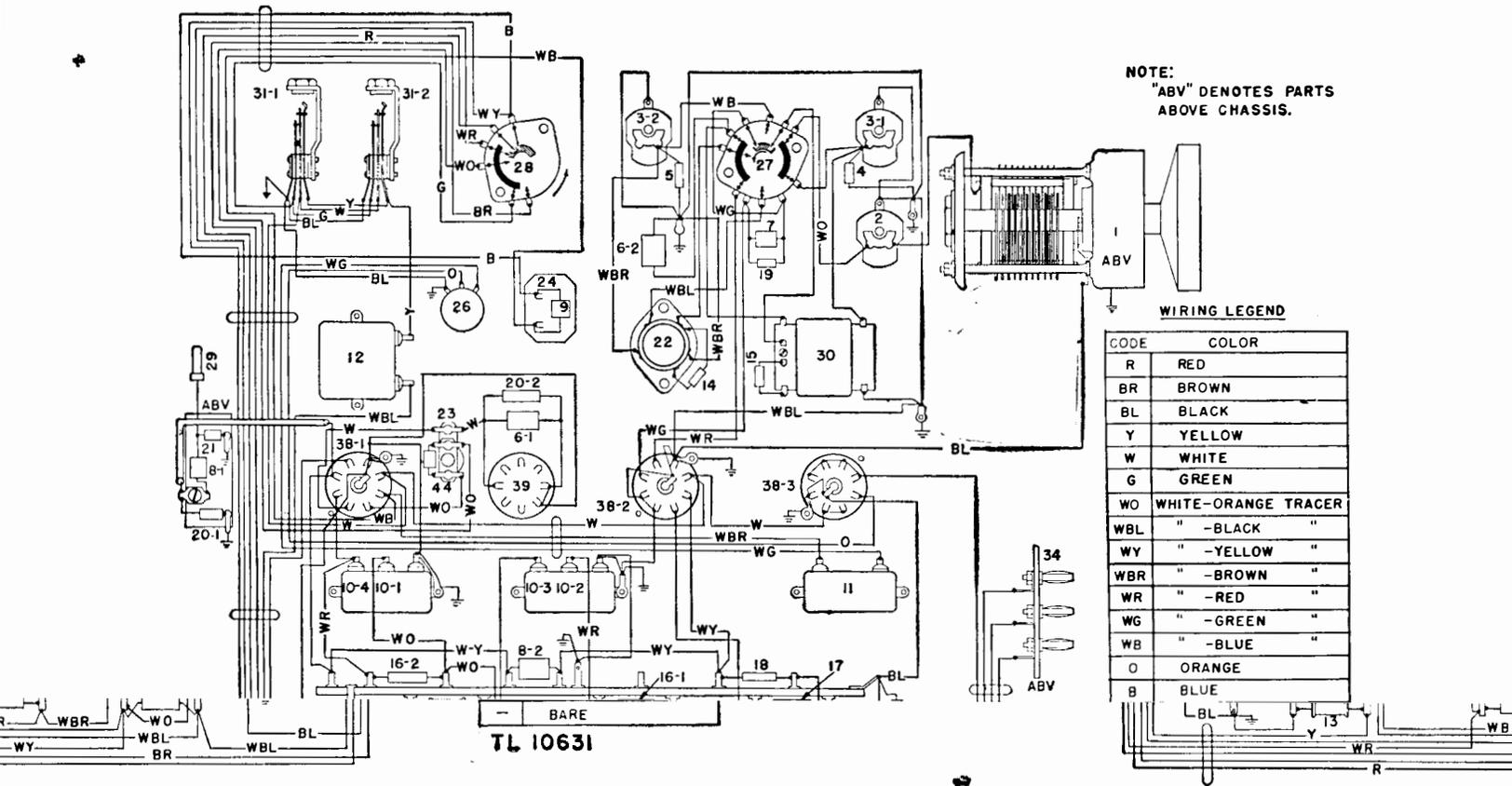
Frequency Meter BC-221-E, chassis wiring diagram.
