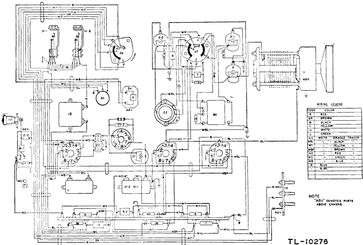
Figure 73. Frequency Meter BC-221-AA, chassis wiring diagram.
