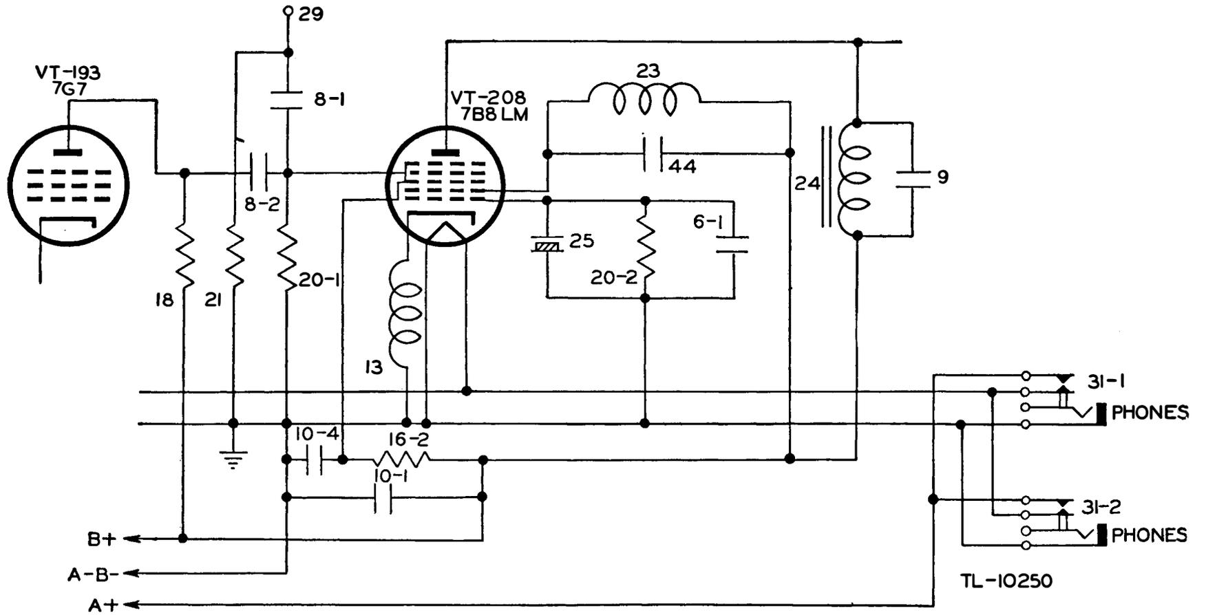
Figure 46. Frequency Meter BC-221-E, functional diagram, crystal-oscillator circuit.
