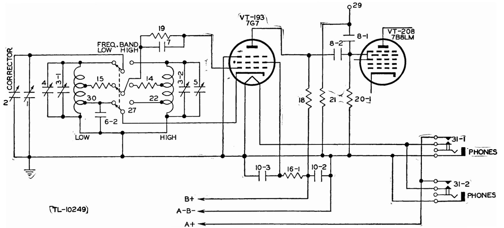
Figure 47. Frequency Meter BC-221-E, functional diagram, variable frequency oscillator circuit.
