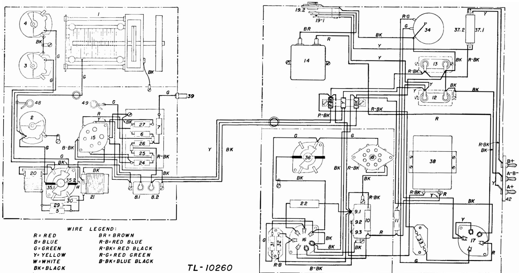
Figure 33. Frequency Meter BC-221-A, chassis wiring diagram.
