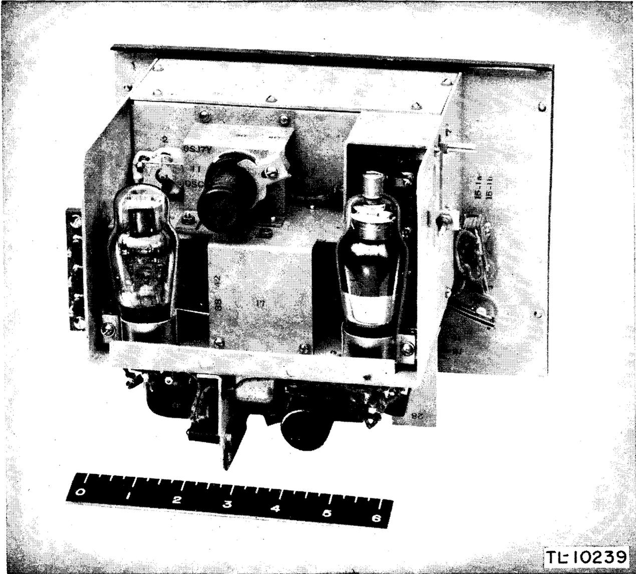
Figure 22. Frequency Meter BC-221-F, rear view of chassis.
