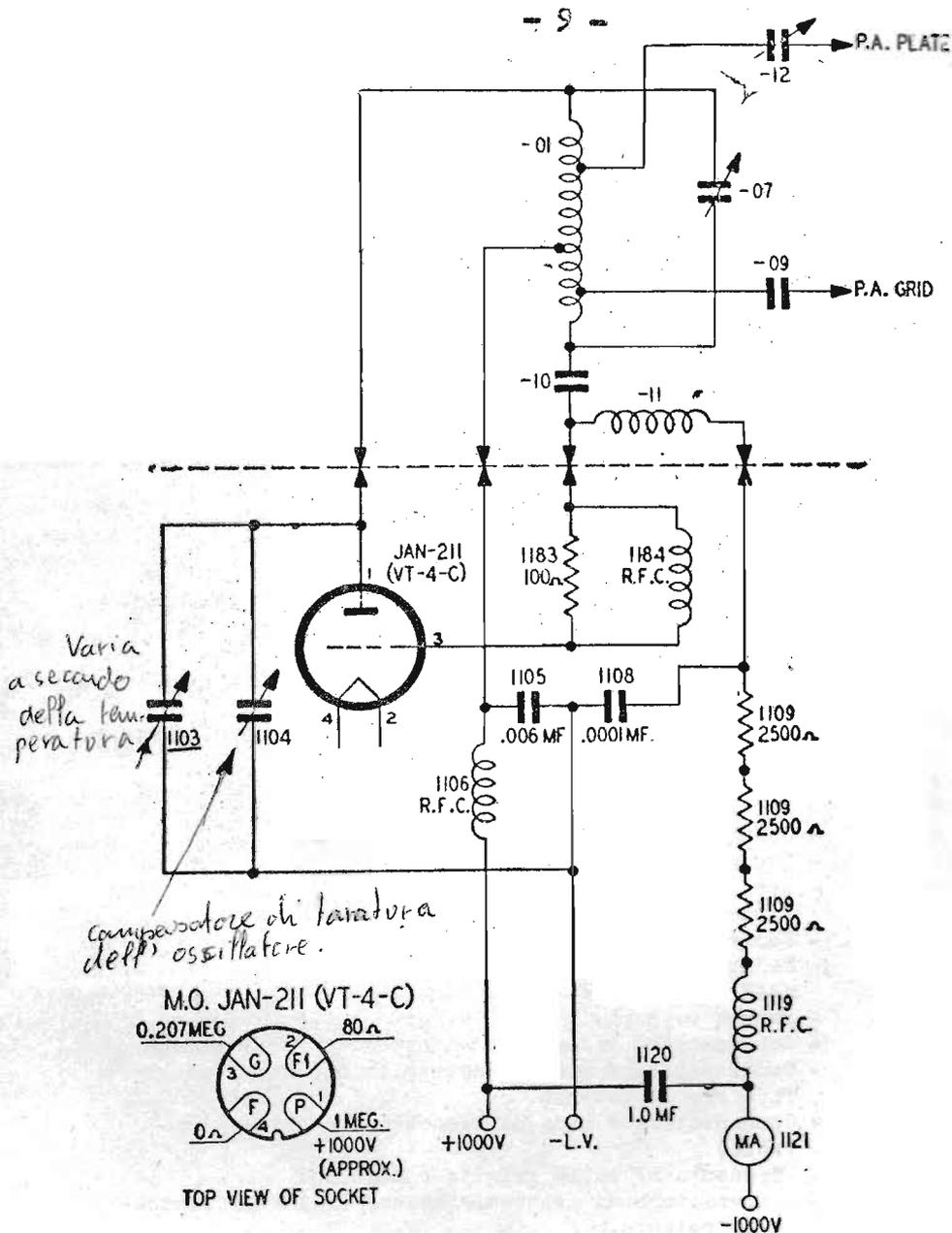
NOTE:—CIRCUIT ABOVE DOTTED LINE IS IN TUNING UNIT; THAT BELOW DOTTED LINE IS IN TRANSMITTER.
