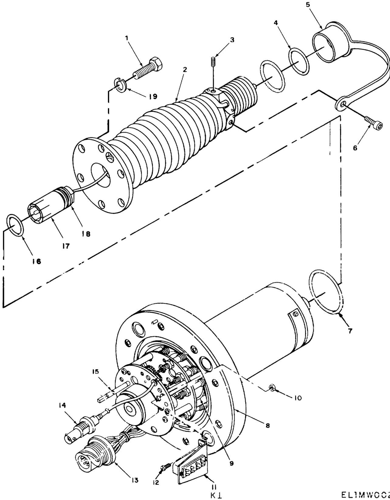
FIGURE 2. MATCHING UNIT BASE, ANTENNA MX-6707/VRC (SHEET 1 OF 2).
