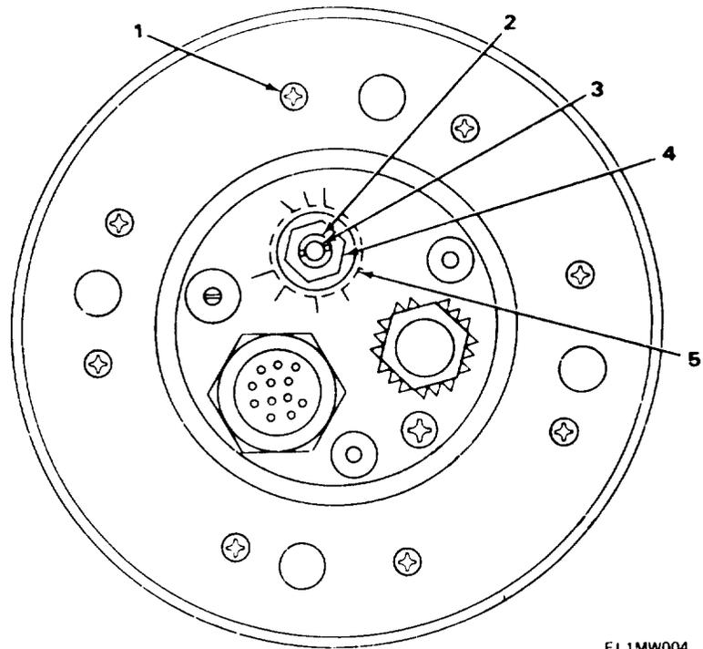
FIGURE 3. MATCHING UNIT BASE, ANTENNA MX-6707/VRC, BOTTOM VIEW, EXTERIOR AND INTERIOR.
