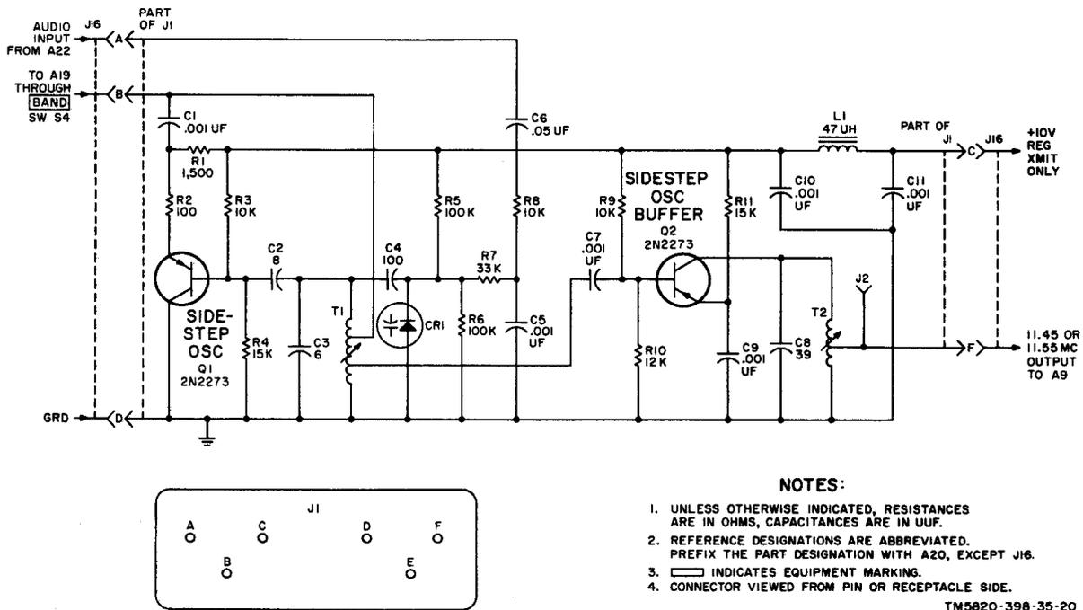
Figure 8. Sidestep oscillator module A20, schematic diagram.
