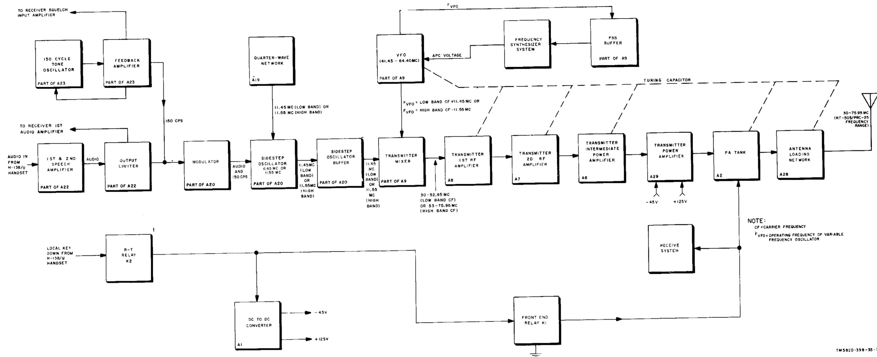
Figure 83. Receiver-transmitter block diagram, transmitted signal paths.
