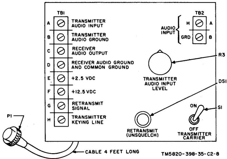
Figure 79.6. Test assembly, schematic/wiring diagram.
