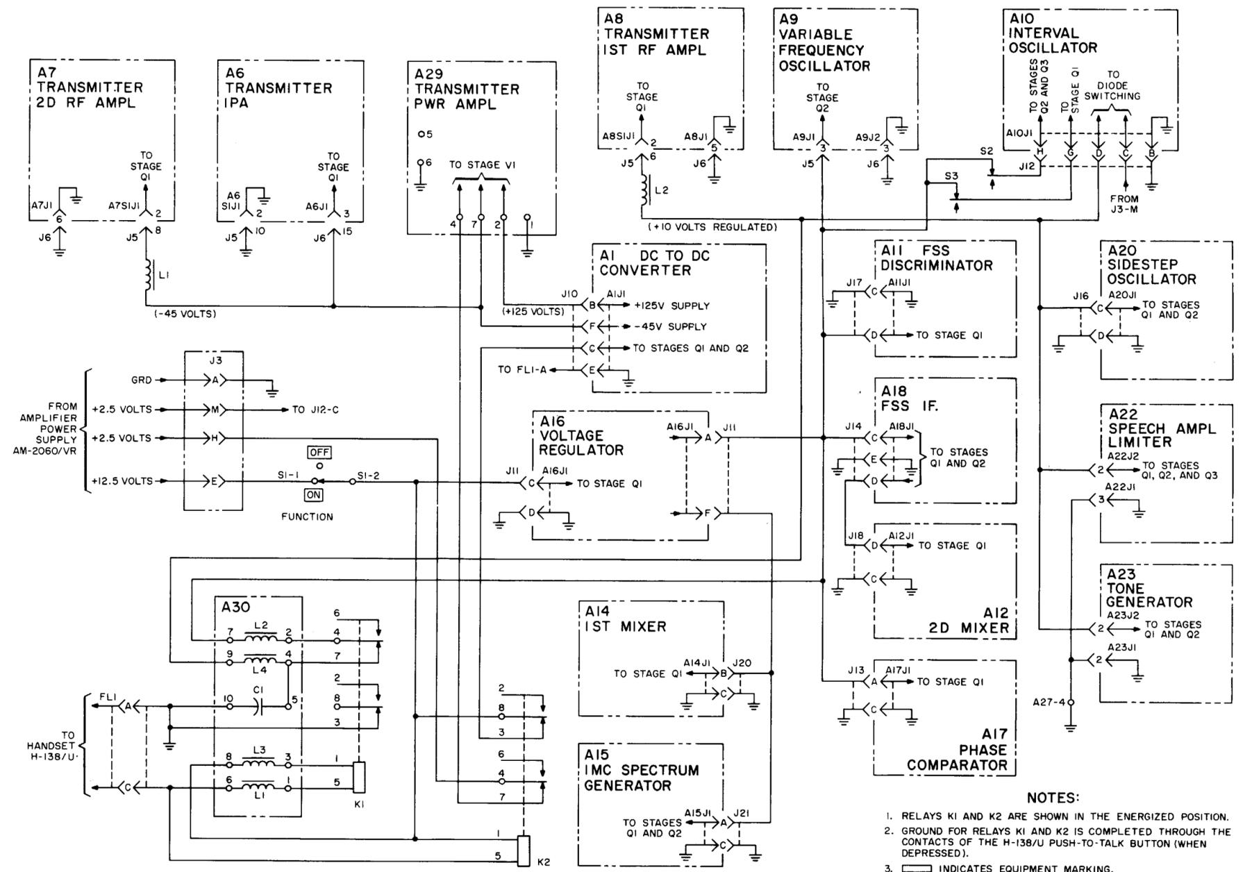
Figure 87. Power distribution, transmit condition, simplified schematic diagram.
