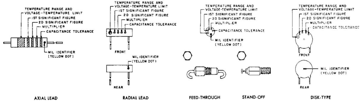
GROUP III Capacitors, Fixed, Ceramic-Dielectric (Temperature Compensating) Style CC
