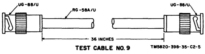
Figure 79.3. Test cables No. 7, No. 8, and No. 9.
