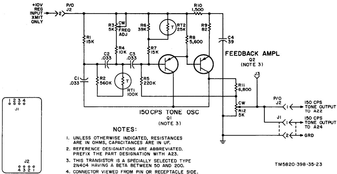
Figure 7. Tone generator module A23, schematic diagram.
