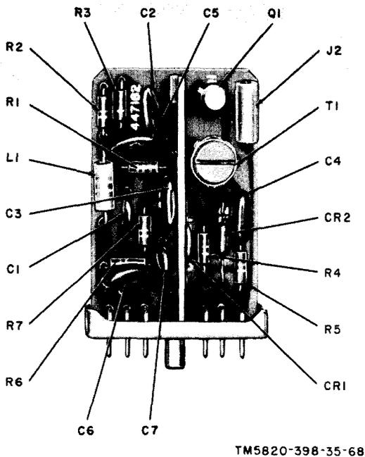
Figure 69. Module A17, parts location
