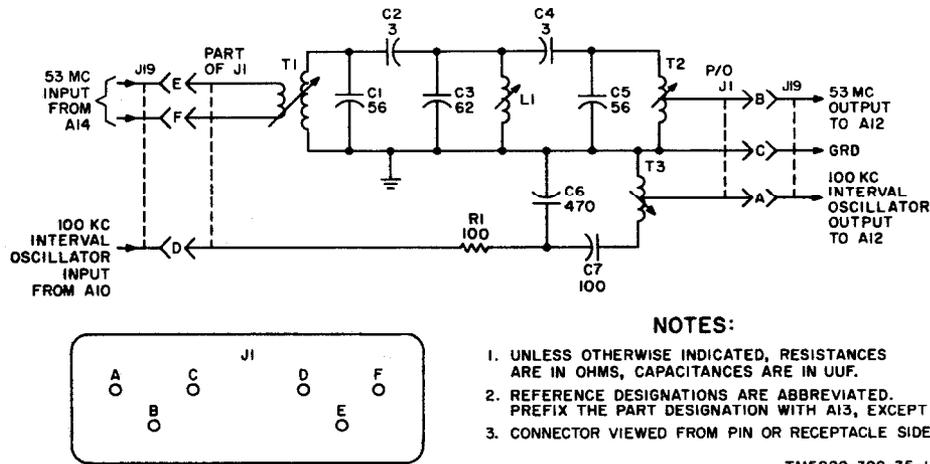
Figure 20. 53-Mc filter module A 13, schematic diagram
