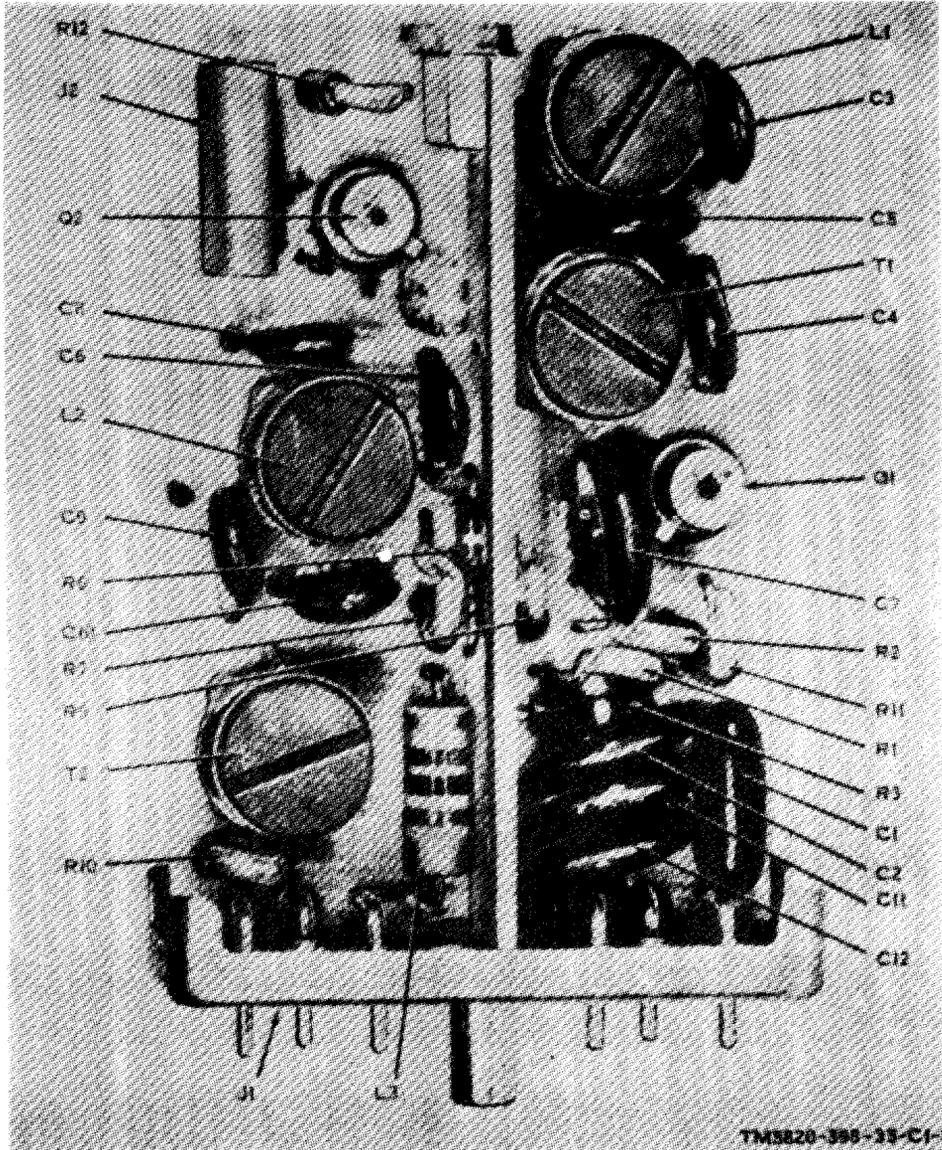
*Figure 70.1. Module A18, late model, parts location.*
