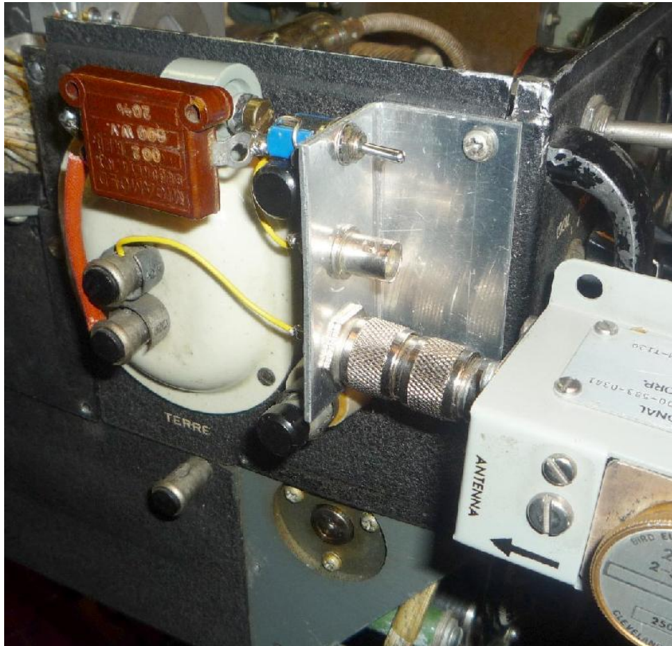
Figure 4.1 – ART-13 RF Connections
