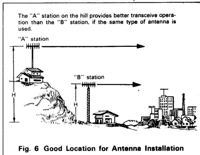
Fig. 6 Good Location for Antenna Installation
