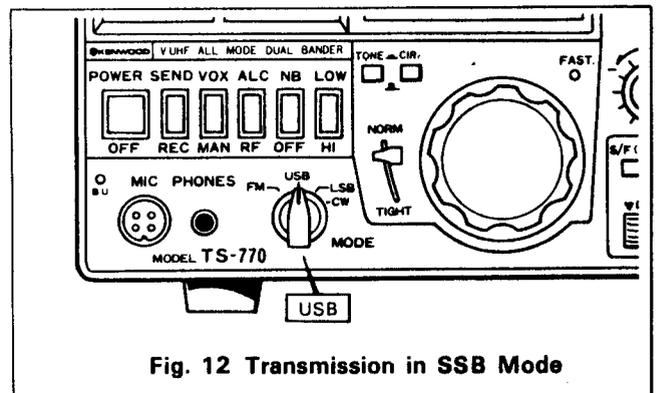
Fig. 12 Transmission in SSB Mode
