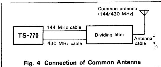
Fig. 4 Connection of Common Antenna
