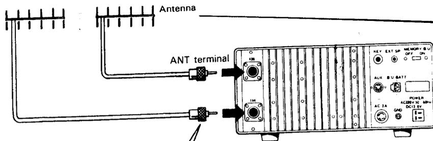
A. Mounting the UHF type connector
