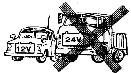
For mobile operation, connect the unit to a 12V car battery (6A). Do not connect it to a 24V battery.
