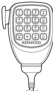
Each time you press the desired key, the Commander will automatically enter transmit mode and send the corresponding control command to the Transporter.
