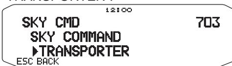
Now the Commander and Transporter are in Sky Command mode. For operations in this mode, see "CONTROL OPERATION". First switch ON the HF transceiver and press [SYNC] on the Commander. To exit the Sky Command mode, access Menu 703 and select "OFF".
