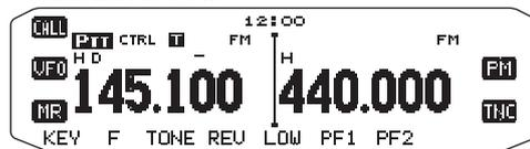
**Note:** When accessing a repeater that requires a 1750 Hz tone, you do not need to activate the Tone function. Simply press the key assigned to the 1750 Hz tone {Menu 507 ~ 512} to transmit the tone.
