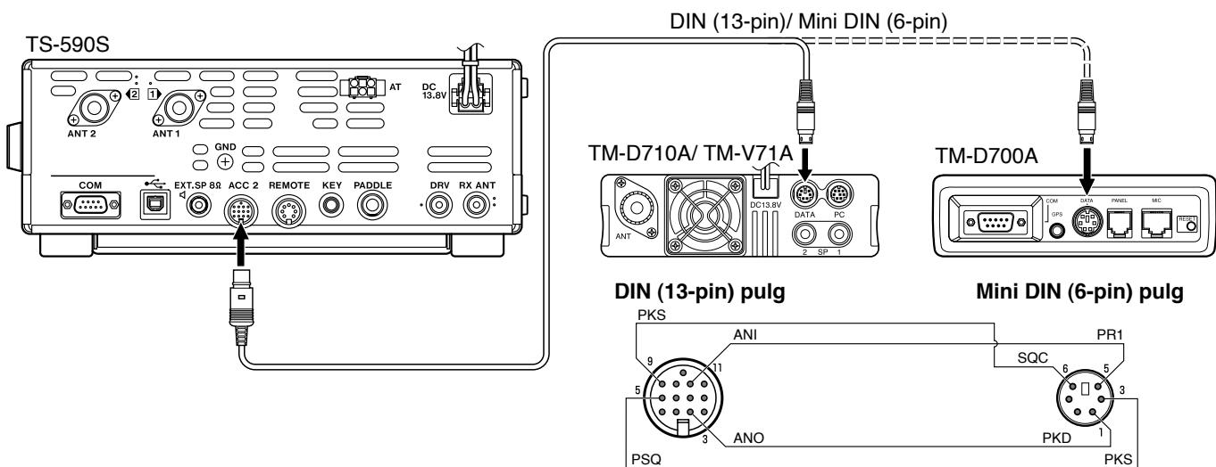
After connecting the 2 transceivers with the cable, access Menu Nos. 73 (PKS polarity) and 74 (Busy lockout) on the TS-590S transceiver and select "on". You will further need to adjust the audio input/ output level of the TS-590S transceiver using Menu Nos. 66 and 67.
