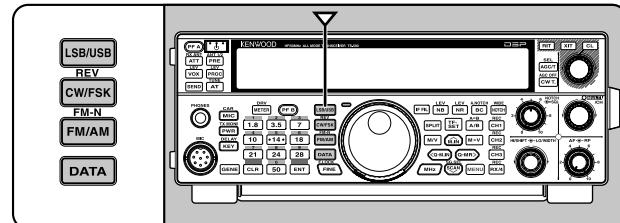
Access Menu No. 23 then press [M.IN] to select "on" to turn the Auto Mode selection ON. When it is ON, "AUTO" appears. As a default, if you change the frequency above or below 9.5 MHz, the transceiver automatically switches modes; LSB for frequencies under 9.5 MHz and USB for frequencies 9.5 MHz and over. You can further add the frequency borders to the Auto Mode selection {page 51}.
