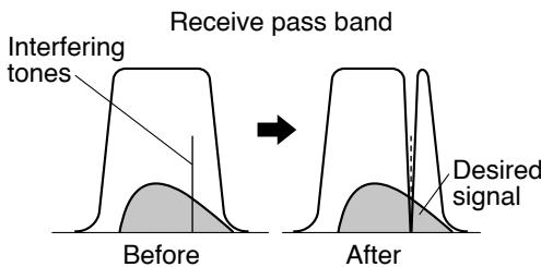
Press and hold [BC (A.NOTCH)] to toggle the Auto Notch Filter ON and OFF.
