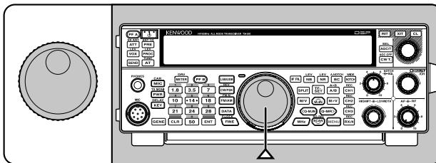
You may prefer directly entering a frequency using the numeric keypad if the desired frequency is far from the current frequency. Press [**ENT**], then press the numeric keys as necessary. For details, refer to "Direct Frequency Entry" {page 28}.
