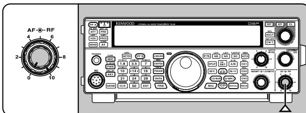
**Note:** The position of the AF control does not affect the volume of beeps caused by pressing keys nor the CW TX sidetone. The audio level for Digital mode operation is also independent of the AF control setting.
