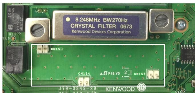
Fig. 16 Additional Roofing Filter Mounting Slot
