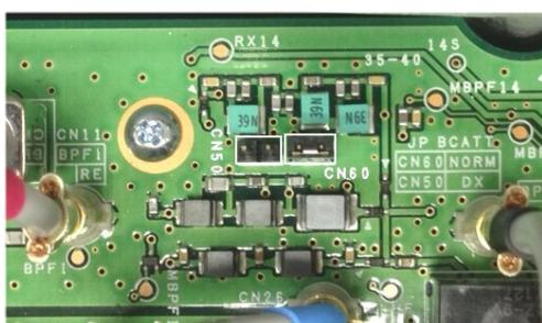
Fig. 24 Main Band Jumper Pin Locations
