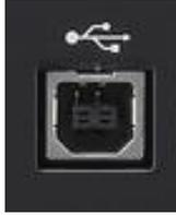
Fig. 144 USB Connector (on the Rear Panel)
