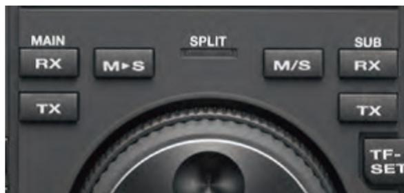
Fig. 101 Key Allocation Suitable for Split Operation
