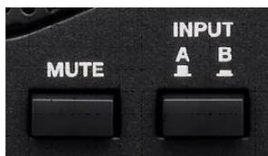
Fig. 21 Input Select Switch (A/B) (on the Front Panel)
