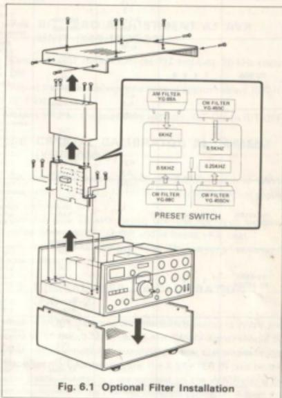
Fig. 6.1 Optional Filter Installation
