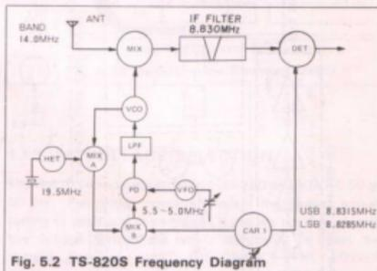
Fig. 5.2 TS-820S Frequency Diagram
