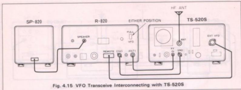
Fig. 4.15 VFO Transceiver Interconnecting with TS-520S
