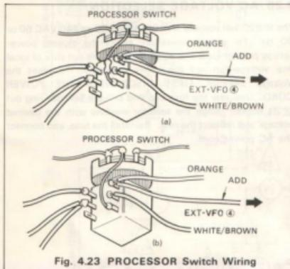
Fig. 4.23 PROCESSOR Switch Wiring
