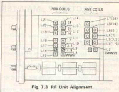
Fig. 7.3 RF Unit Alignment
