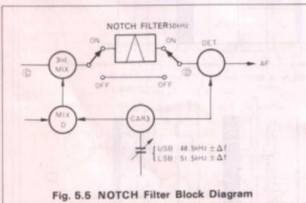
Fig. 5.5 NOTCH Filter Block Diagram
