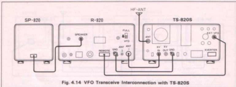
Fig. 4.14 VFO Transceiver Interconnection with TS-820S
