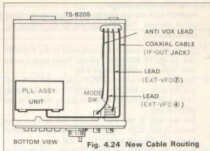
Fig. 4.24 New Cable Routing
