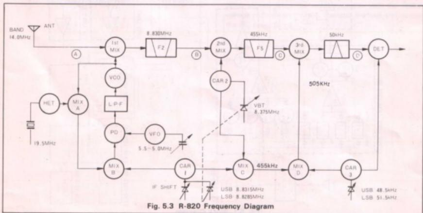
Fig. 5.3 R-820 Frequency Diagram
