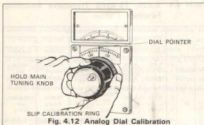
Fig. 4.12 Analog Dial Calibration
