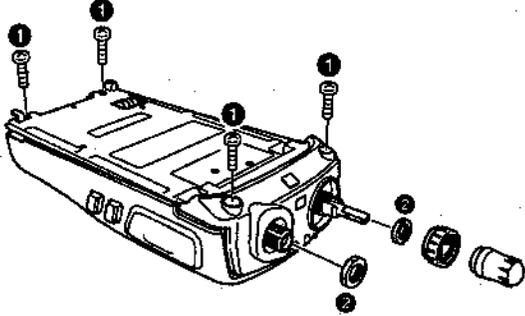
2. Pull out the panel assembly (●) and separate the chassis from the case gradually, beginning with the bottom (●). Finally, remove the waterproof seal rubber (●) from the groove, being careful not to break the rubber.
