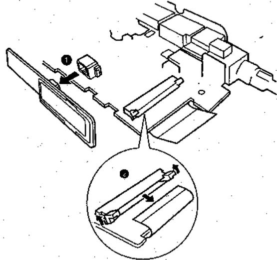
2. Release the four hooks (●) on the right guide from the control PC board. The right guide and LCD assembly (●) will be detached.
