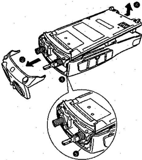
3. The main body is divided into two blocks: a case and a chassis. However, they are connected with a flat cable. The TH-D7A/E can be turned on, checked and adjusted.
