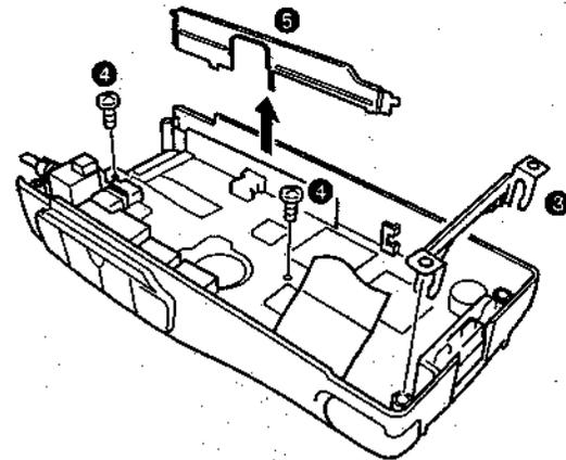
3. Push the cross key section (●) on the key top upward from the front with a finger. The control PC board is lifted and removed from the case.
