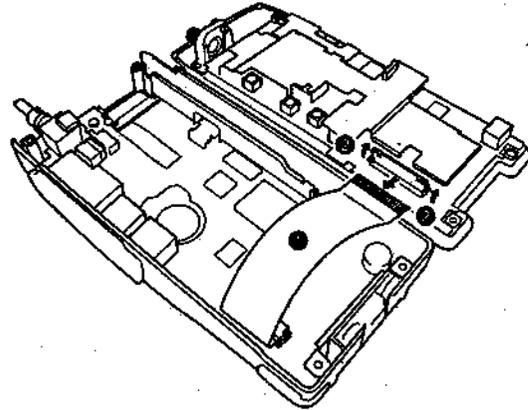
2. To remove the control PC board, remove the holder (●) and the two screws (●) holding the PC board. Then slide the fitting (●) on the back of the PTT switch to remove it.
