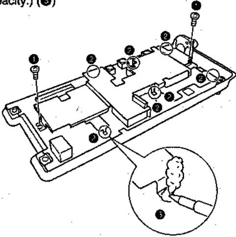
2. Remove the four screws (●) holding the power module and the four screws (●) holding the PC board. (The VHF power module and the shield case (●) are installed together.)
