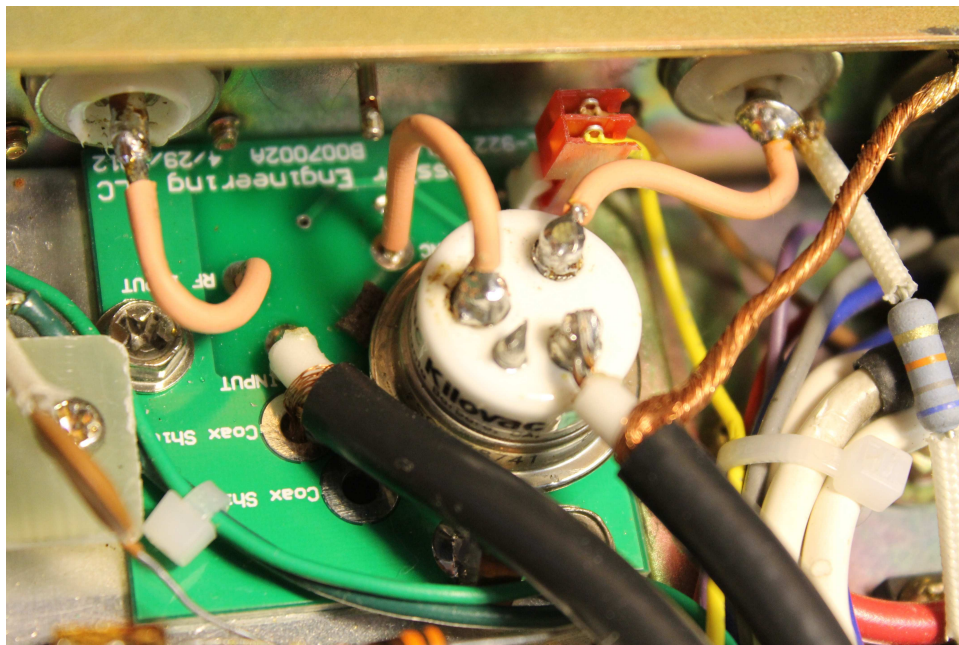
Figure 2.13: QSK T/R Relay PCB Installed
