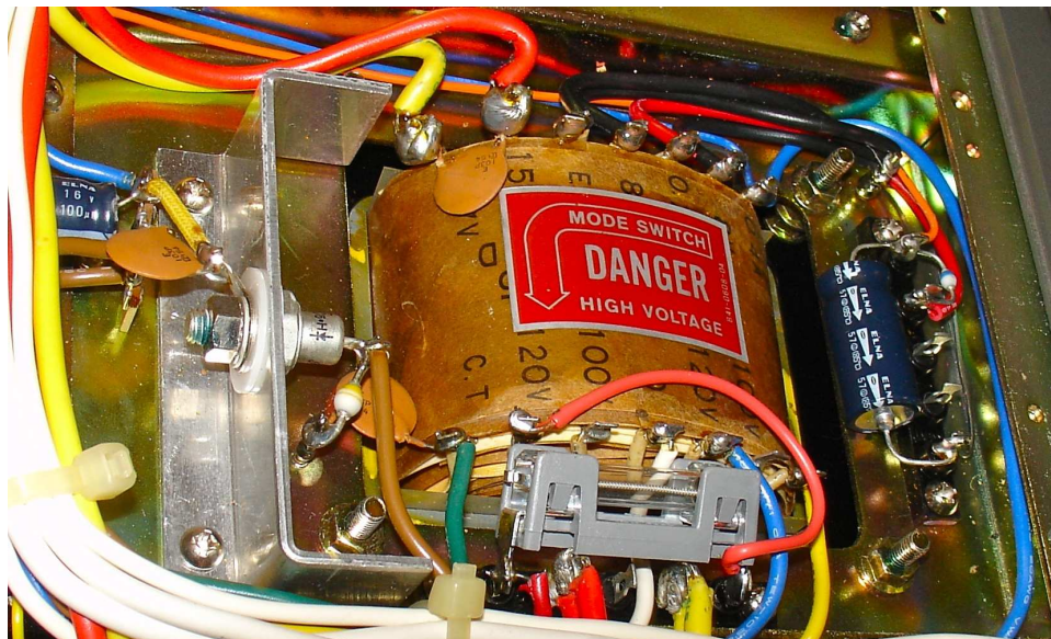
Figure 2.20: Zener Bias Diode Prior to Removal
