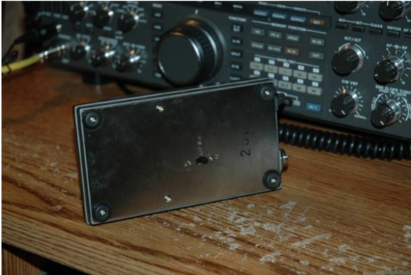
Bottom View- Shows Pre_amp “In/Out” switch
